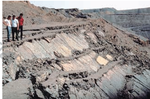
Photo B Slope failures in open cast mines, southern Spain.
