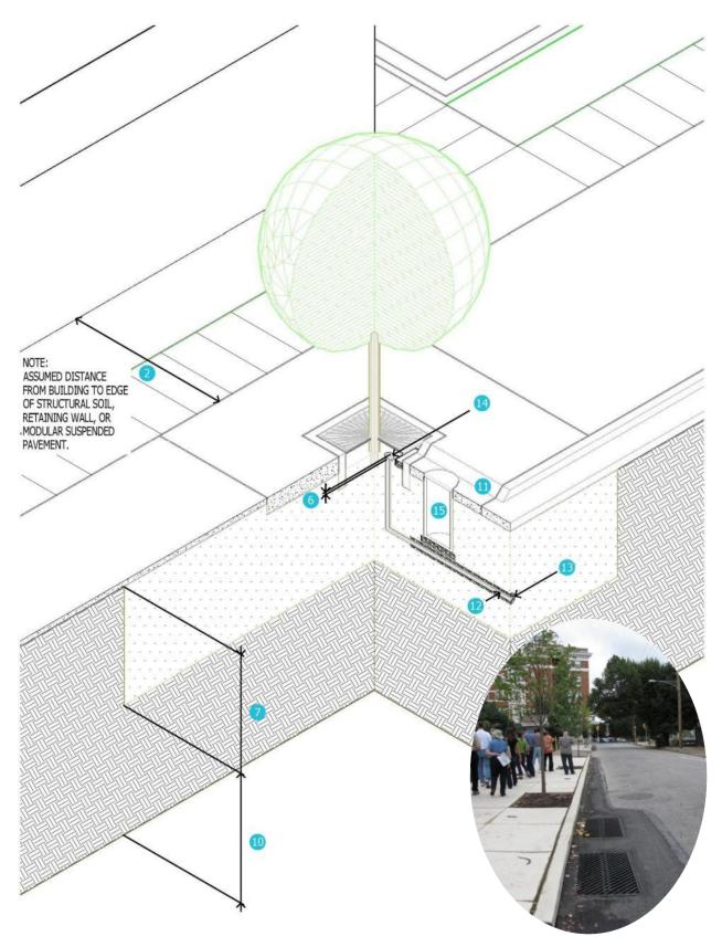
FIGURE 5-8 TREE BOX DIAGRAM
