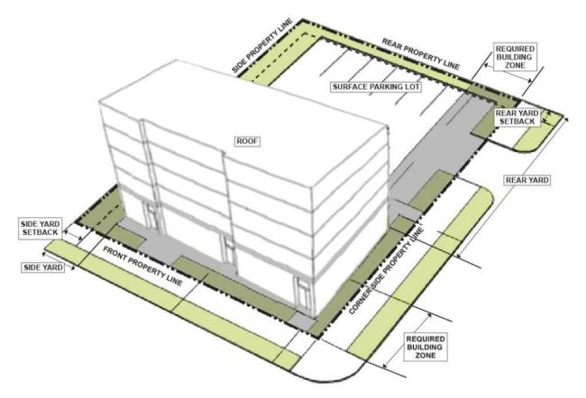
FIGURE 6-3 POTENTIAL ELEMENTS OF A BUILDING SITE
