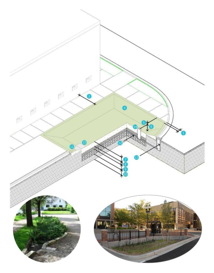
FIGURE 5-9 BIORETENTION CURB EXTENSION DIAGRAM
