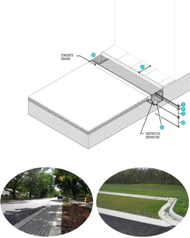
FIGURE 5-10 PERMEABLE PAVEMENT DIAGRAM
