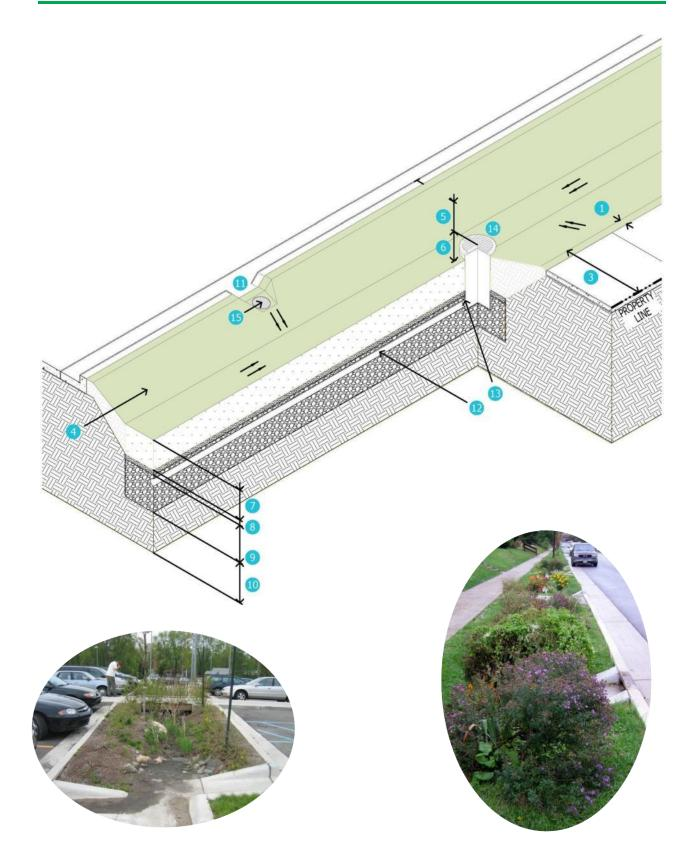
FIGURE 5-6 BIORETENTION SWALE DIAGRAM
