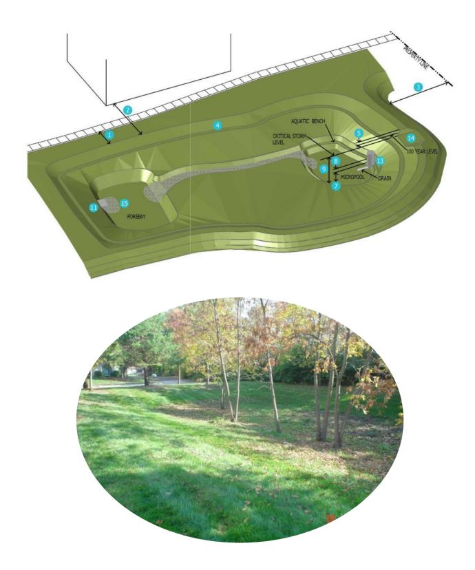
FIGURE 5-15 EXTENDED DRY DETENTION DIAGRAM
