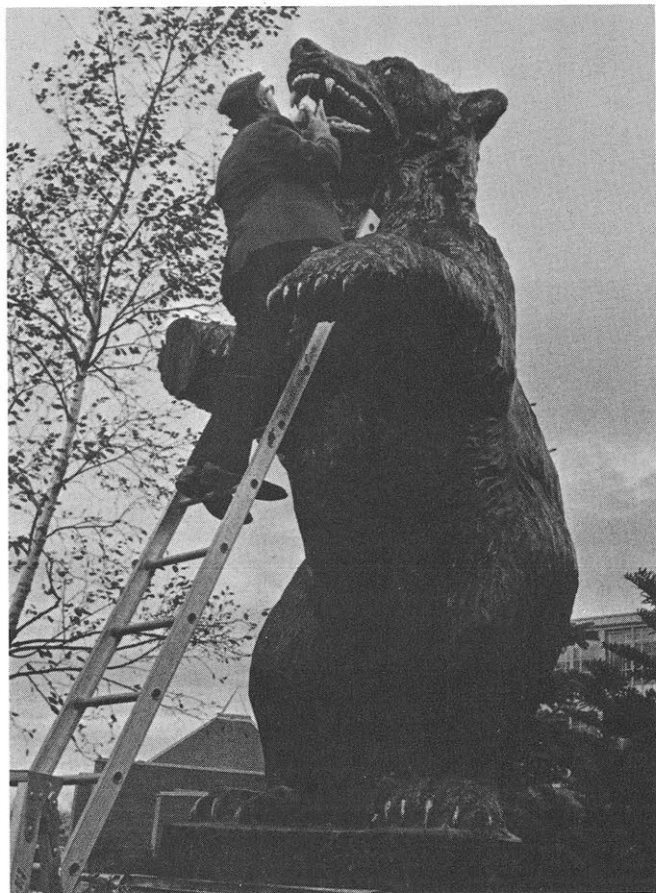
Figure 32 —The Shigometer detects decay in many types of wood products. F533448
