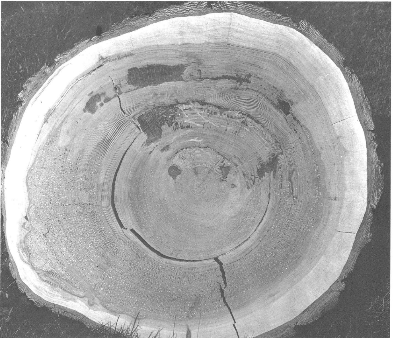
Figure 17— Fomes pini in Douglas-fir. F533424
