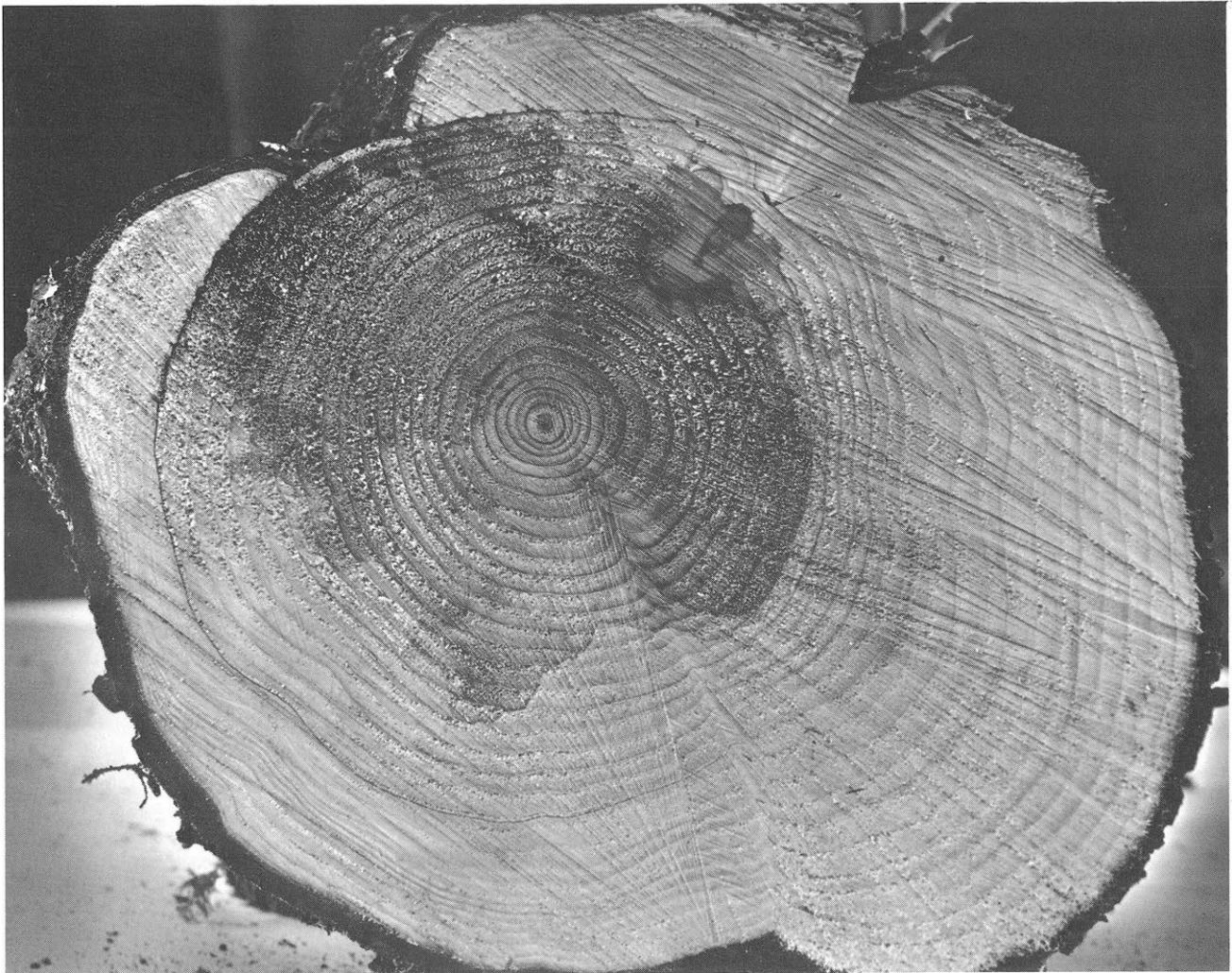
Figure 13 —Discolored and decayed wood in western hemlock. F533421
