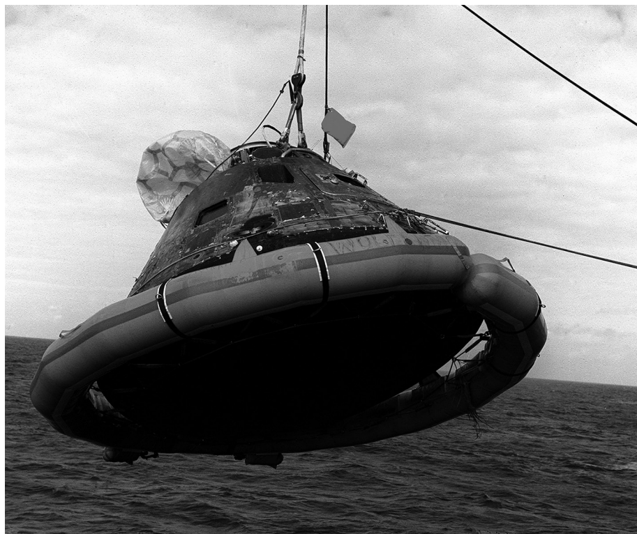
Figure 4.4 Apollo 11 Command Module and its flotation collar hoisted aboard the USS Hornet . Astronauts have already exited from the craft.
