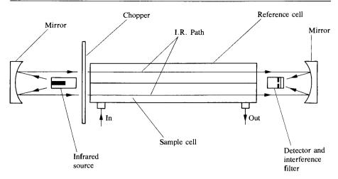
Fig. 19.5 Diagram of the infrared analyser unit of the Lion Intoximeter 3000 breath alcohol analyser. Reproduced by permission of Lion Laboratories Ltd, Ty Verlon Industrial Estate, Barry, Wales CF6 3BE, UK.
