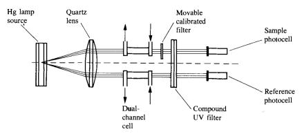
Fig. 8.5 Block diagram of a double-beam UV detector.
