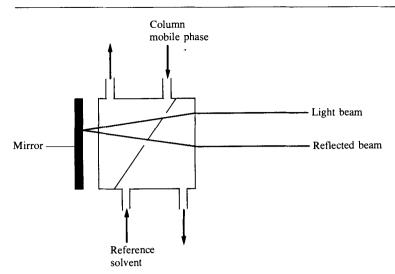
Fig. 8.4 Refractive index detector.
