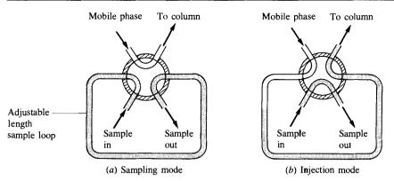
Fig. 8.3 Operation of a sample loop.
