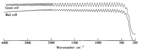
Fig. 19.7 Interference patterns from empty fixed-path-length cell. Reproduced by permission from R. C. J. Osland, *Principles and Practices of Infrared Spectroscopy*, 2nd edn, Philips Ltd, 1985.
