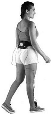
Figure 1.8 Stride Analyzer footswitch-based portable gait analysis system (B & L Engineering, Tustin, CA)
