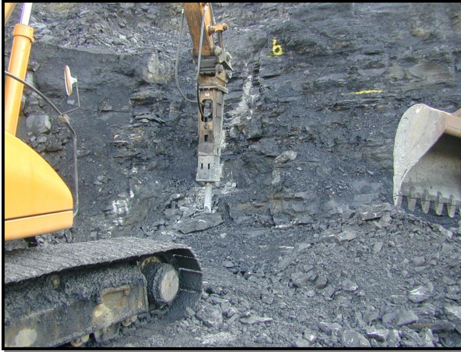
Plate 5 – Rock pecker on secondary breakage duties
