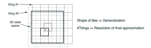
Figure 9.5: Multiple, overlapping gridtilings.
