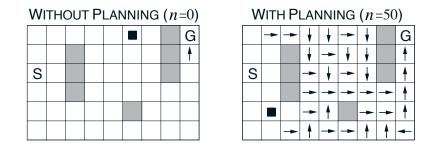
Figure 8.6: Policies found by planning and nonplanning Dyna-Q agents halfway through the second episode. The arrows indicate the greedy action in each state; no arrow is shown for a state if all of its action values are equal. The black square indicates the location of the agent.
