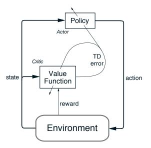
Figure 11.1: The actor-critic architecture.
