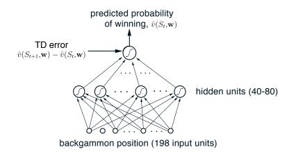
Figure 14.2: The neural network used in TD-Gammon
