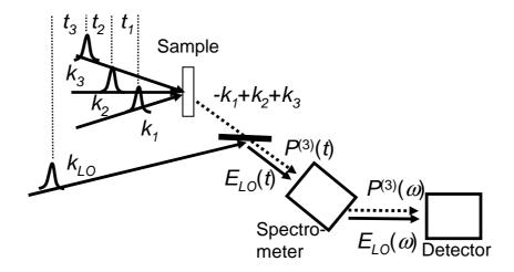
The action of this spectrometer is to perform the Fourier-transform with respect to  $t_3$ . Scanning of  $t_3$  is no longer needed. When using an array detector that covers the whole  $\omega_3$ -frequency range of interest in one shot, this actually reduces the measurement time significantly since only one time axis  $t_1$  needs to be scanned.
