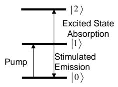
where both the  $0\rightarrow 1$  and the  $1\rightarrow 2$  transition are near-resonant with the probe pulse (however, they don't necessarily have exactly the same frequency). In a pump-probe experiment, we use the following geometry:
