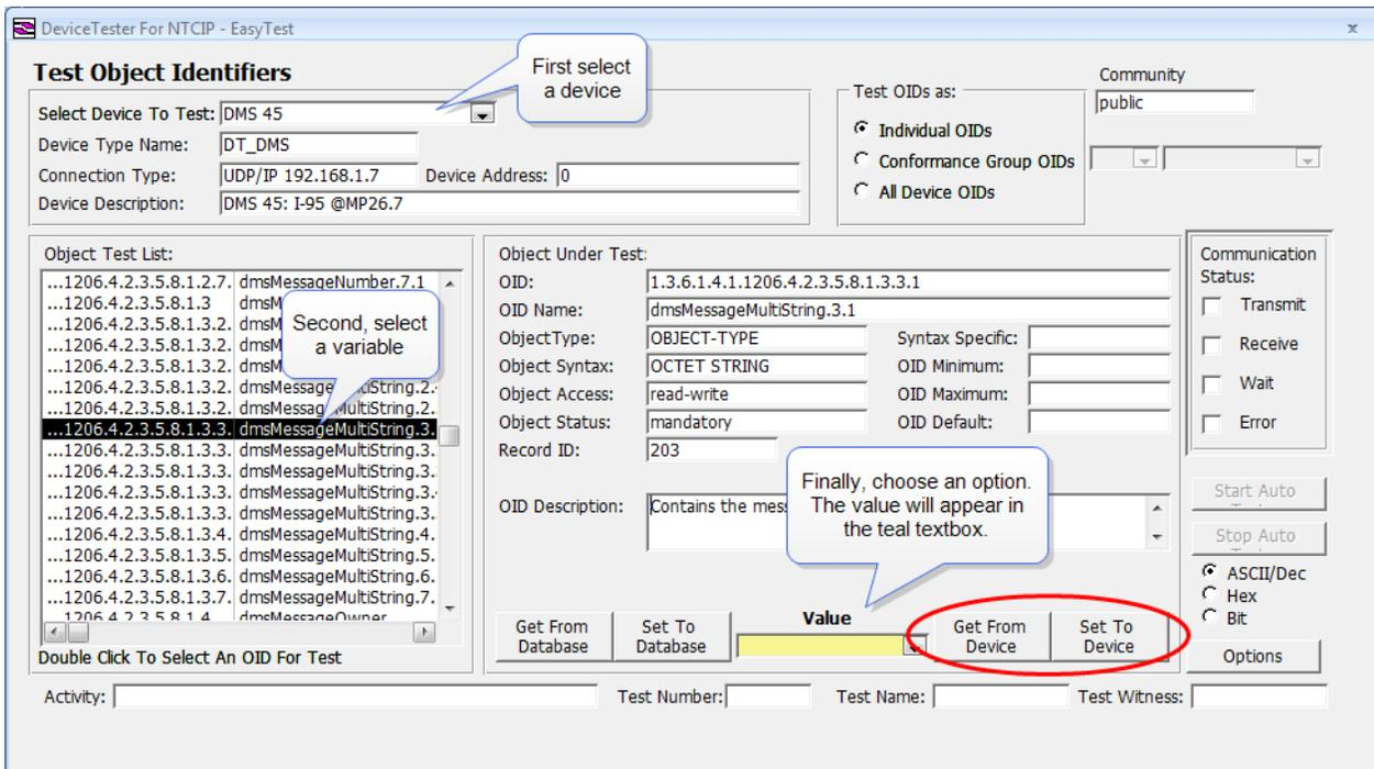
To Set (write a value to) an object, enter the value in the Value box, then click on the Set to Device box.
