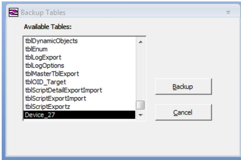
2. Choose the device required in the list by highlighting it. Press Backup. A dialog window will appear, asking where to save the .MDB file. Once the file is saved, it can be transferred to another system.
