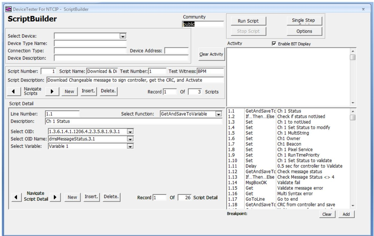
3. First, select the device you wish the script to run on using the Select Device drop down. The information at the top of the form will automatically fill in.
