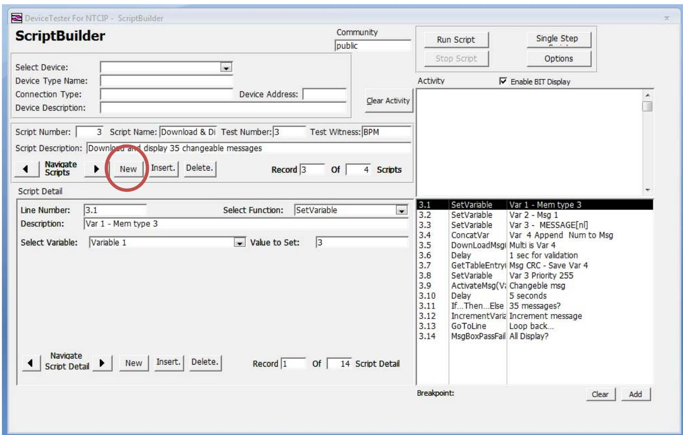
2. The script number will be automatically generated, but the description should be entered at this point. A test number (optional field that is a reference number) and a test witness (optional field for tests witnessed by a third party) can be entered as well.
