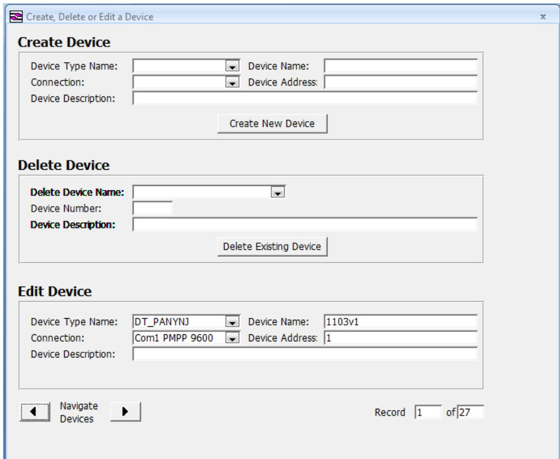
9. Use the top of the form to create the new device. Use the drop down menu to select a Device Type, and use the Connection drop down to select the
