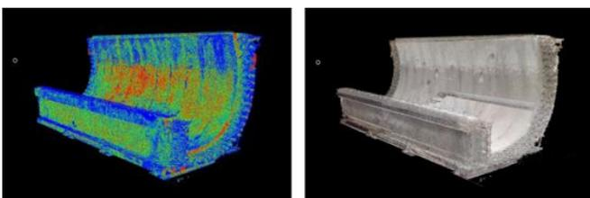
**Figure 8** – Complete point cloud and image in 3D.
