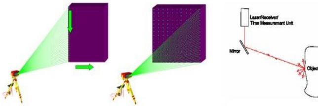
**Figure 2 - LiDAR scanning process** (Source: Leica-geosystems).
