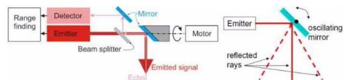
Figure 1 - LiDAR's principles [10].
