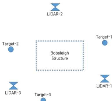
**Figure 6** – Layout of the scan and target control point around bobsleigh structure.
