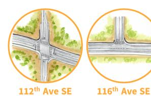
Signalized intersection has potential for highspeed crashes and minor-leg stop control can lead to risky behaviors in congested conditions
