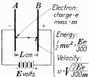
FIG. 68.—Acceleration of an electron in a uniform electric field. The expression for velocity neglects the change of mass which occurs at high velocities [cf. Eq. (51)].
