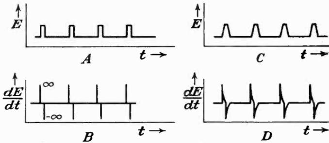
FIG. 219.—Differentiation of sync pulses. Ideal rectangular pulses (A) when differentiated produce sharp pulses of infinite amplitude (B), whereas nonideal trapezoidal pulses (C) produce pulses of finite height followed by sloping discharges (D).
