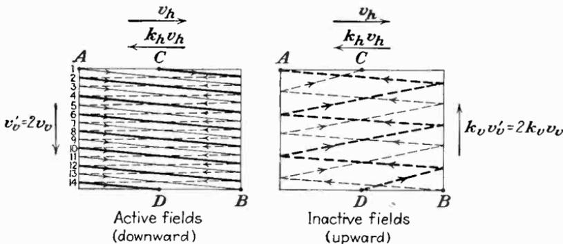
FIG. 20.—The odd-line method of interlaced scanning, now standard in the United States. The upward and downward scanning motions are of equal length (*cf.* Fig. 19) and the number of lines in each field is a whole number plus one-half ( $262\frac{1}{2}$  lines for a 525-line pattern).
