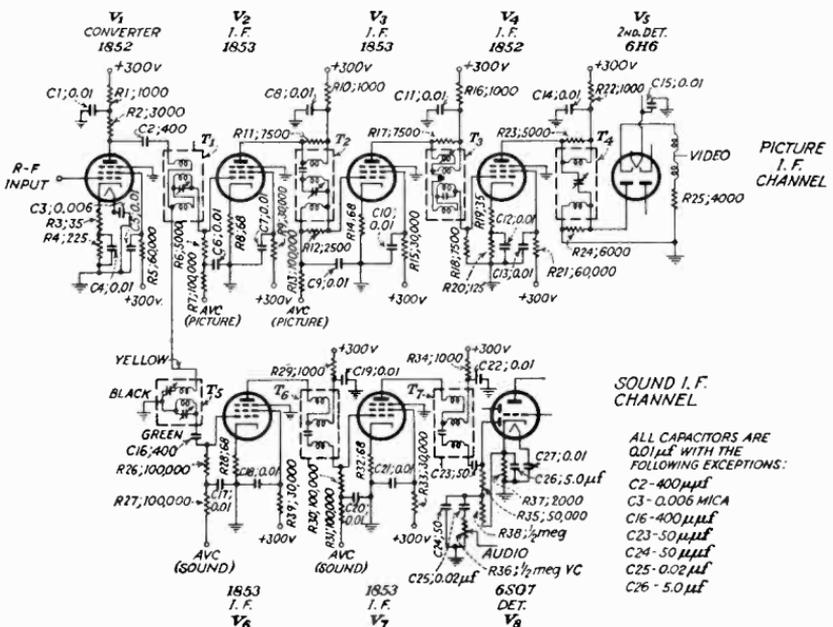
FIG. 299.—Typical i-f system (picture and sound) using commercially available i-f coupling units.
