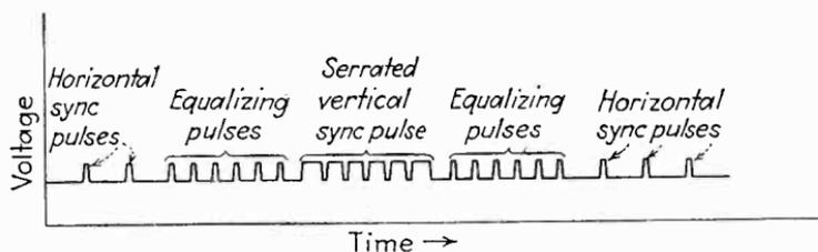
FIG. 93.—The serrated type of vertical sync pulse (with equalizing pulses). In this system, the energy contained in the serrated pulse is integrated to distinguish it from the smaller energy present in the horizontal pulses. The equalizing pulses produce equal energy integrations during successive blanking periods between the interlaced fields.
