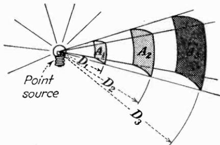
FIG. 28.—Light flux radiating from a point source. As the illuminated areas  $A_1$ ,  $A_2$ , and  $A_3$  are removed from the source, the light flux available in the given solid angle is spread over larger and larger areas, with resulting decrease in illumination.
