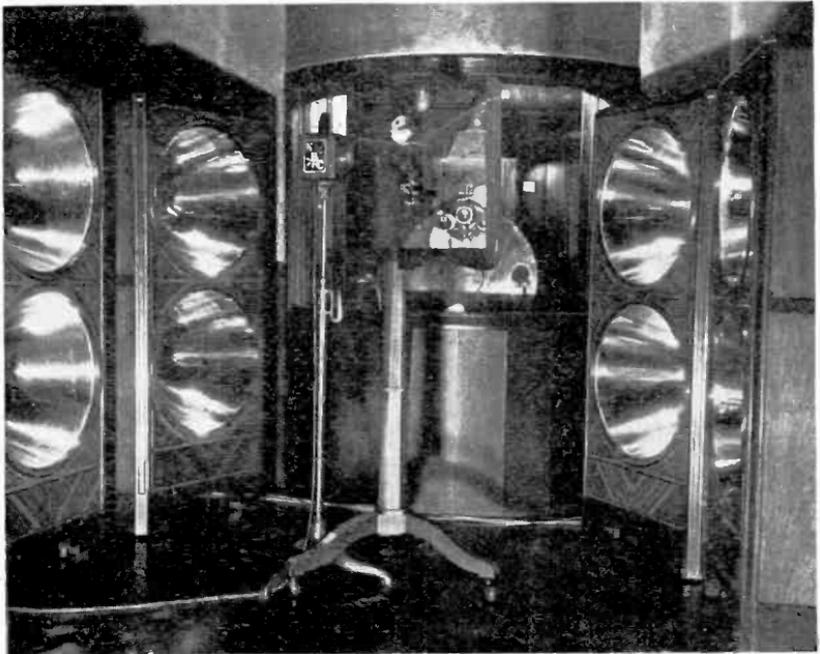
FIG. 46B.—Early NBC television pickup equipment, which made use of the flying-spot method of mechanical scanning. Eight phototubes and reflectors were used to gather the light reflected from the object being televised. The scanning disk and lens system are visible in the booth at the rear.
