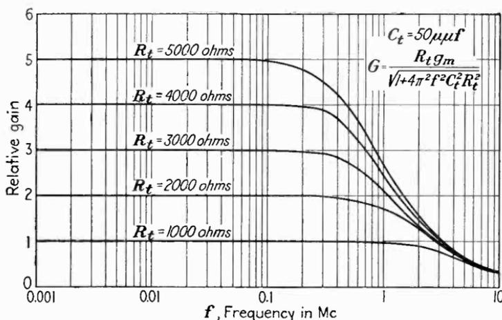
FIG. 121.—Effect on high-frequency response (uncompensated amplifier) of increasing the shunt resistance  $R_t$ . While higher gain may be obtained thereby at low frequencies, the presence of the shunt capacitance places an upper limit on the gain at high frequencies.
