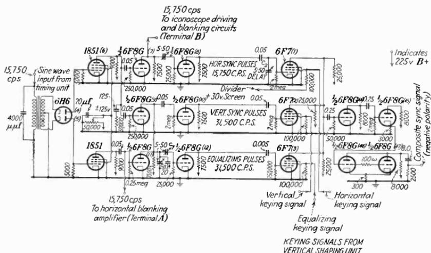
FIG. 254.—Horizontal shaping units of the sync signal generator. This unit accepts 15,750-c.p.s. timing pulses from the timing unit (Fig. 251), and 60-c.p.s. keying signals from the vertical shaping unit (Fig. 255), and derives from them the composite sync signal with horizontal, equalizing, and serated-vertical pulses. It produces also 15,750-c.p.s. blanking signals for the iconoscope and picture tube.
