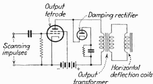
FIG. 87.—Typical output circuit of magnetic deflecting system, with damping rectifier and absorption circuit to remove oscillations shown in Fig. 86.
