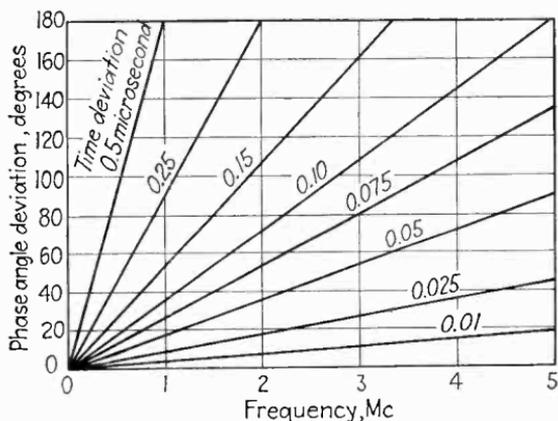
FIG. 103.—Relationship between angular phase measure and the equivalent time delay. The phase angle corresponding to a given fixed time delay becomes larger as the frequency increases.
