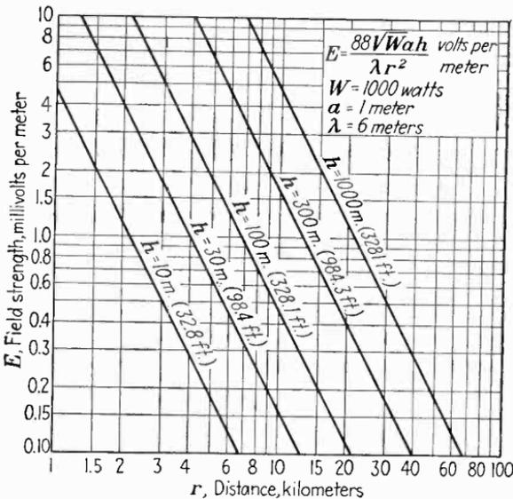
FIG. 152.—Signal field strength against distance and transmitting antenna height, for given values of power, receiving antenna height and operating wavelength, computed by Eq. (207).
