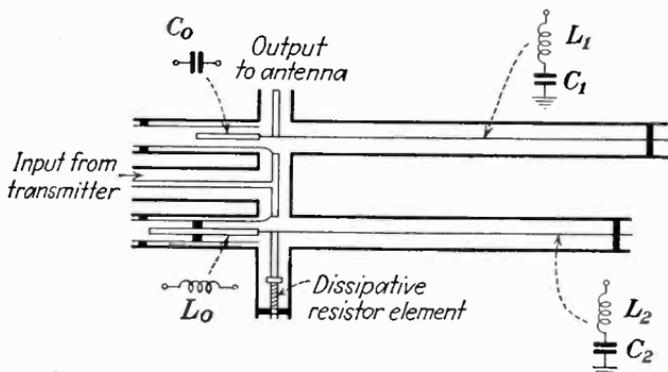
FIG. 266A.—Structure of coaxial vestigial sideband filter used at station W2XBS. The lumped constants shown refer to the corresponding symbols in Fig. 163. (After G. H. Brown.)
