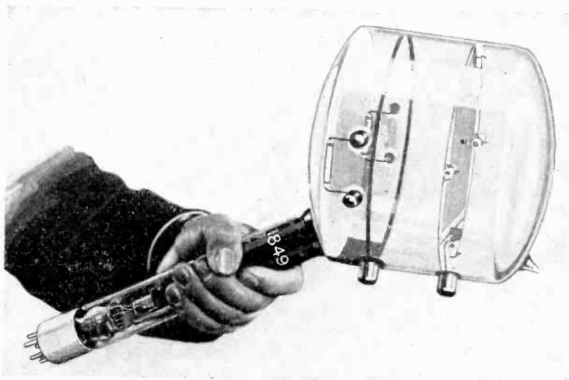
FIG. 8.—A typical television camera tube, the type 1849 iconoscope, now widely used in television broadcasting.
