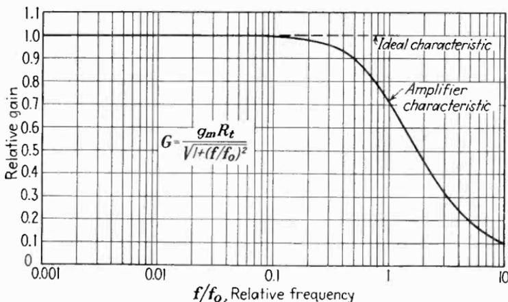
FIG. 118.—High-frequency amplitude-response characteristic of the uncompensated amplifier (Fig. 117) plotted in terms of the reference frequency  $f_0$  determined by the values of shunt resistance and capacitance in the coupling circuit.
