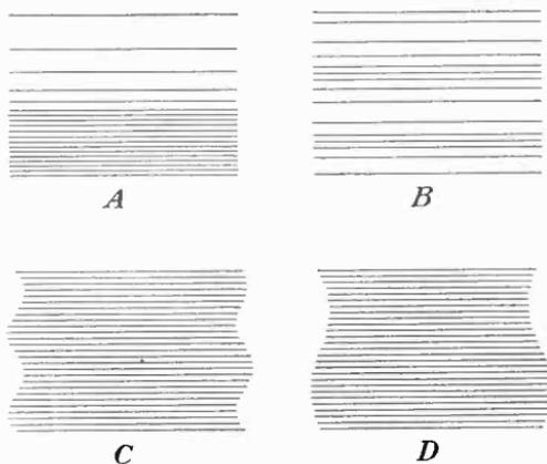
FIG. 23.—Scanning defects characteristic of the pattern as a whole. *A* and *B* result from nonlinear vertical scanning, *C* from linear displacement, and *D* from variations in the horizontal scanning amplitude.
