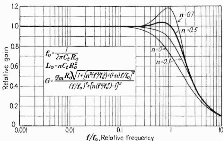
FIG. 126.—Amplitude-frequency response characteristics of the shunt-peaking compensated amplifier, for different values of the compensating inductance  $L_o$ . The case for  $n = 0$  is the uncompensated case, whereas that for  $n = 0.5$  is that usually adopted in practice. Plotted as the magnitude of Eq. (147).
