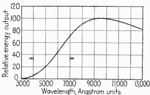
FIG. 34.—Spectral distribution of a standard tungsten incandescent lamp operated at 2870°K. The arrows mark the approximate limits of the visible region of the spectrum (violet, 4000 Angstroms, to red, 7000 Angstroms).
