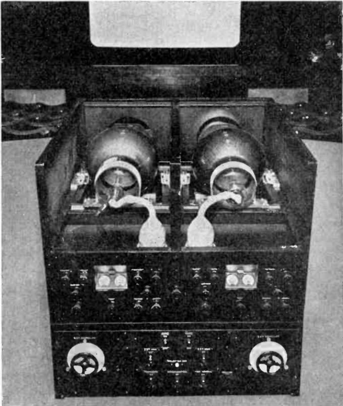
FIG. 309.—British type of projection picture-tube equipment. An accelerating voltage of 50,000 volts is used to obtain pictures about 9 by 12 feet in size.
