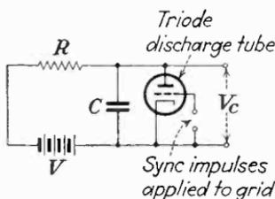
FIG. 80.—Saw-tooth generating circuit widely used in television practice. A three-element discharge tube (gas-filled thyratron or vacuum triode) discharges the capacitor when a sync pulse is applied to its grid.
