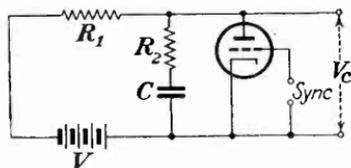
FIG. 82.—Peaking circuit used to produce the voltage waveform of Fig. 81C. The combination of  $R_2$  and  $C$  acts to produce a voltage wave, part impulse, part saw-tooth, necessary to produce a saw-tooth of current in an inductive-resistive circuit.
