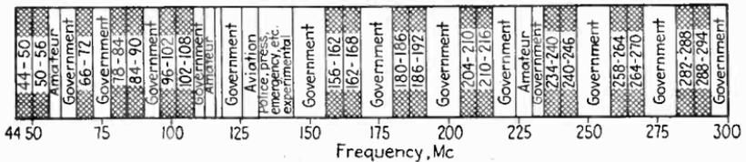
FIG. 146.—Principal features of frequency allocations made by the Federal Communications Commission in 1937, for frequencies from 44 to 300 Mc. A recent F.C.C. revision (June, 1940) has allocated the 44-50 Mc. channel to frequency modulation and the 60-66 Mc. channel to television.
