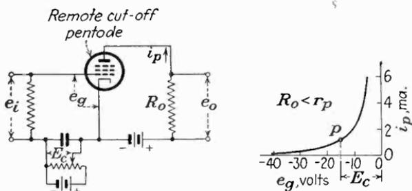
FIG. 137.—Typical distorting amplifier circuit used for obtained nonlinear reproduction ("gamma-control" amplifier). By adjusting the bias voltage  $E_c$  different portions of the  $i_p$ - $e_o$  operating characteristic may be chosen.
