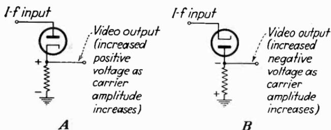
FIG. 192.—Video detector polarities: *A*, the cathode-above-ground connection which produces a positively poled output (output signal more positive as carrier amplitude increases). The anode is returned to ground through the i-f circuit; *B*, the anode above ground (cathode grounded through i-f) which produces a negatively poled output.
