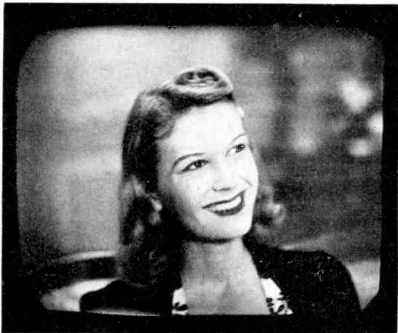
FIG. 56.—Appearance of television image when subject is adequately illuminated and when shading-correction signal has been added to remove effects of spurious shading signal. (Figs. 54, 55, and 56 from Lohr, "Television Broadcasting.")
