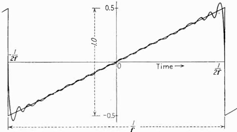
FIG. 108.—The ideal saw-tooth wave, represented by Eq. (81). The wavy line shows the approximation to the original wave obtained when twenty harmonics are included in the sum of the series.
