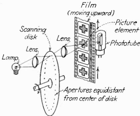
FIG. 45.—Light-source scanning of motion-picture film. In this arrangement, all the light is directed to each successive picture element, and subsequently collected by the phototube. When a multiplier phototube is used this method is capable of high-definition transmission with adequate signal-to-mask ratio.
