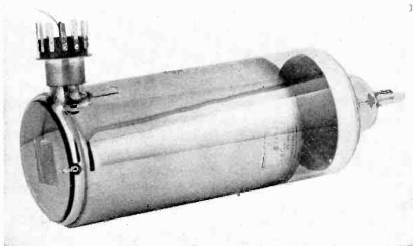
FIG. 48B.—Physical appearance of a modern image dissector, designed especially for the transmission of motion-picture film images. The terminals at the top lead to the electrodes in the electron-multiplier structure.
