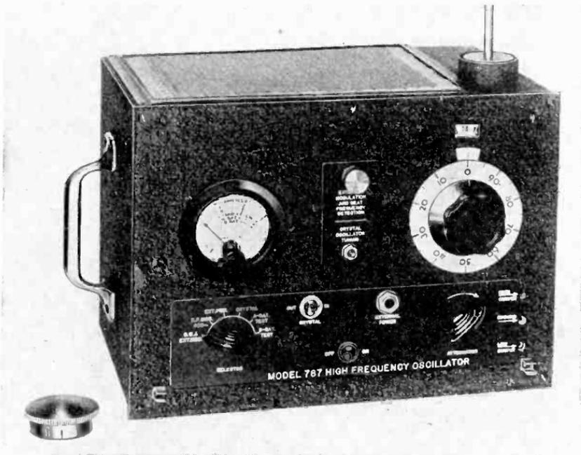
FIG. 306A.—External appearance of u-h-f signal generator, suitable use in method shown in Fig. 305.
