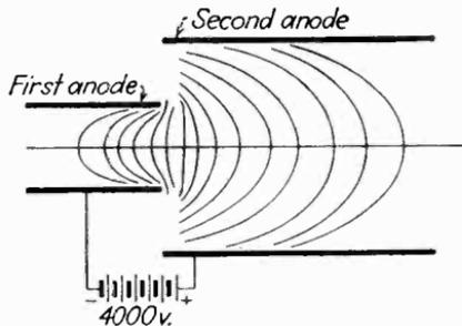
FIG. 63.—Equipotential contours of the second electron lens of the gun shown in Fig. 61. Any electrode system having cylindrical symmetry about the gun axis can serve as a lens, but the particular form shown has gained the widest acceptance in commercial tubes.
