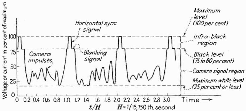
FIG. 98.—Three lines and blanking periods of the N.T.S.C. Standard Video Signal.
