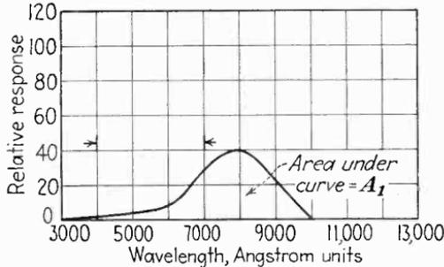
FIG. 36.—Response of the photoelectric surface of Fig. 35 to the spectral distribution of Fig. 34, that is, the product of the two curves. Note that the response in the visible region (between the arrows) is very low, compared with that in the infra-red region above 7000 Angstroms.
