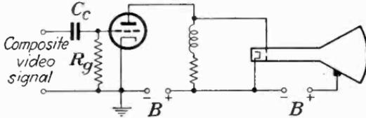
FIG. 213.—Simple d-c reinsertion circuit operating on the grid-current characteristic of the video amplifier, which operates without cathode bias. The circuit has two inherent drawbacks: the video tube draws heavy plate current in the absence of signal, and the control grid of the picture tube assumes cathode potential if the plate current of the video amplifier fails.
