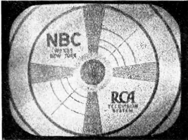
FIG. 234.—Interference caused by tube and circuit masking voltages (thermal agitation and shot-effect noise) usually associated with a weak signal and most clearly visible in the absence of other interferences.
