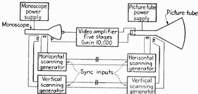
FIG. 302.—Basic connections of simple image-signal generator, which operates without generation of standard sync signals and hence does not produce an interlaced pattern, but which serves for many test purposes.
