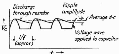
FIG. 210.—Ripple percentage based on height of discharge curve.
