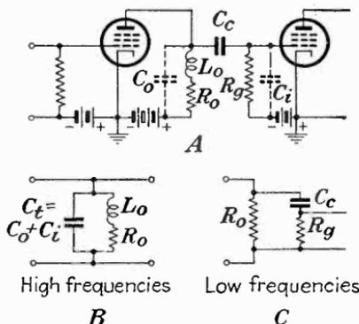
FIG. 125.—The “shunt-peaking” system of compensating high-frequency response by the insertion of the coil  $L_o$  in shunt across the amplifier output (and in series with the load resistor). *B* and *C* give the equivalent circuit at high and low frequencies.
