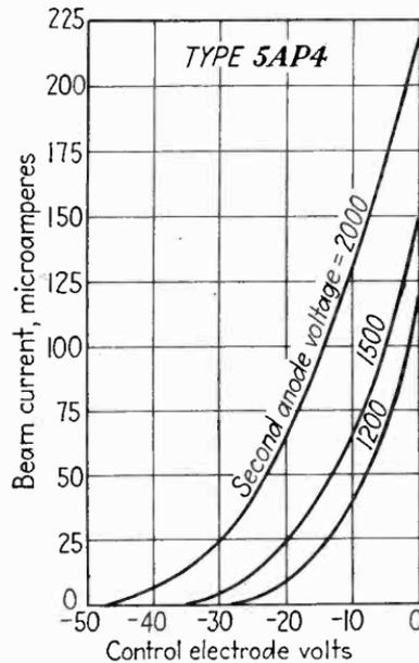
FIG. 65.—Typical control characteristic of an electrostatic gun. Note that the relationship between control voltage and beam current is not linear, particularly so in the operating region from  $-15$  to  $-40$  volts.
