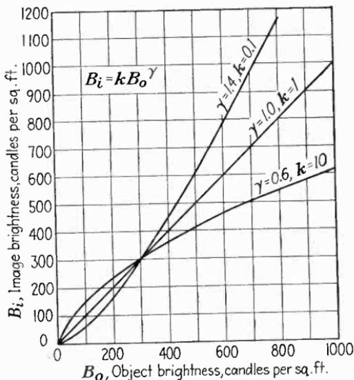
FIG. 114.—Relationships between object brightness (in studio) and image brightness (at receiver) which satisfy the condition that the sensation in the minds of the receiver audience shall be proportional to the sensation in the minds of the studio audience. Based on the Weber-Fechner law which states that sensation is proportional to the logarithm of brightness (cf. Figs. 194 to 198).
