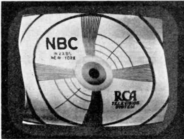
FIG. 231.—Hum (60-c.p.s.) in the horizontal deflection circuit or horizontal synchronizing circuit, or both.
