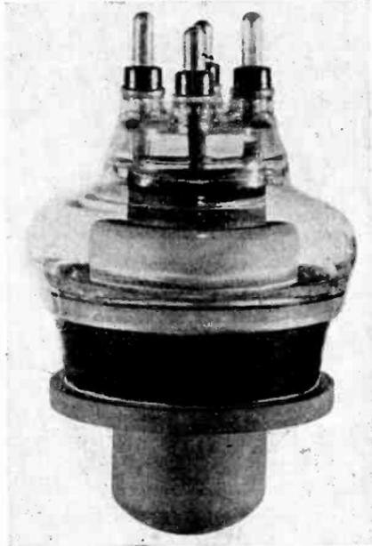
FIG. 260A.—Type GL-880 triode tube with re-entrant anode which allows adequate cooling without excessive electrode length. Used in amplifiers in the General Station at Albany (Fig. 272).
