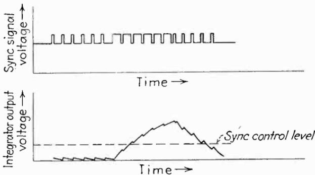
FIG. 223.—Integration of serrated vertical sync pulse and equalizing pulses. The instant of synchronization occurs when the integrated pulse passes through the sync control level. Very slight changes in waveform cause irregular synchronization, hence the need for equalizing pulses (*cf.* Fig. 97).
