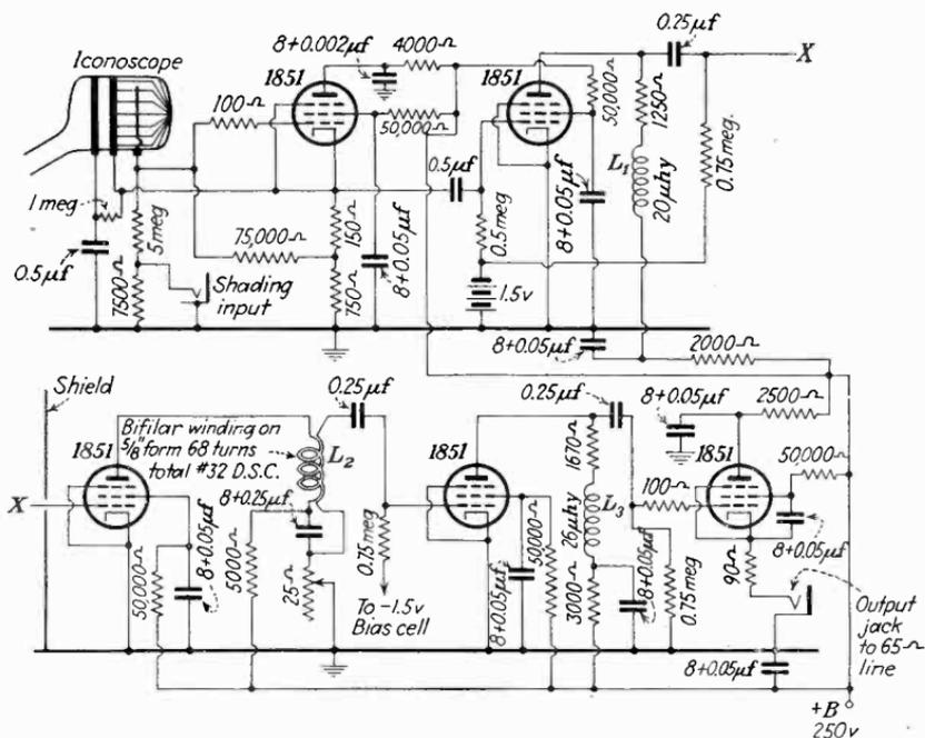
FIG. 242.—Complete diagram of iconoscope preamplifier.
