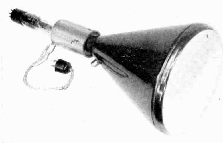
FIG. 85.—Typical magnetically-deflected picture tube. The scanning yoke (cylindrical structure) contains two sets of coils which produce horizontal and vertical deflecting fields at right angles to the axis of the tube.
