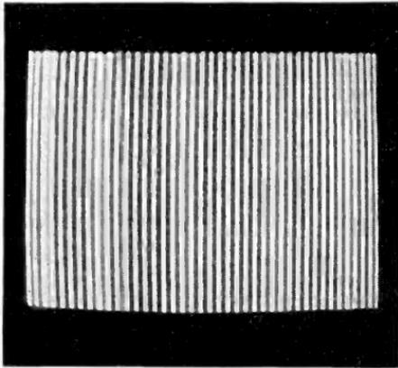
FIG. 293—Line pattern obtained with 660,000 c.p.s. signal applied to control grid and horizontal sync circuits. Note the wide bands in the background, formed during the horizontal retrace. The value of  $k_A$  indicated is about 10 times.
