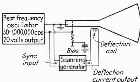
FIG. 290.—Nonimage method of testing linearity and amplitude of scanning motions.
