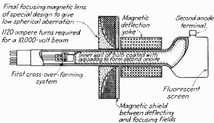
FIG. 308.—Internal arrangement of projection picture-tube system shown in Fig. 307.
