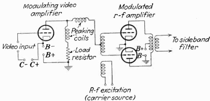
FIG. 159.—Method of conductive coupling between modulating video amplifier and modulated r-f amplifier. The plate of the video amplifier operates at the bias potential of the r-f amplifier, hence the cathode of the video amplifier must be maintained at a high negative potential.
