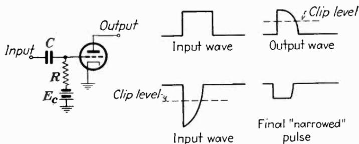
FIG. 253A.—The narrowing function in wave-shaping circuits. The initial square wave is passed through the differentiating circuit ( $RC$  circuit, left) and clipped (upper right). Then the portion above the clip level is amplified and clipped again. The final pulse is thus narrowed but not delayed.
