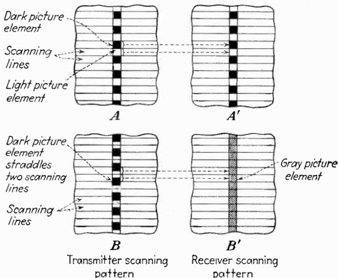
FIG. 12.—Relationship of scanning lines to picture elements. If the scanning lines pass directly over the picture elements, the reproduction  $A'$  is like the original  $A$ . If, however, the scanning lines "straddle" the picture elements, the detail may be wholly lost in the reproduction (cf.  $B'$  with  $B$ ).
