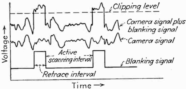
FIG. 245.—Combination of blanking signal (bottom) and camera signal (middle) to form a semicomposite signal which can be clipped at the blanking level.
