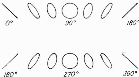
Fig. 187.—Lissajous figures formed on cathode-ray oscilloscope screen for various phase displacements between voltages of equal amplitude and frequency.
