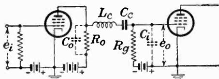
FIG. 128.—The “series-peaking” method of high-frequency compensation, which results in higher gain and more linear phase response than the shunt-peaking method. The series coil  $L_c$  isolates the two capacitances  $C_o$  and  $C_i$ .
