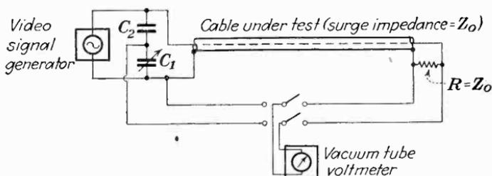
FIG. 145.—Measurement of attenuation in coaxial cable.
