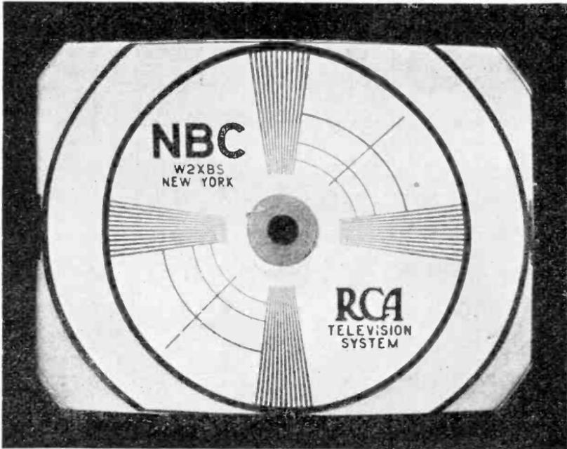
FIG. 25B.—Televised reproduction of the chart in Fig. 25A, photographed from the monitor picture tube in the NBC studios. The resolution of the wedges is substantially complete, representing "350-line" performance. Note, however, the indefiniteness of the inner portions of the horizontal wedges, indicating that 400 active scanning lines are just barely able to reproduce 350 picture elements in the vertical direction.
