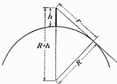
FIG. 149.—Geometrical relationship of antenna height to the horizon distance.
