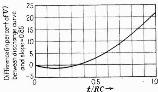
Fig. 77.—Difference between charge-time curve and linear slope ( $= 0.85$ ). A nonlinearity of  $\pm 1$  per cent can be achieved if the charging time is restricted to  $0.4RC$  or less, but the nonlinearity increases to  $\pm 5$  per cent if the charge is allowed to continue for  $t = 0.7RC$  seconds.
