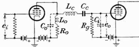
FIG. 130.—The shunt-series peaking system which combines the advantages of the shunt- and series-peaking coils.
