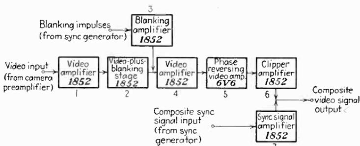
FIG. 243.—Block diagram of control amplifier (blanking and mixing amplifier) which produces the composite video signal from its camera, blanking, and synchronization components.
