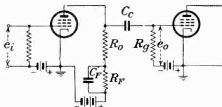
FIG. 131.—Compensation filter ( $R_F C_F$ ) applied to improve the amplitude and phase responses at low frequencies.
