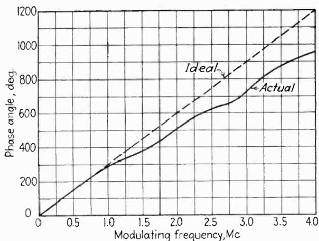
FIG. 188.—Typical phase response curve of an i-f amplifier. Note that the angle is measured in hundreds of degrees, representing the cumulative effects of several stages.
