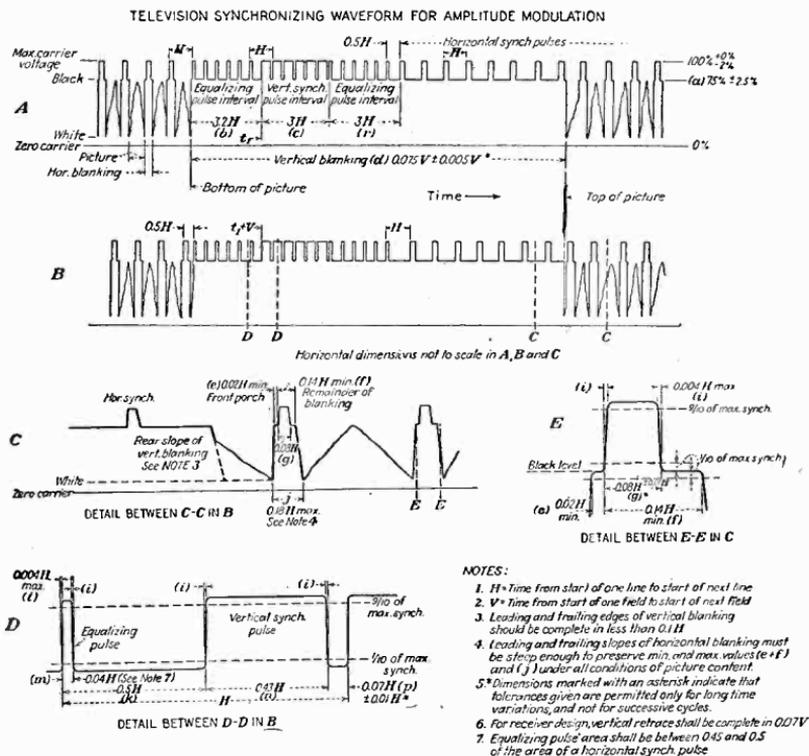
FIG. 312.—N.T.S.C. standard television signal.
