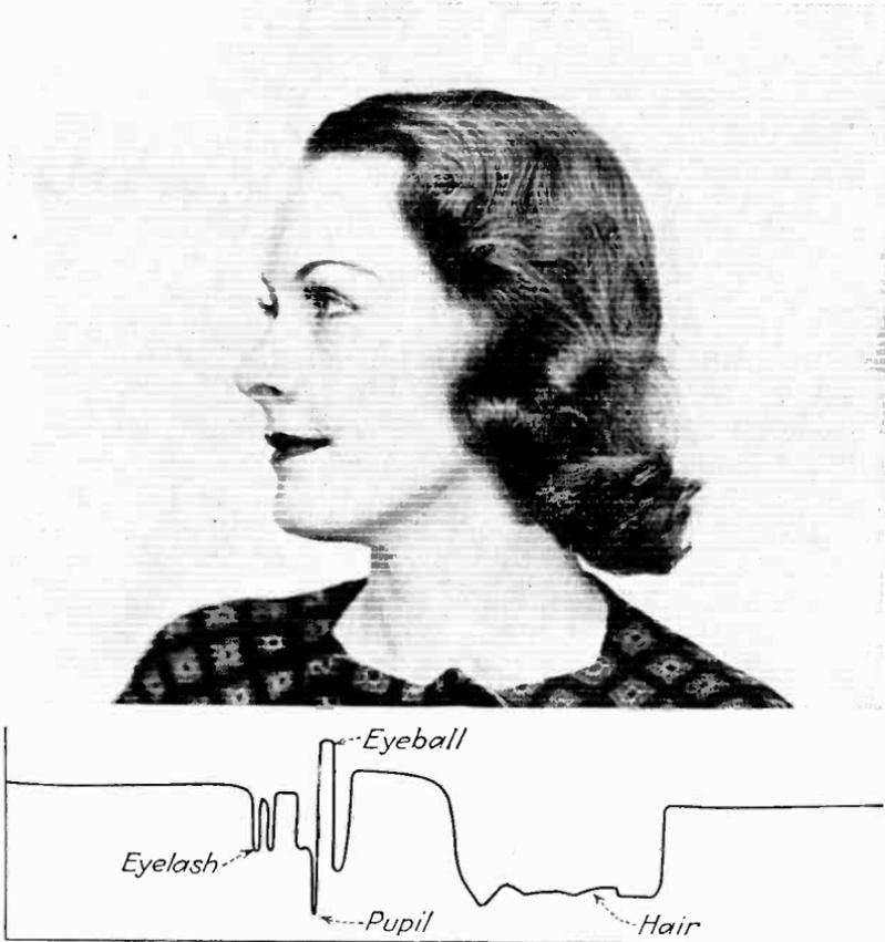
FIG. 6A.—The scanning technique. The image is divided into a number of parallel horizontal lines, each of which is explored in succession for the information it contains. The diagram shows the values of brightness (measured with a densitometer) at corresponding points along the line which passes directly through the pupil of the left eye. This "waveform" represents the information contained in that particular scanning line.
