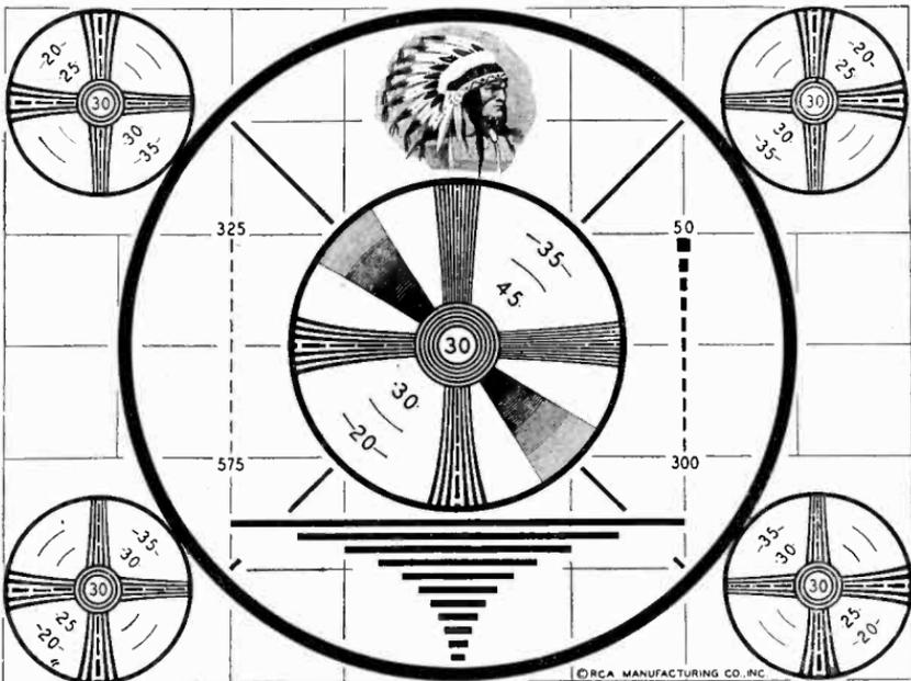
FIG. 301B.—Test chart printed on signal plate of type 1899 monoscope.
