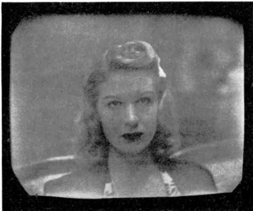
FIG. 55.—Appearance of televised image when subject is insufficiently illuminated.
