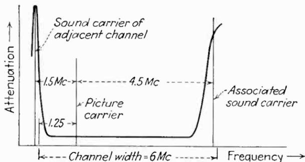
FIG. 162.—Attenuation characteristic required to transmit the vestigial sideband carrier signal according to the R.M.A. transmission standards.
