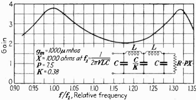
FIG. 182.—Response curve of the capacitively coupled band-pass circuit shown in the inset (after Seeley and Barden).
