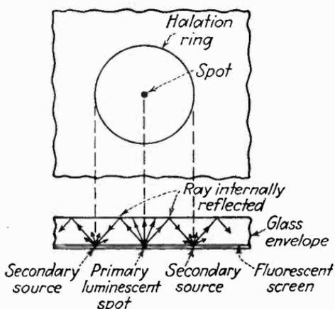
FIG. 206.—Halation due to total internal reflection in the glass face of the picture tube.
