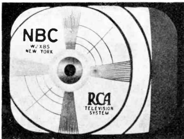
FIG. 238A.—Incorrect positioning due to excessive d-c component in horizontal scanning system.
