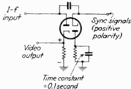
FIG. 193.—Double-diode circuit for video detection and amplitude separation of sync signals. The  $RC$  circuit in the right-hand section develops the cutoff bias.
