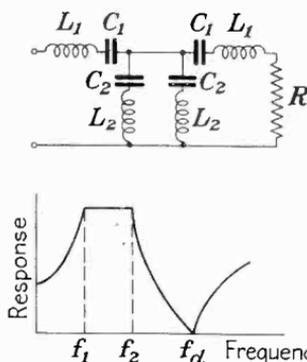
Fig. 179.—Elementary band-pass filter (*m*-derived) and idealized response characteristic.
