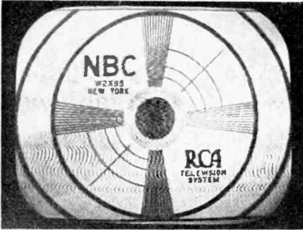
FIG. 232.—Stippled effect due to excessive interference from diathermy apparatus. The herringbone pattern results from frequency modulation of the diathermy interference.
