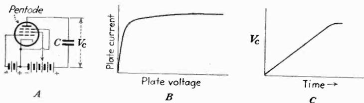
FIG. 78.—Current-limiting action of the pentode tube, useful for obtaining a linear charge-vs.-time relationship, but seldom used in television scanning circuits.
