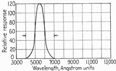
FIG. 37.—Standard visibility curve of the human eye. Compare with the response curve of the photoelectric surface, in Fig. 35.
