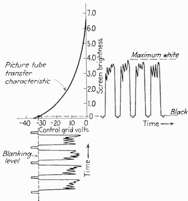
FIG. 212.—Signal-to-light relationship in a typical picture tube. The bias of the tube should be set so that the blanking level of the signal just coincides with the zero-light level of the output scale.
