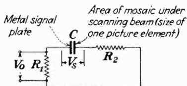
FIG. 57.—Equivalent signal circuit of iconoscope, on which the transient analysis is based.  $C$  is the capacitance between globules under a picture element and the signal plate.  $R_1$  is the coupling resistor and  $R_2$  is the ohmic resistance of the secondary emission path from mosaic to collector electrode.
