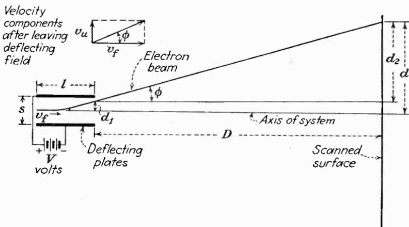
FIG. 69.—Electric deflection of an electron beam. The upward component of velocity, imparted while the electron is between the deflecting plates, persists for the remainder of the motion, producing the upward deflection  $d_2$ .
