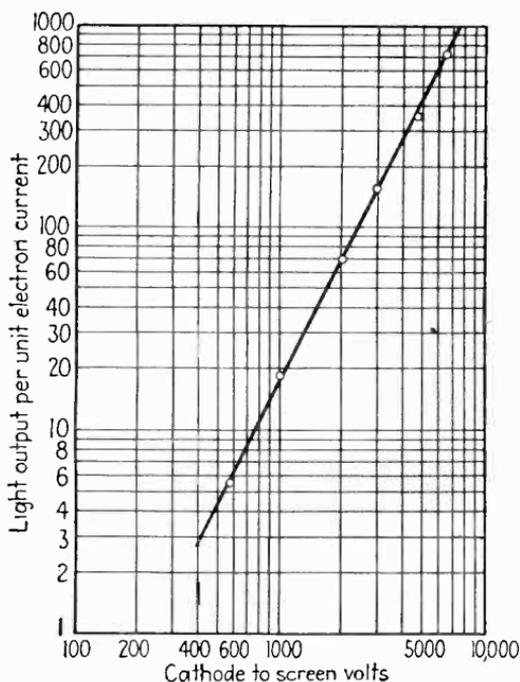
FIG. 202B.—Light output vs. screen potential, according to Nottingham's findings, which indicate the relationship in Eq. (251).
