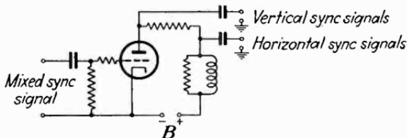
FIG. 224.—Combined waveform separator circuit in plate circuit of sync amplifier. The inductance differentiates the high-frequency pulses, while the resistor develops the low-frequency signals for integration.
