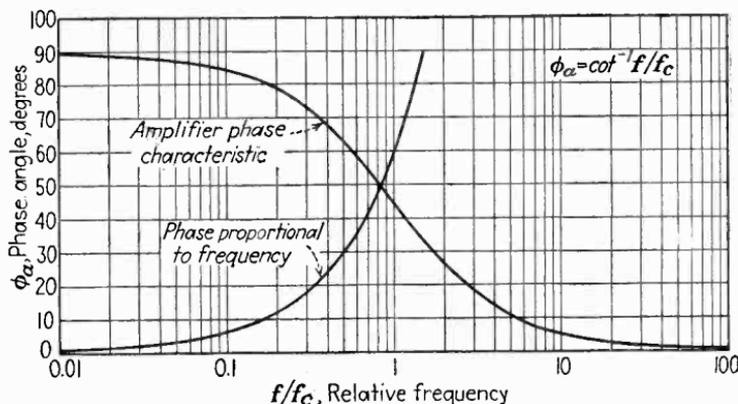
FIG. 124.—Phase-frequency characteristic of the uncompensated amplifier.
