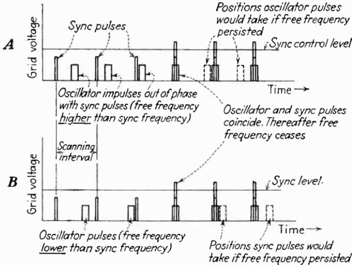
FIG. 91.—Two forms of synchronization between sync impulses and pulse generator impulses. In A the free generator frequency is higher than the sync frequency, and the sync impulses occur *during* the active scanning interval. Consequently the picture is divided in two by the blanking interval. This situation is avoided in B by making the free frequency lower than the sync frequency, so that the sync impulses and blanking occur at the end of the active scanning interval.
