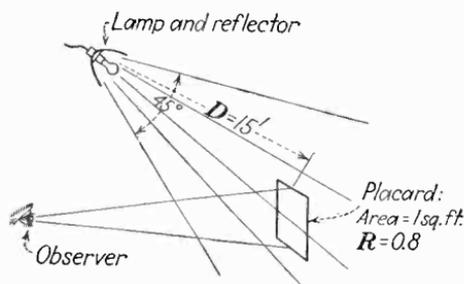
FIG. 30.—Illumination of a reflecting placard. The observed brightness depends on the distance  $D$  from the light source, and on the reflecting coefficient  $R$ , as well as on the geometry of the reflecting system.
