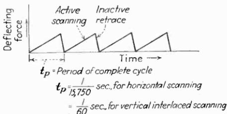
FIG. 73.—Saw-tooth waveform of deflecting force, required to produce a scanning pattern of uniform horizontal and vertical scanning velocities.
