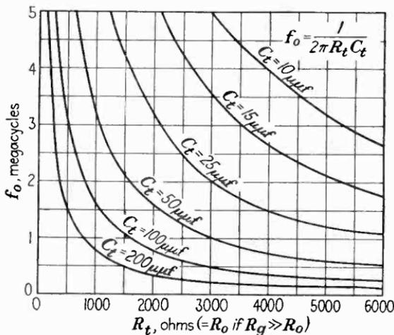
FIG. 119.—The reference frequency  $f_0$  in terms of the shunt capacitance  $C_t$  and resistance  $R_t$ .
