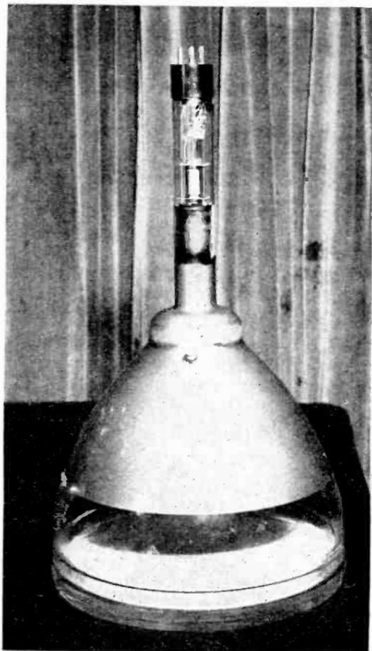
FIG. 200B.—Flat-faced picture tube, with glass face 0.6 in. thick to withstand external atmospheric pressure.
