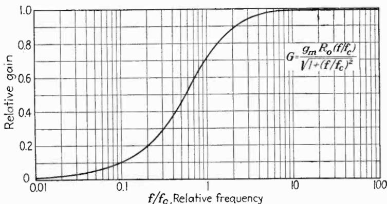
FIG. 123.—Amplitude-frequency response curve of uncompensated amplifier at low frequencies, in terms of the reference frequency  $f_c$  determined by the coupling capacitor and grid resistor.
