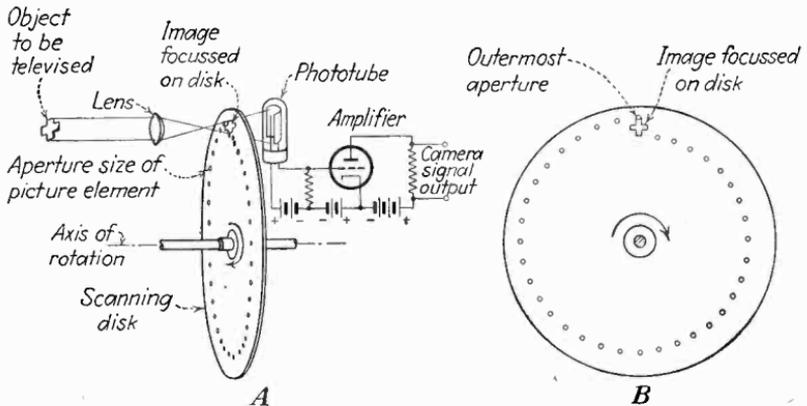
FIG. 43.—Elementary rotating-disk scanning. The 36 apertures, arranged in a spiral, scan the image in a succession of 36 lines, passing the light to the phototube. This method is limited by the small amount of light contained in each scanning aperture.
