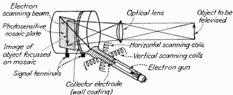
FIG. 9.—Diagrammatic view of the operation of the iconoscope camera tube.
