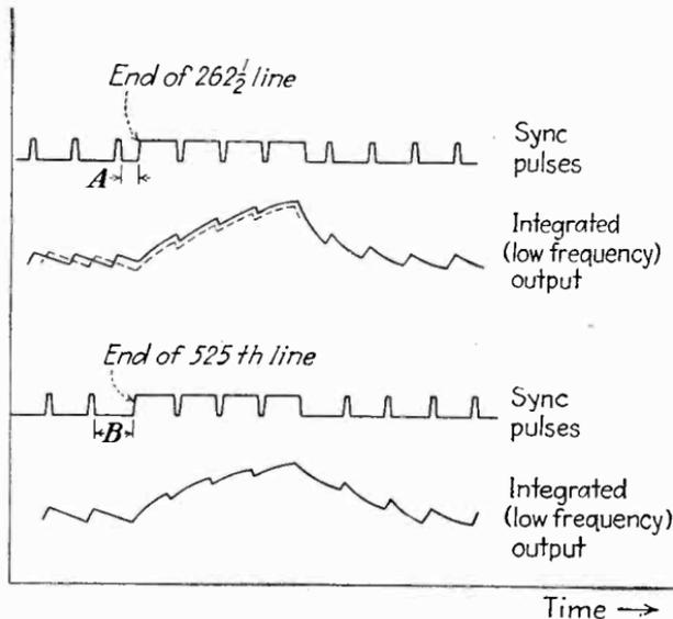
FIG. 97.—Effect of half-line difference in successive fields on integrated vertical sync pulse. The dashed line in the upper figure is the lower figure superimposed. The difference between the two integrated pulses is made negligibly small by the insertion of equalizing pulses (*cf.* Fig. 93).
