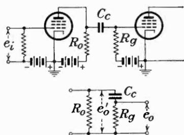
FIG. 122.—Uncompensated amplifier with equivalent low-frequency circuit.
