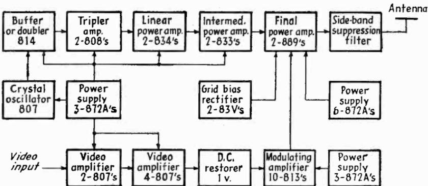
FIG. 269.—Tube line-up of a typical 1000-watt picture transmitter manufactured by the RCA Manufacturing Co.
