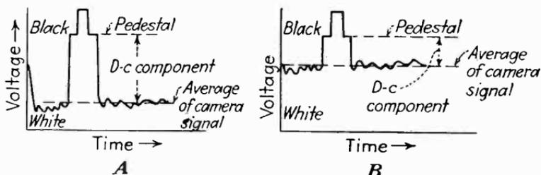
Fig. 247.—Control of the average picture brightness by variation of the pedestal height. By increasing the pedestal height in the control amplifier, the picture may be made brighter, provided the pedestal height remains constant in the rest of the transmission system.
