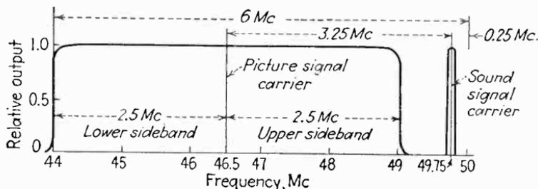
FIG. 147.—Double sideband television channel, now superseded by the vestigial system in the United States.
