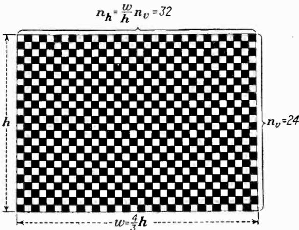
Fig. 14.—Relationship between vertical and horizontal resolution when picture-element spacing is equal in the two dimensions. The total number of picture elements is then  $\frac{4}{3} \times n_v^2$ , where  $n_v$  is the number in the vertical dimension and  $\frac{4}{3}$  is the ratio of the picture's width to its height.
