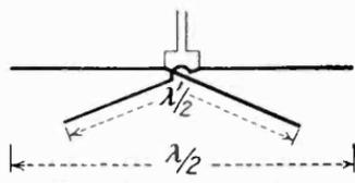
FIG. 173.—Double doublet, designed for two operating wavelengths,  $\lambda$  and  $\lambda'$ , which displays good response within those limits.
