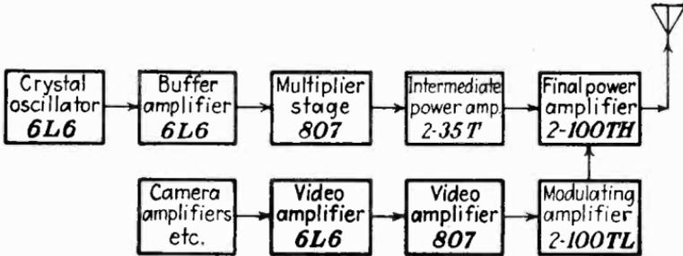
FIG. 268.—Tube line-up of a typical 50-watt picture transmitter, station W2XVT, Passaic, N. J.
