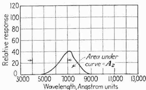
FIG. 40.—Response of the photoelectric surface to the spectral distribution of Fig. 39, determined by multiplying the curves in Figs. 35 and 39. The area under this curve,  $A_2$ , is compared with the area  $A_1$  under the curve in Fig. 36 to obtain the value of luminous sensitivity to the nonstandard light source.
