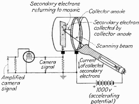
FIG. 51.—Electrical connections of the signal circuit of an iconoscope tube. The series connection between mosaic and collector is completed by the passage of secondary electrons, which constitute the output signal current of the tube. (For the optical action of the iconoscope, see Fig. 9 page 18.)
