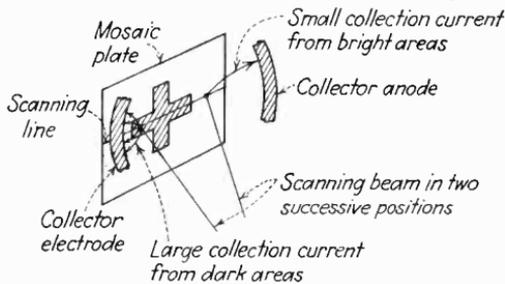
FIG. 52.—Difference in collection current between dark and bright areas on the mosaic. The photoelectric emission from the dark areas is small, hence the retarding field is small and the secondary emission (induced by the scanning beam) is large. In bright areas the reverse condition exists, and the collection current is small. Hence the output current is "negative" relative to the brightness differences.
