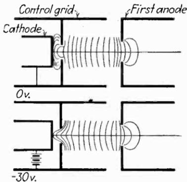
FIG. 64.—Variations in contours with control-grid potential. Top, with cathode and grid at same potential, the field at the cathode surface is strong and widespread. Bottom, with the control grid 30 volts negative, the field is weaker and covers a smaller area of the cathode. (After Maloff and Epstein.)
