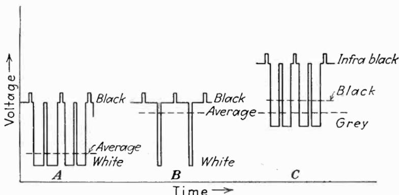
FIG. 261.—Variation of the average of the video signal: *A*, white image with narrow black bar; *B*, black image with narrow white bar, with blanking level held same as in *A*; *C*, white image with narrow black bar, as in *A*, but with average coinciding with average in *B*. Most of the signal in *C* is lost above the black level, due to the upward displacement of the average.
