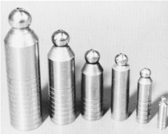
FIGURE 4.16.3 Ball-joint members and other spherical surfaces are given an accurate finish by honing. (Courtesy XLO Micromatic.)
