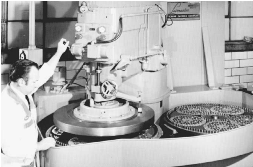
FIGURE 4.16.8 A production lapping machine for flat surfaces. Parts can be unloaded and loaded on one table while lapping takes place on the other table. (Courtesy Lapmaster Division, Crane Packing Co.)
