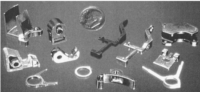
FIGURE 3.16.1 A collection of typical metal injection molded parts. (Photo courtesy of Precision Castparts Corporation.)
