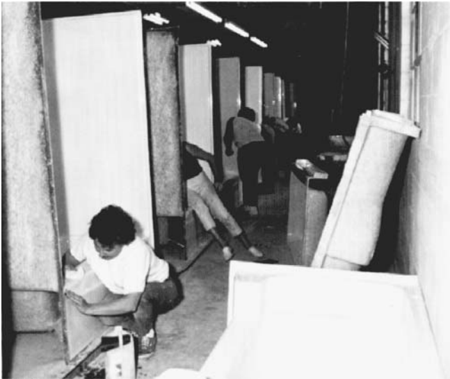
FIGURE 6.6.2b Tub and shower units made by the spray-up process. (Courtesy Universal-Rundle Corp.)
