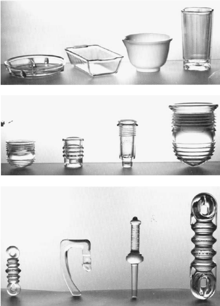
FIGURE 6.11.3 Examples of pressed glassware. (a) Block-mold glassware. (b) Split-mold glassware. (c) Font-mold glassware. (Courtesy Corning Glass Works.)
