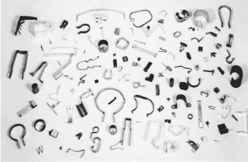
FIGURE 3.4.2 Parts that involve relatively complex forming can usually be more economically produced on four-slides. (Courtesy Torin Corporation.)
