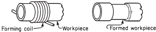
FIGURE 3.15.4 Compression forming of tubing. (From Metals Handbook, American Society for Metals.)
