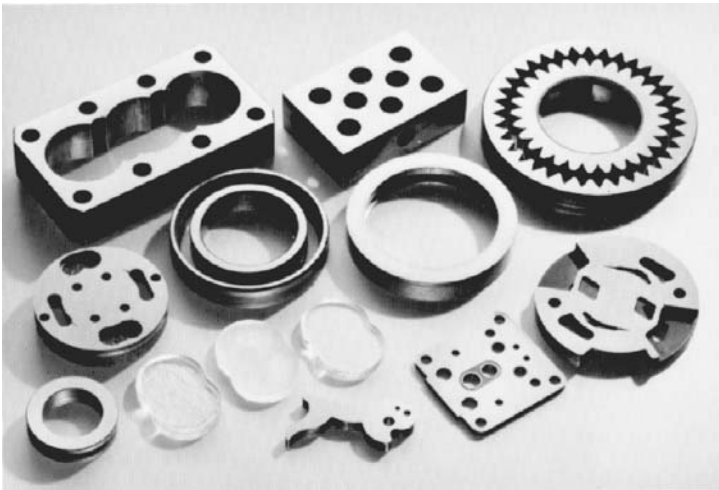
FIGURE 4.16.9 Collection of typical flat lapped parts. ( Courtesy of Lapmaster Division, Crane Packing Co. )
