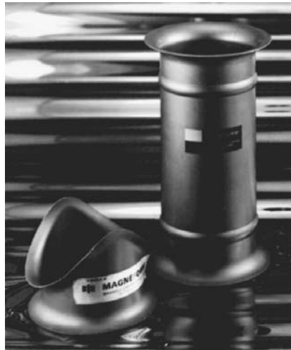
FIGURE 3.15.6 Typical components produced with the aid of electromagnetic forming. (a) Lightning-reflector facets. (b) Automotive cruise-control assembly. (c) Aircraft ducting.
