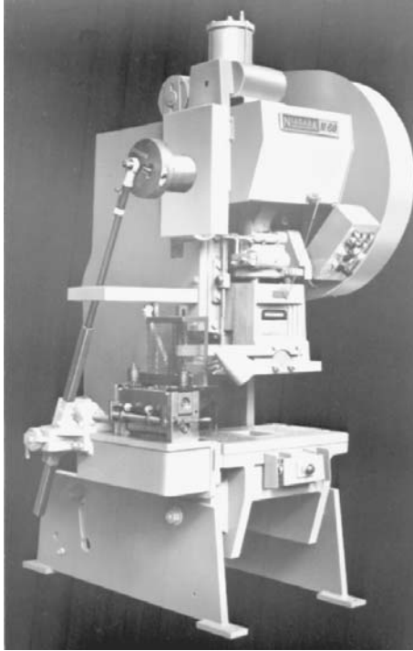
FIGURE 3.2.1 Typical crankshaft-type punch press. Coiled sheet metal is fed through the die automatically. Finished parts are ejected through the open back of the press. (Courtesy Niagara Machine & Tool Works.)
