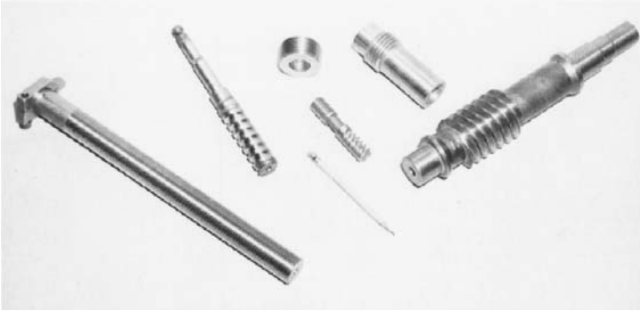
FIGURE 4.13.1 Thread grinding, performed on the parts shown, is typical of the kind of operations that can be performed on center-type grinding machines. (Courtesy Jones & Lamson, Waterbury Farrel Division of Textron, Inc.)
