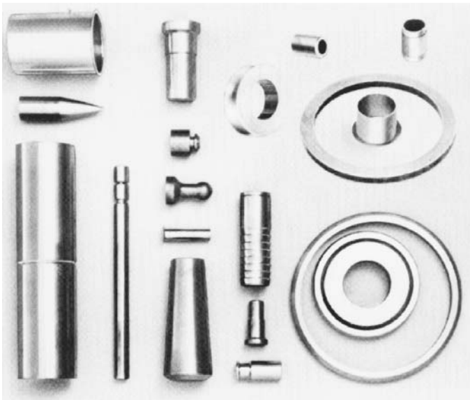
FIGURE 4.2.5 Typical parts cut off with lathe-type cutoff machines. ( Courtesy Modern Machine Tool Co. )
