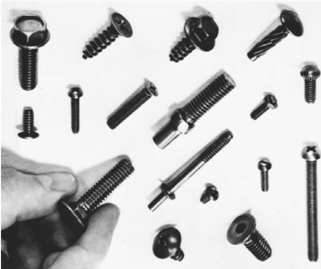
FIGURE 3.7.3 Combination cold-heading and thread-rolling machines form these completed fasteners. ( National Machinery Co. )
