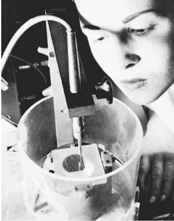
FIGURE 4.21.1 Abrasive jet linked to a pantograph cuts intricate patterns in silicon semiconductors. (Courtesy S. S. White Industrial Products.)
