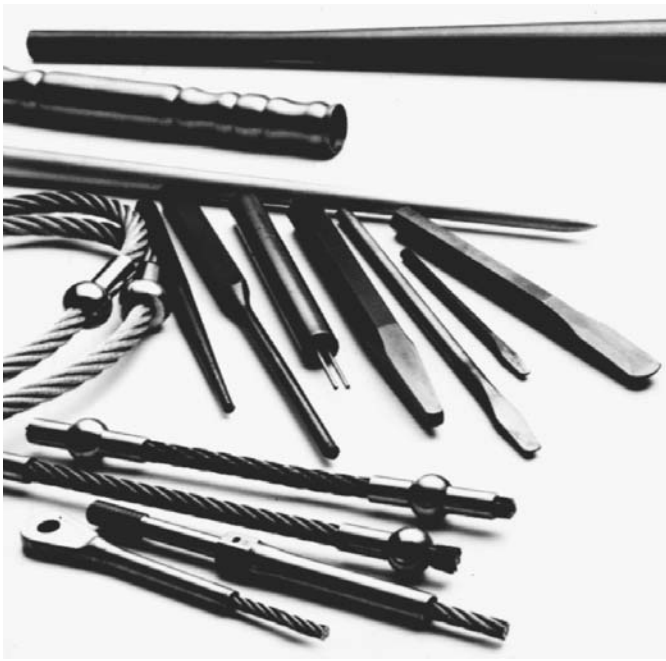
FIGURE 3.9.3 Examples of parts that are rotary-swaged. Note, in addition to the tapered pieces produced on conventional two- or four-die rotary swagers, the convoluted part and cable assemblies made on die-closing machines and parts with rectangular cross sections made on stationary die machines. (Courtesy Fenn Mfg. Co.)
