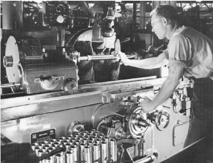
FIGURE 4.8.14 Center-type thread grinding. (Courtesy Teledyne Landis Machine.)
