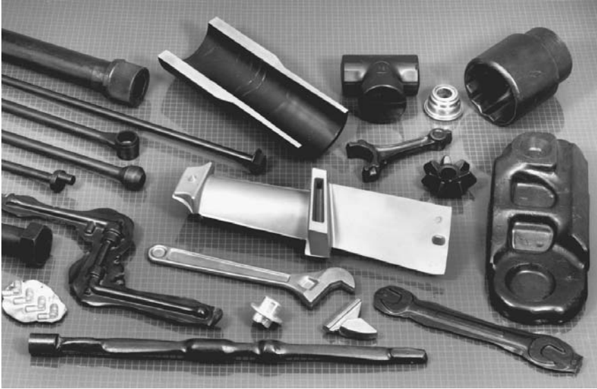
FIGURE 3.13.3 A collection of typical forgings. Note that some still have flashing attached. (Courtesy National Machinery Company.)
