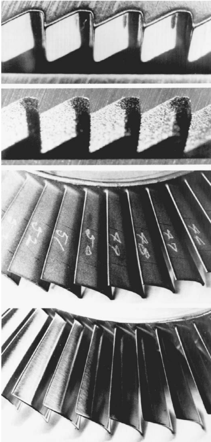
FIGURE 4.21.3 Examples of parts processed with abrasive-flow machining. (a) Deburring and polishing ratchet teeth. (b) Polishing turbine blades. (Courtesy Extrude Hone Corp.)
