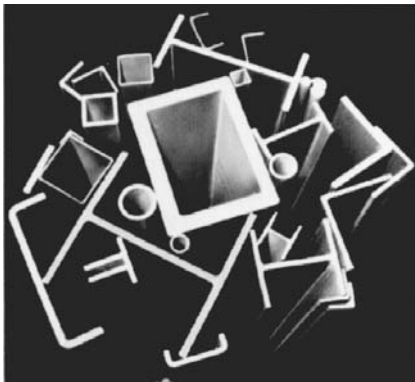
FIGURE 6.6.2j Typical cross-sectional shapes which can be produced by pultrusion. (Courtesy Morrison Molded Fiber Glass Co.)
