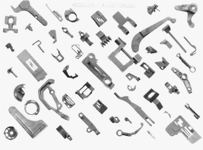
FIGURE 5.3.2 Collection of investment-cast parts. Note their complexity and size, as indicated by the 6-in ruler. (Courtesy The Singer Company.)
