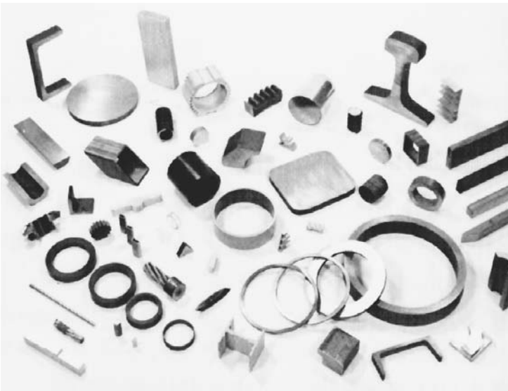
FIGURE 4.2.3 Typical parts and shapes cut by abrasive saws. (Courtesy W. J. Savage Co.)
