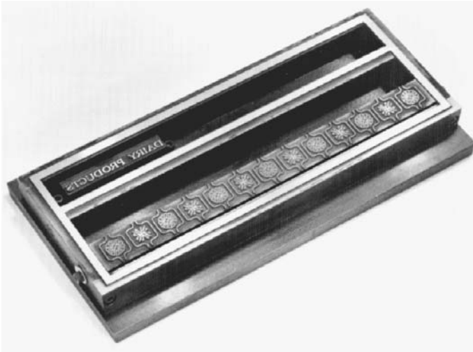
FIGURE 6.12.10 An engraved hot-stamp die. The die will be heated to the transfer temperature of the foil (about 275°F, or 135°C). When it is pressed against the part, an exact duplicate of the die pattern will transfer. Note the intricate detail that this process can transfer. (Courtesy Service Tectonics Instrument, Detroit, Mich.)
