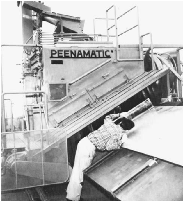
FIGURE 8.7.1 Forming an aircraft-wing panel by peening. ( Courtesy Metal Improvement Co. )
