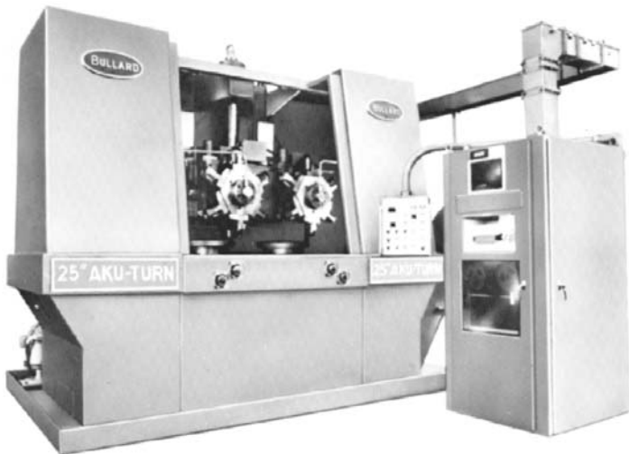
FIGURE 4.4.5 Vertical double-spindle chucking machine. (Courtesy The Bullard Company.)
