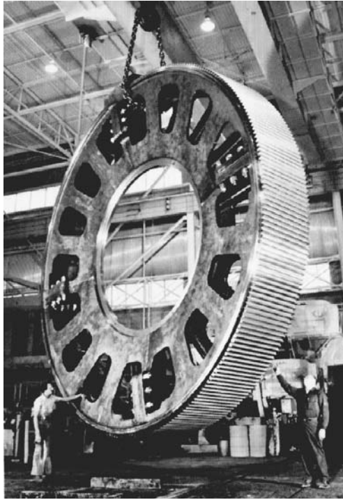
FIGURE 4.22.1 This helical ring gear for an ore-grinding mill is 24 ft in diameter and over 3 ft wide; it weighs 70 tons. (Courtesy The Falk Corporation, subsidiary of Sundstrand Corporation. )
