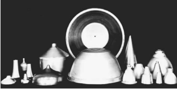
FIGURE 3.6.3 Typical parts produced by metal spinning. (Courtesy Autospin, Inc.)
