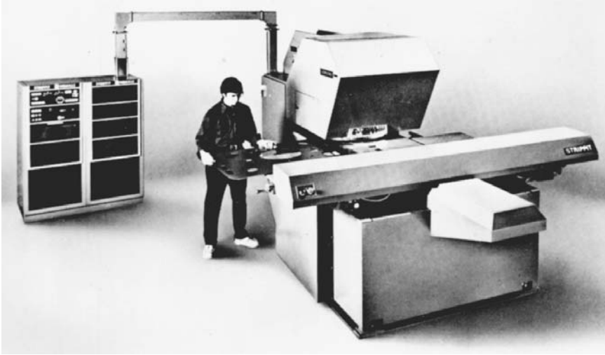
FIGURE 3.2.5 Turret punching machine equipped with computer control. (Courtesy Strippit-Houdaille.)
