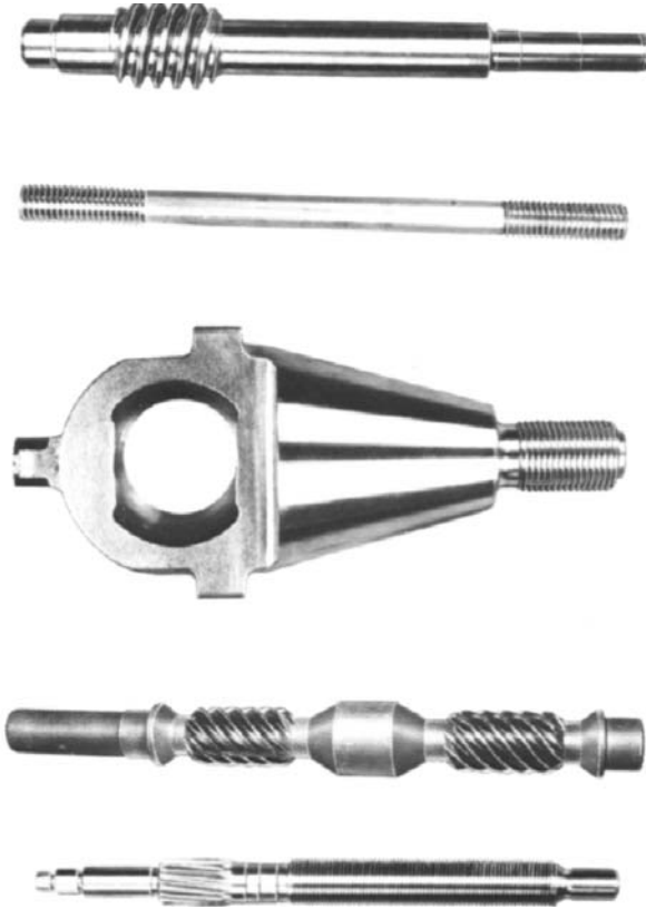
FIGURE 4.8.18 Typical parts with rolled threads. (Courtesy Teledyne Landis Machine.)
