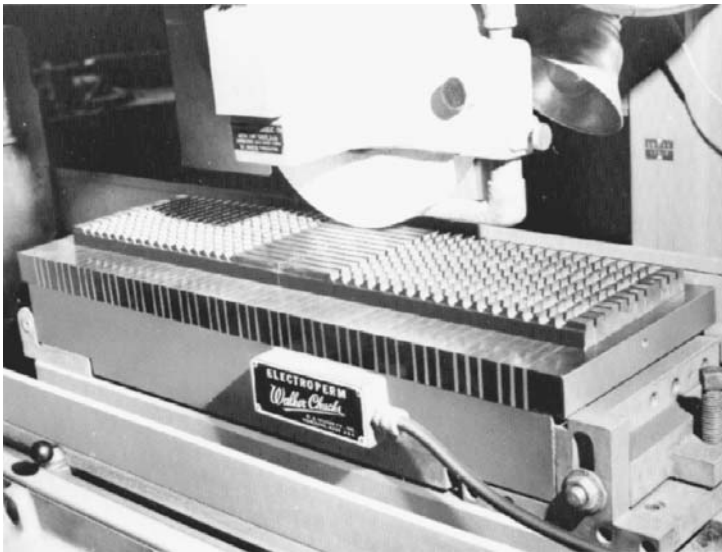
FIGURE 4.15.4 Series of broaching-tool elements being surface-ground. (Courtesy O. S. Walker Co., Inc.)
