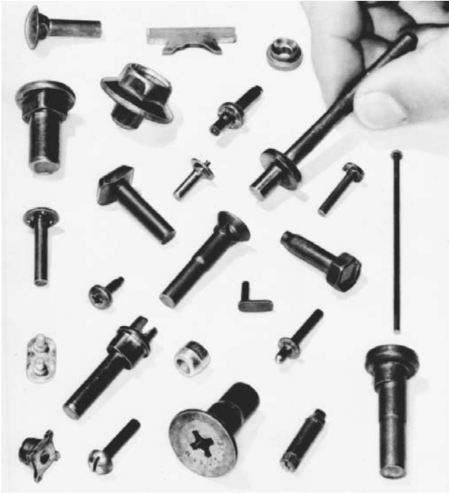
FIGURE 3.7.2 One die and two punches form these double-blow cold-headed parts. ( National Machinery Co. )
