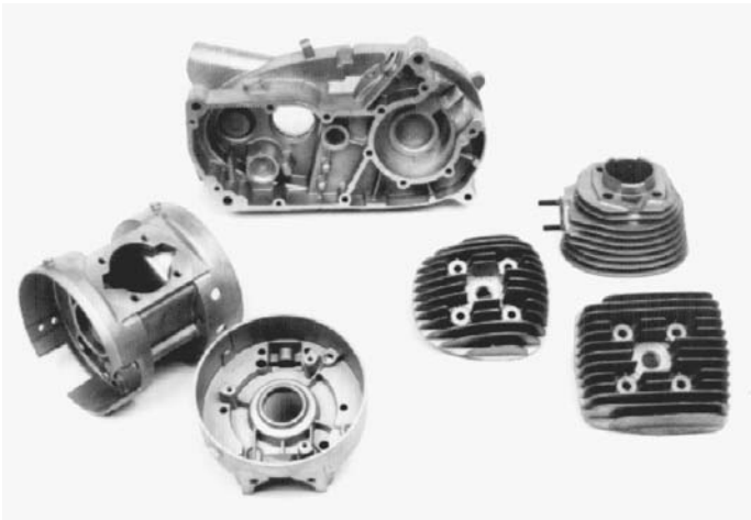
FIGURE 5.4.3a These aluminum die castings for a motorcycle engine show how good design can provide ribs where needed for strength and cored holes for fastening while maintaining fairly constant wall thickness. (Courtesy Aluminum Industrie Vaasen.)
