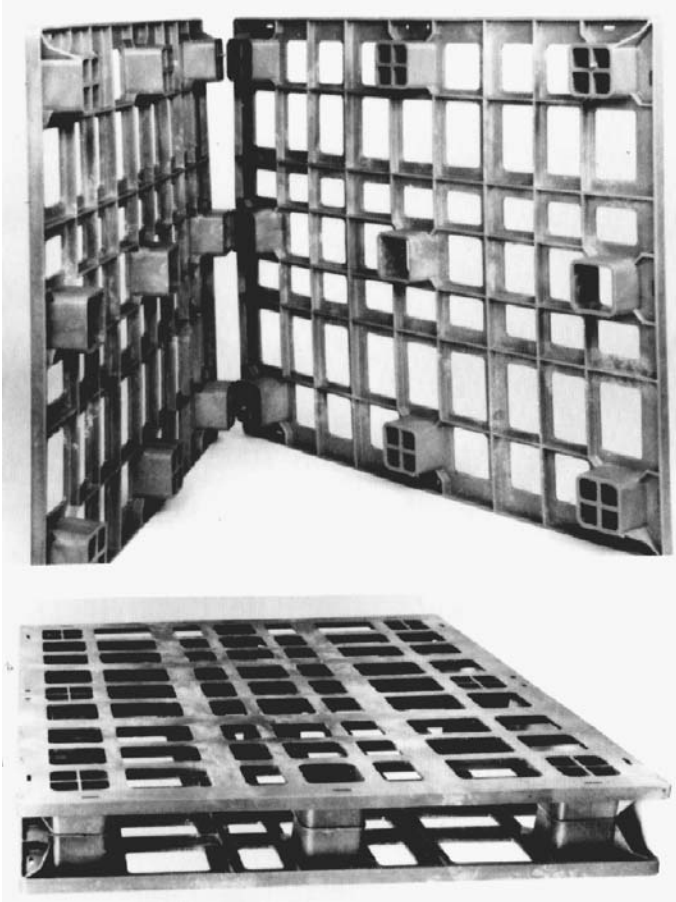
FIGURE 6.3.2 Structural-foam industrial pallet, molded in two pieces that are hot-plate-welded together. (Courtesy Union Carbide Corp.)
