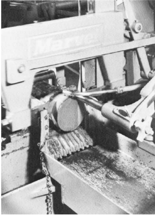
FIGURE 4.2.1 Hacksaw cutoff of bar stock. (Courtesy Armstrong-Blum Mfg. Co.)
