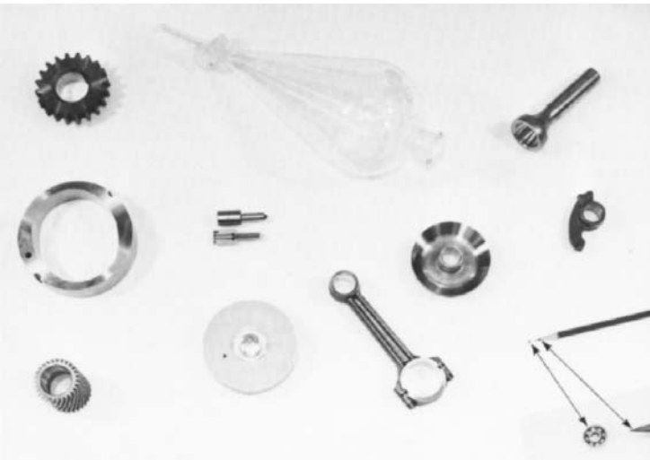
FIGURE 4.12.3 Typical internally ground parts. (Courtesy Bryant Grinder Corporation.)
