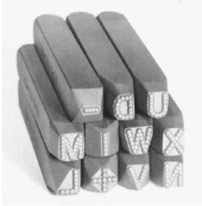
FIGURE 8.6.5 Low stress-inducing type for stamp-indented markings. (Courtesy Pannier Corporation.)
