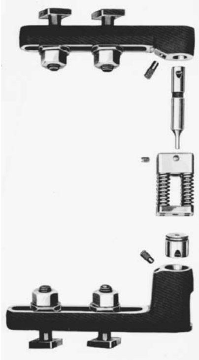
FIGURE 3.2.8 Exploded view of a punch-die combination used with a master reusable die set. The stripper is self-contained, and holes of different sizes and shapes can be produced by changing to the appropriate punch and die inserts. (Courtesy S. B. Whistler & Sons, Inc.)
