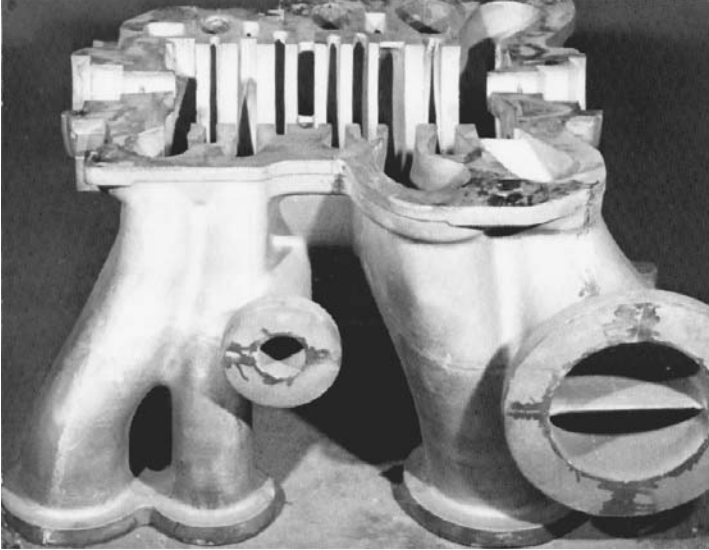
FIGURE 5.1.2 This turbine manifold is an example of the complexity of part that can be produced by sand-mold casting. (Courtesy Meehanite Worldwide Division of Meehanite Metal Corporation.)
