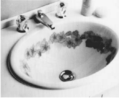
FIGURE 6.6.2c Acrylic-faced hand-bowl unit made by vacuum forming and spray-up (rigidizing). (Courtesy J. S. Johns Co.)
