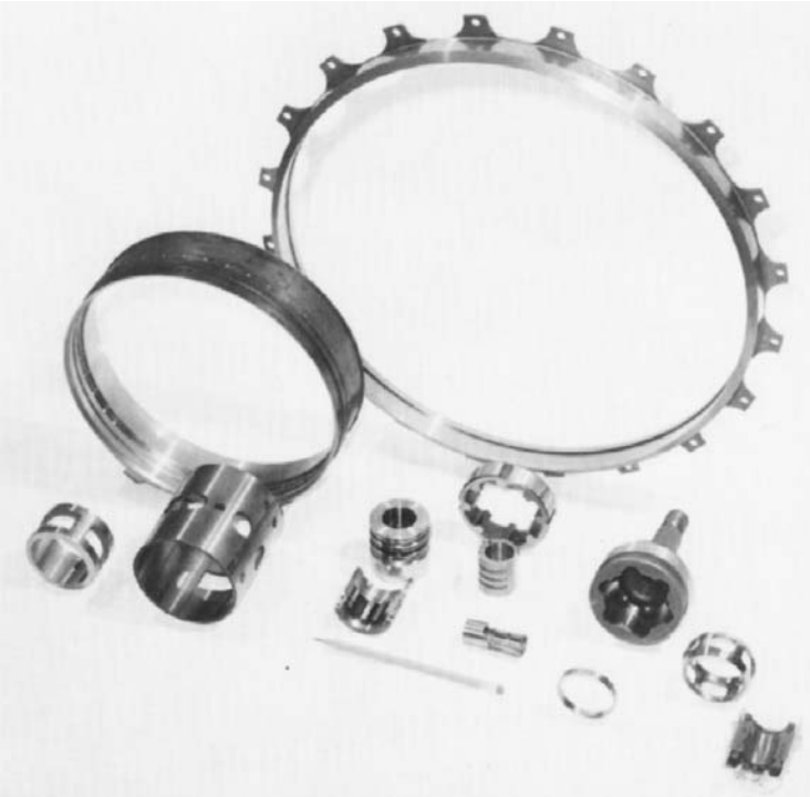
FIGURE 4.12.2 Typical internally ground parts. The internal surfaces of these parts are routinely ground despite thin walls, interruptions, and special contoured cross sections. (Courtesy Bryant Grinder Corporation.)
