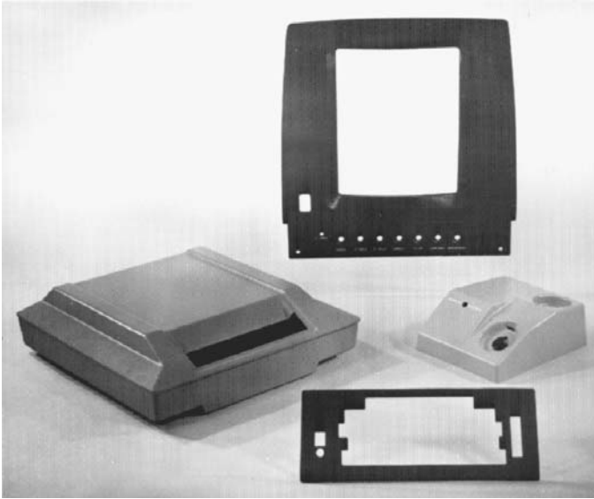
FIGURE 6.8.2 Business-machine housings and other parts produced by thermoforming. (Courtesy Mercury Plastics Corp.)
