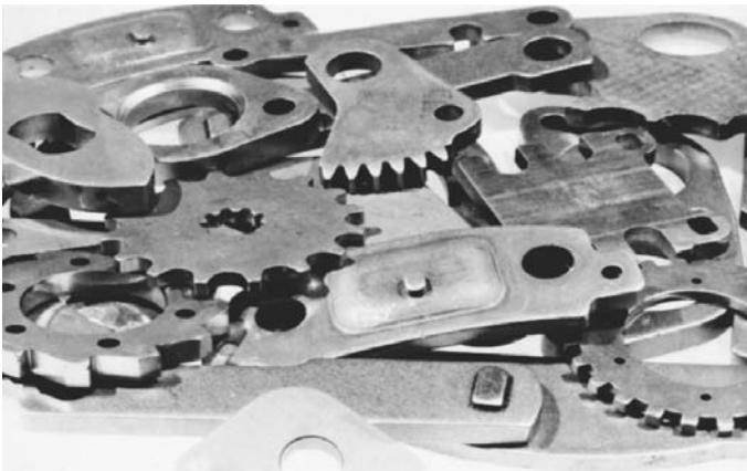
FIGURE 3.3.8 A collection of typical fine-blanked parts. (Courtesy American Feintool, Inc.)
