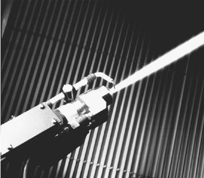
FIGURE 8.3.11 An HVOF (high-velocity oxygen fuel) gun in operation. (Courtesy Sulzer Metco.)
