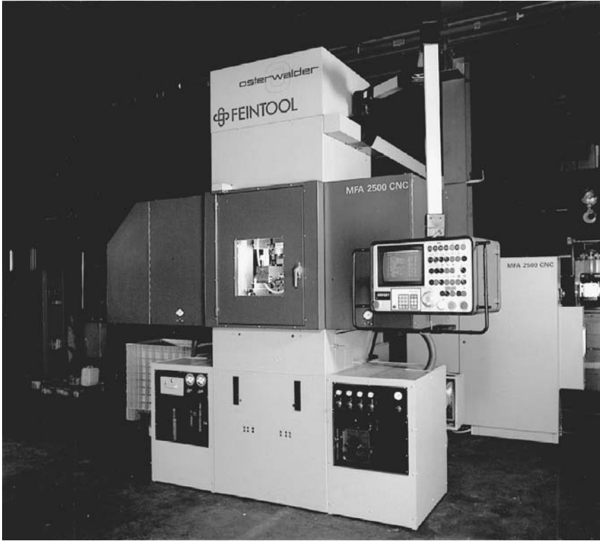
FIGURE 3.3.1 A 250-ton fine-blanking press. (Courtesy American Feintool, Inc.)
