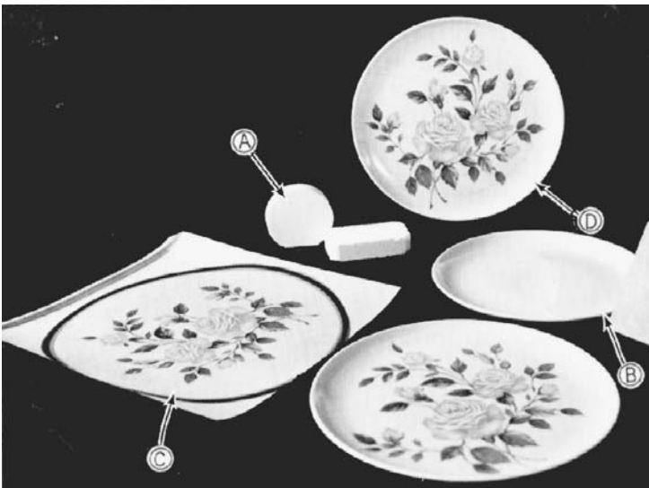
FIGURE 6.12.18 Materials that make melamine dinnerware. (A) Melamine powder in a preform. (B) Molded-melamine plate without the overlay sheet. (C) The printed overlay sheet. (D) Molded decorated melamine plate.
