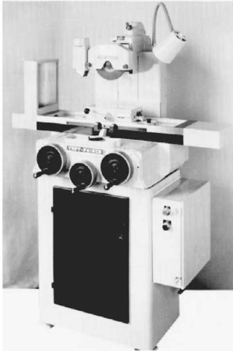
FIGURE 4.15.2 Typical horizontal-spindle reciprocating-table surface grinder. (Courtesy Taft-Peirce Manufacturing Co.)
