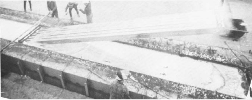
FIGURE 8.3.3 The galvanized steel is withdrawn from the clean molten-zinc bath. The zinc layer is now metallurgically bonded to the steel. (Courtesy St. Joe Lead Company.)
