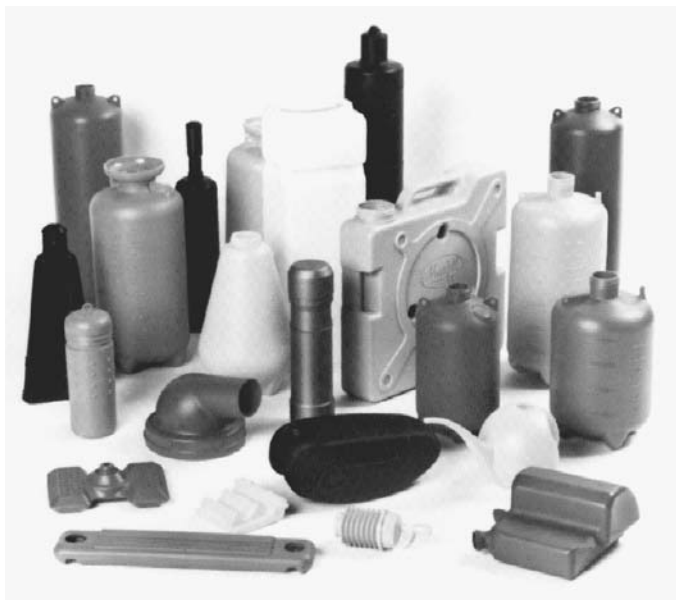
FIGURE 6.5.1 Collection of typical blow-molded articles. (Courtesy Air-Lock Plastics, Inc.)
