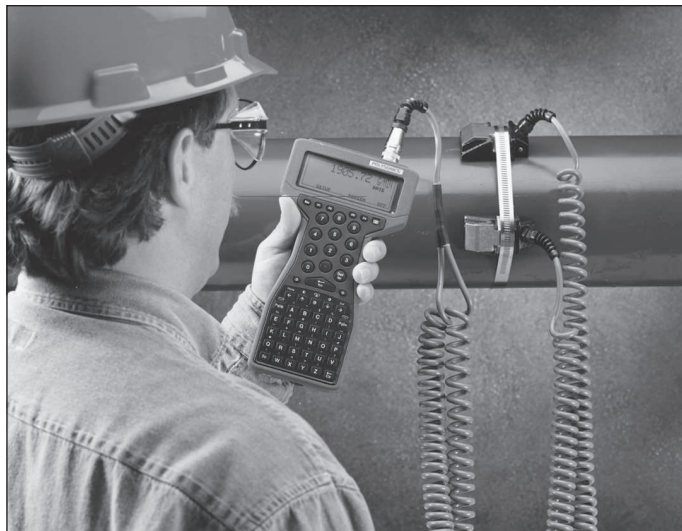
Fig. 6.35 Ultrasonic flowmeters: (a) pulse type; (b) doppler-shift type (from Ref. 41); (c) a portable noninvasive installation (Courtesy of Thermo Polysonics, Houston, TX.)
