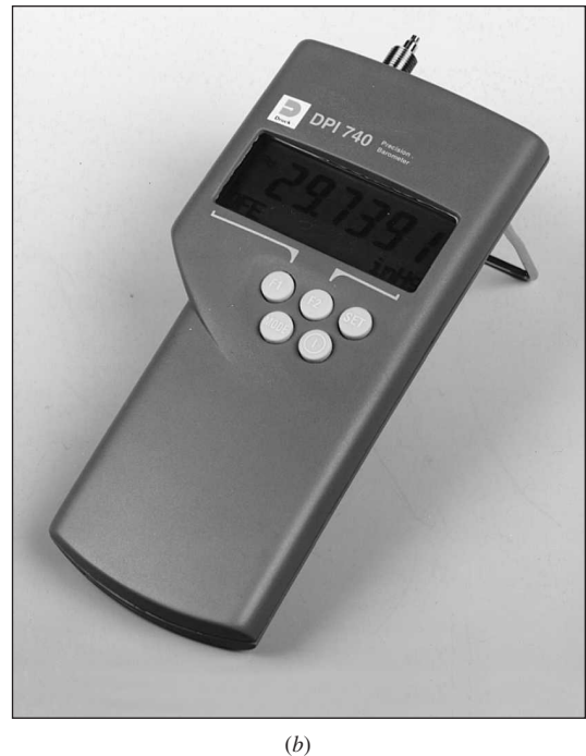
Fig. 2.6 A barometer measures local absolute atmospheric pressure: (a) the height of a mercury column is proportional to p_{\text{atm}} ; (b) a modern portable barometer, with digital readout, uses the resonating silicon element of Fig. 2.28c. (Courtesy of Paul Lupke, Druck, Inc.)
