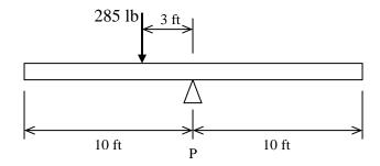
12. A simply supported beam 50 feet in length is loaded as shown below. Calculate the vertical reaction forces at each end of the beam.
