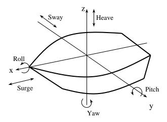
**Figure 1.16** A ship's axes and degrees of freedom
