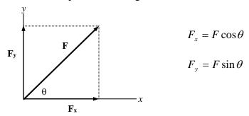
**Figure 1.6** Resolution of a vector into its components
