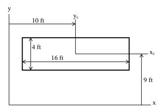
Figure 1.15 Illustrating the parallel axis theorem
