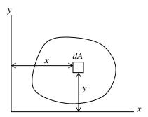
Figure 1.10 Diagram used for moment of area calculations
