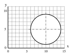
15. Determine the centroid of the shape below about both the x and y axes.
