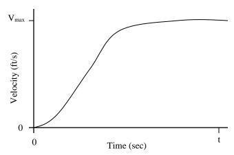
Figure 1.2 Ship's speed as a function of time
