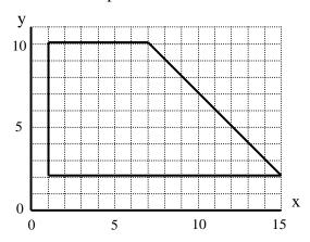
16. Determine the centroid of the shaded area about the x and y axes.
