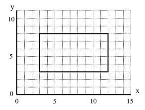
14. Determine the first moment of area of the shape below about both the x and y axes.
