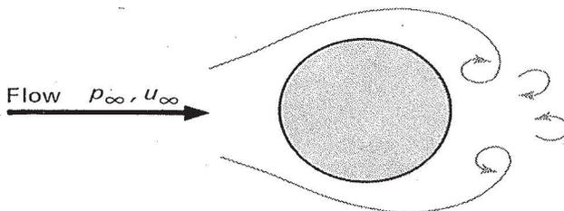
Fig. 6-5 Cylinder in cross flow.
