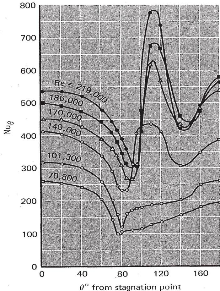
late flow separation. Consequently, the form drag is reduced, and this is represented by the break in the drag-coefficient curve at about  $Re = 3 \times 10^5$ . The same reasoning applies to the sphere as to the circular cylinder. Similar behavior is observed with other bluff bodies, such as elliptic cylinders and airfoils.
