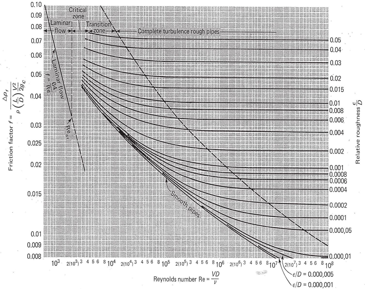
Fig. 6-4 Friction factors for pipes, from Ref. 5.
