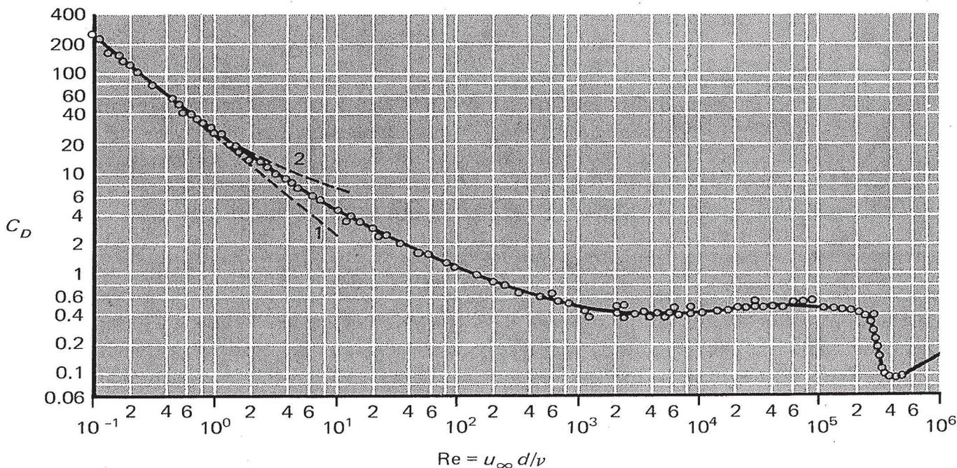
Fig. 6-8 Drag coefficient for spheres as a function of the Reynolds number, from Ref. 6.
