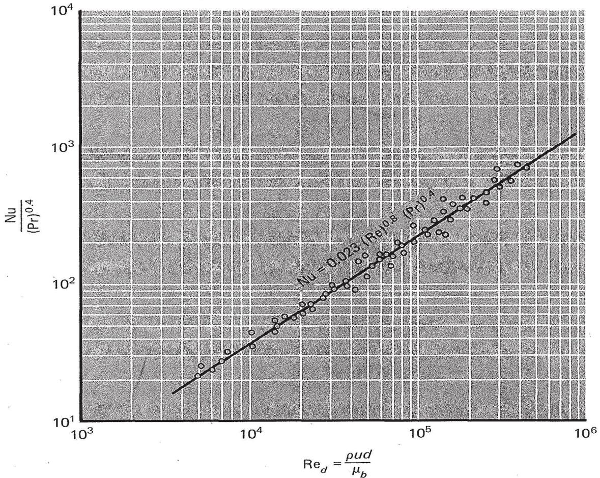
Fig. 6-2 Typical data correlation for forced convection in smooth tubes, turbulent flow.
