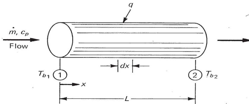
Fig. 6-1 Total heat transfer in terms of bulk-temperature difference.
