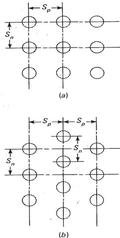
**Fig. 6-12** Nomenclature for use with Table 6-3: (a) in-line tube rows; (b) staggered tube rows.
