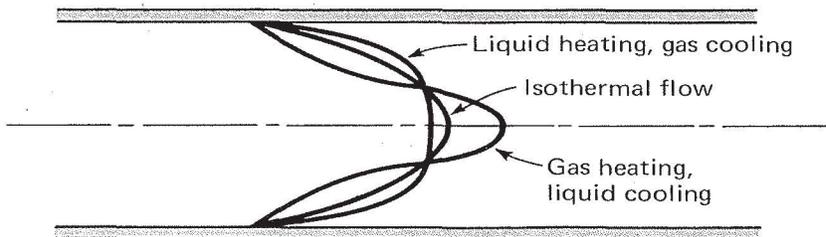
Fig. 6-3 Influence of heating on velocity profile in laminar tube flow.
