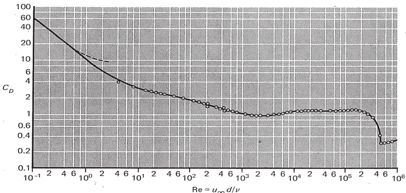
Fig. 6-7 Drag coefficient for circular cylinders as a function of the Reynolds number, from Ref. 6.
