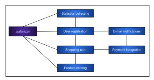
As you can see, we use a **balancer** to route requests to microservices. You can actually connect to microservices directly from the frontend application.
