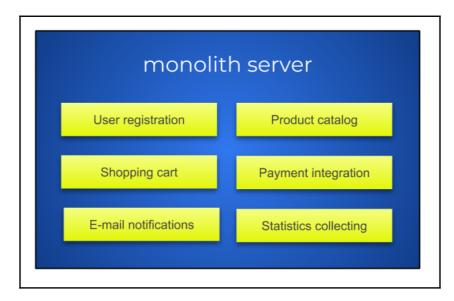
In reality, the real server contains more modules than this, but we have separated them into logical groups based on the tasks they perform. This is a good starting point to breaking your monolith into multiple, loosely coupled microservices. In this example, we can break it further into the pieces represented in the following diagram:
