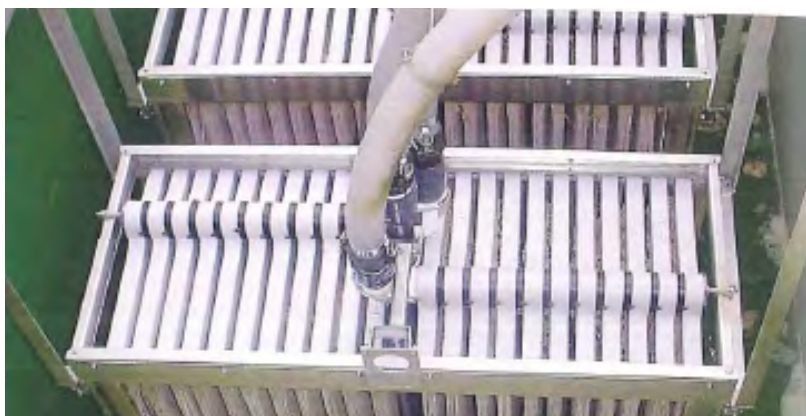
Figure 8.7 module cassettes during In-air cleaning
