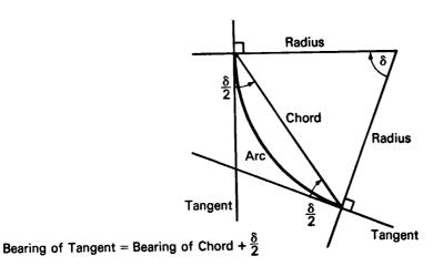
The bearing of the second radius is from the center of the arc to the other end, and the distance is entered as a *negative* number to signal to the computer that this and the prior leg are not perimeter legs, but auxiliary legs of an arc.
