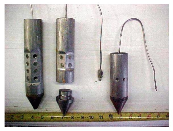
**Figure C-2. Waterloo Profiler™ tip configurations.** (Source: The Johnson Company Inc., Montpelier, VT)
