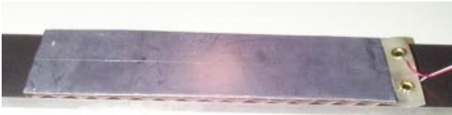
Figure 4.6: Prototype #2 distributed absorber with a constant mass distribution
