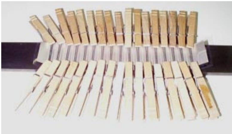
Figure 4.9: PVDF taking its corrugated shape, hold in place with clothes pegs
