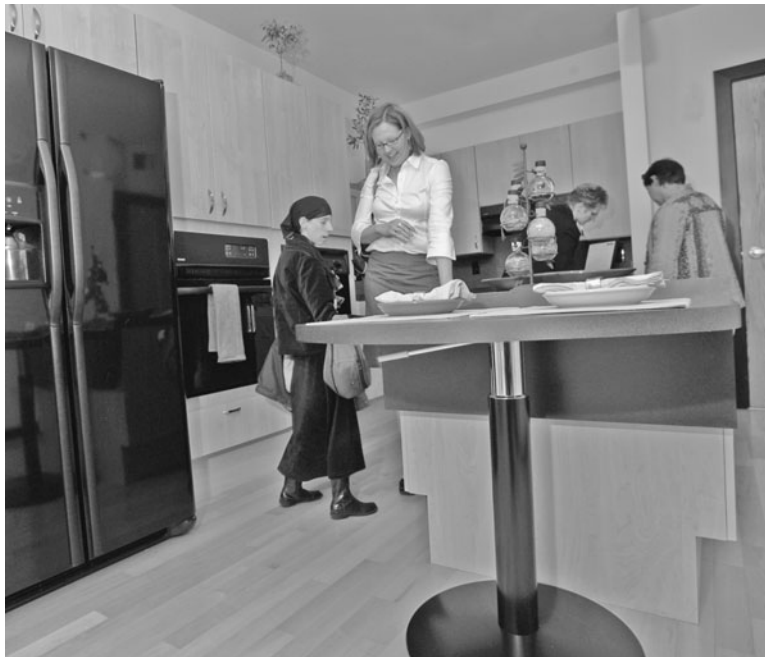
FIGURE 24.4 Easy-to-operate countertop adjusts in height from 28 to 42 in. (Wendi Fitzgerald, photographer for Starkloff Disability Institute.)
