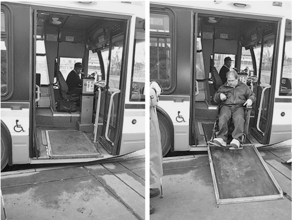
FIGURE 19.3 Low-floor buses have ramps to bridge the horizontal and vertical gaps from the boarding platform, sidewalk, or street. The two photographs show a folding ramp in the stowed position and a wheelchair user descending a deployed ramp.
