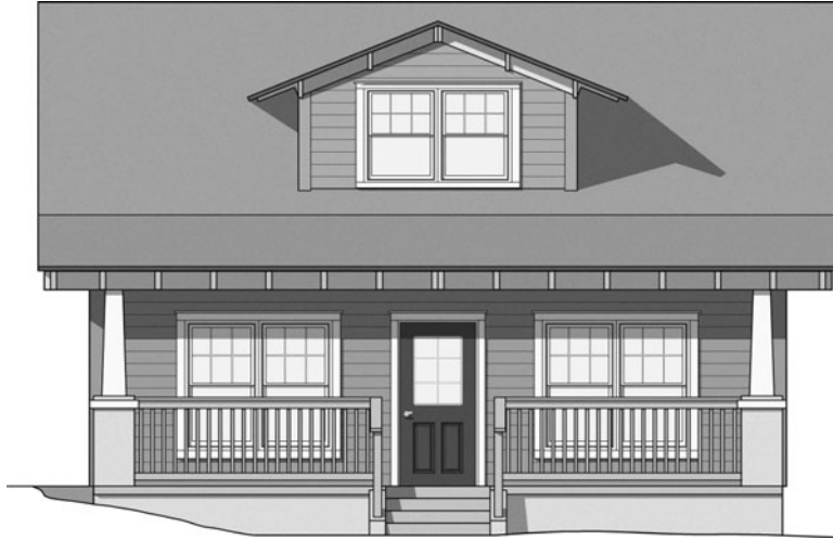
FIGURE 25.2 This three-bedroom, two-bathroom American Craftsman Bungalow single-family house, while initially inaccessible due to the front porch, was redesigned to include a cross-sloping lot with an on-grade front entry. The space-efficient plan contains generous circulation clearances, an L-shaped kitchen, one visitable full bathroom, and two accessible bedrooms. (Image courtesy of Steinfeld and White, 2010.)
