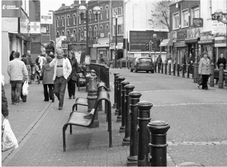
FIGURE 17.1 Too many bollards and street furniture in this secondary street are aesthetically displeasing, but they also restrict movement and create irritating or even dangerous obstructions for parents with strollers and for disabled people.
