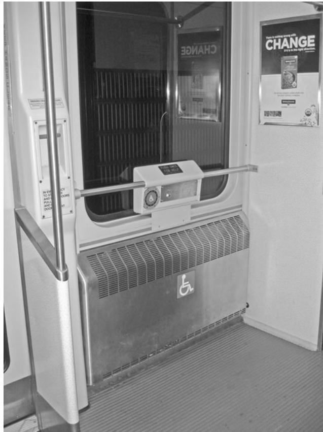
FIGURE 19.5 This low-floor light-rail transit vehicle has wheelchair seating marked by the international symbol of accessibility (ISA). A large button, also marked by the ISA, is provided to request help from the train operator when the passenger wishes to have the ramp deployed. A two-way intercom is also provided.
