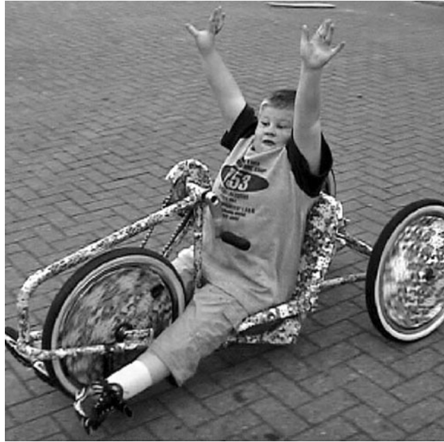
FIGURE 36.2 The award-winning Tilting Trike by RCA design products graduate Ben Wilson (2002). This new pedal-powered tricycle for children can be adapted to the needs of those without lower body strength.
