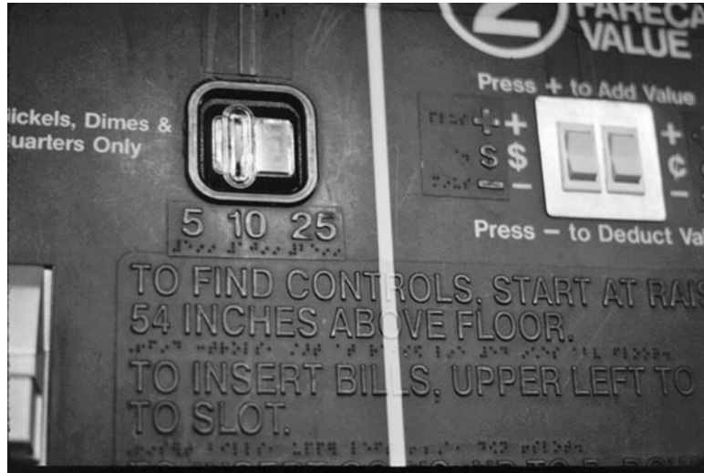
FIGURE 4.4 Subway fare machines with high-contrast and tactile lettering and audible output on demand.
