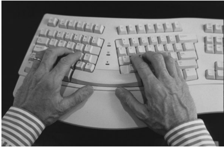
FIGURE 32.6 Ergonomic keyboards allow wrists to maintain neutral postures while typing.
