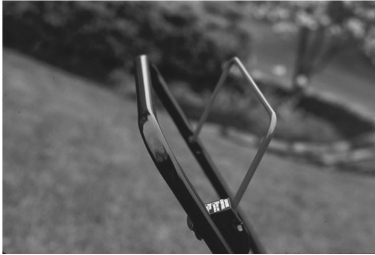
FIGURE 4.5 The “dead-man” switch on a lawn mower handle requires conscious use.
