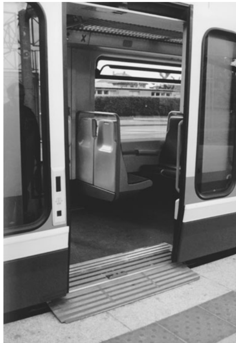
FIGURE 12.2 Horizontal accessibility from the platform. A retractable door step facilitated the leveling with the sidewalk. (Photo by the author.)
