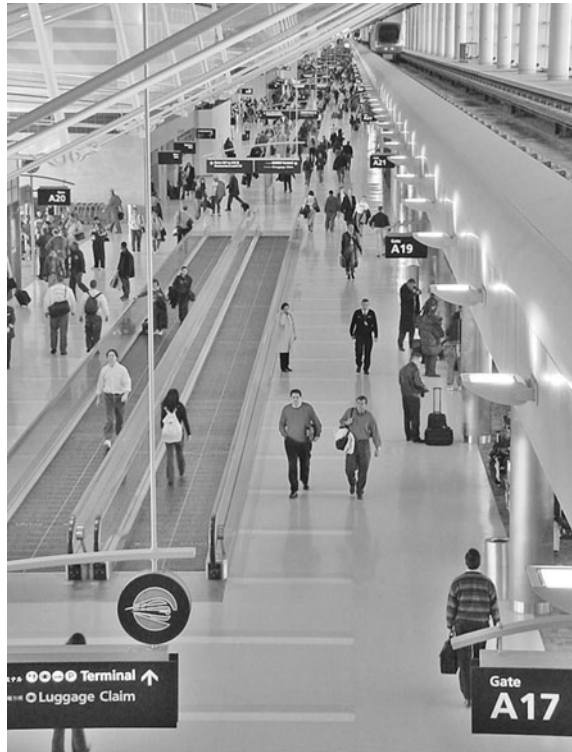
FIGURE 19.1 The Detroit Metro Airport has three methods of circulation: a wide pedestrian promenade, sliding walkways located in the middle of the promenade, and an elevated electric train link.
