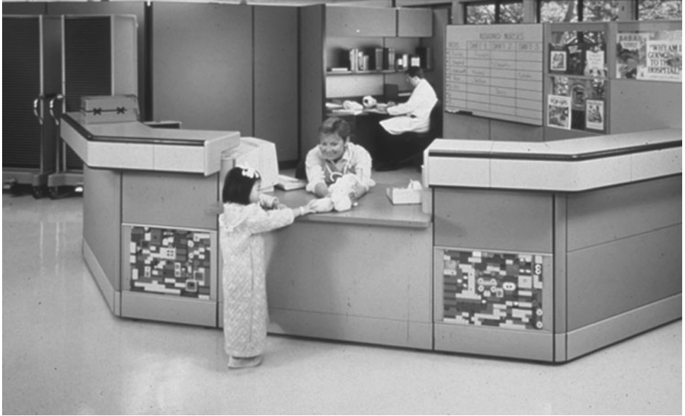
FIGURE 4.7 Lowering one section of the nurses' station counter in a hospital suits the needs of visitors who are shorter or seated in a wheelchair or scooter.
