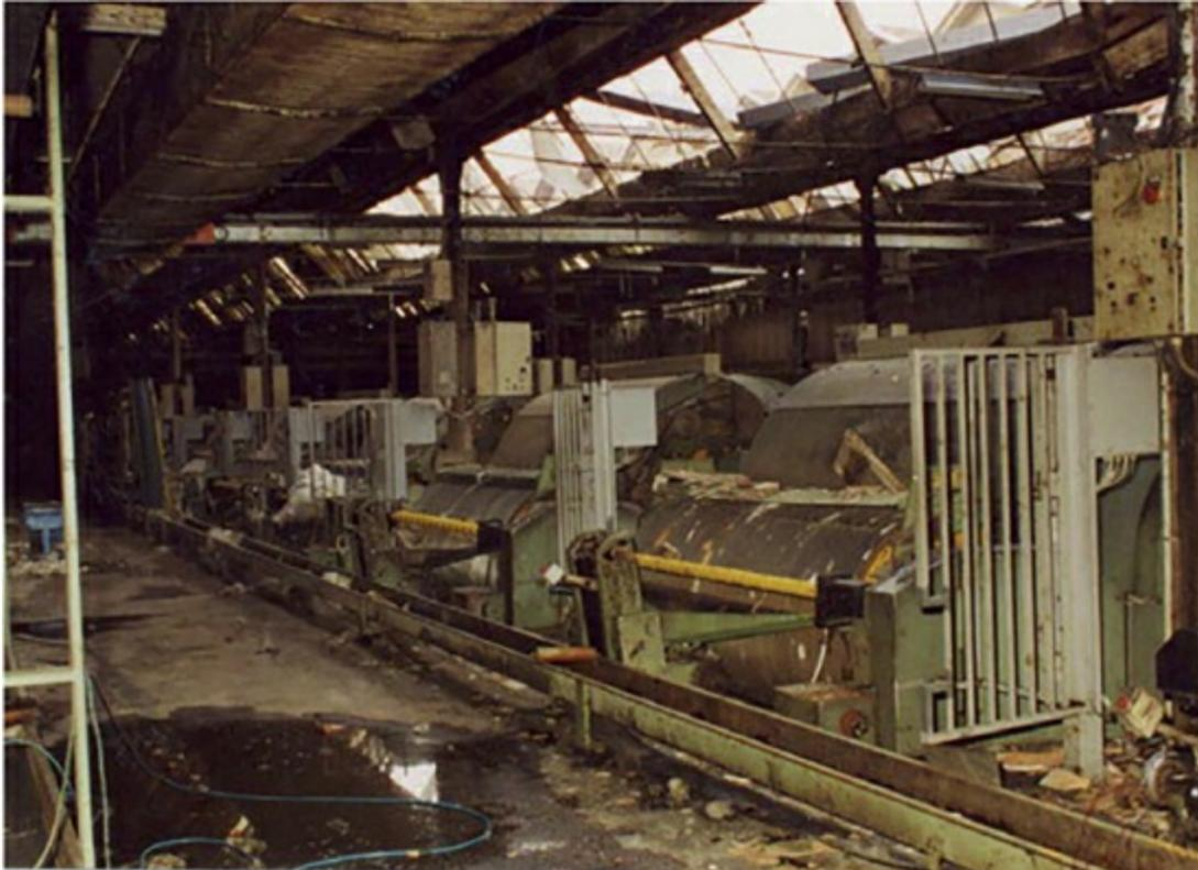
[Figure 4.21](#) Explosion of wool burrs, state of the places, card rooms.
