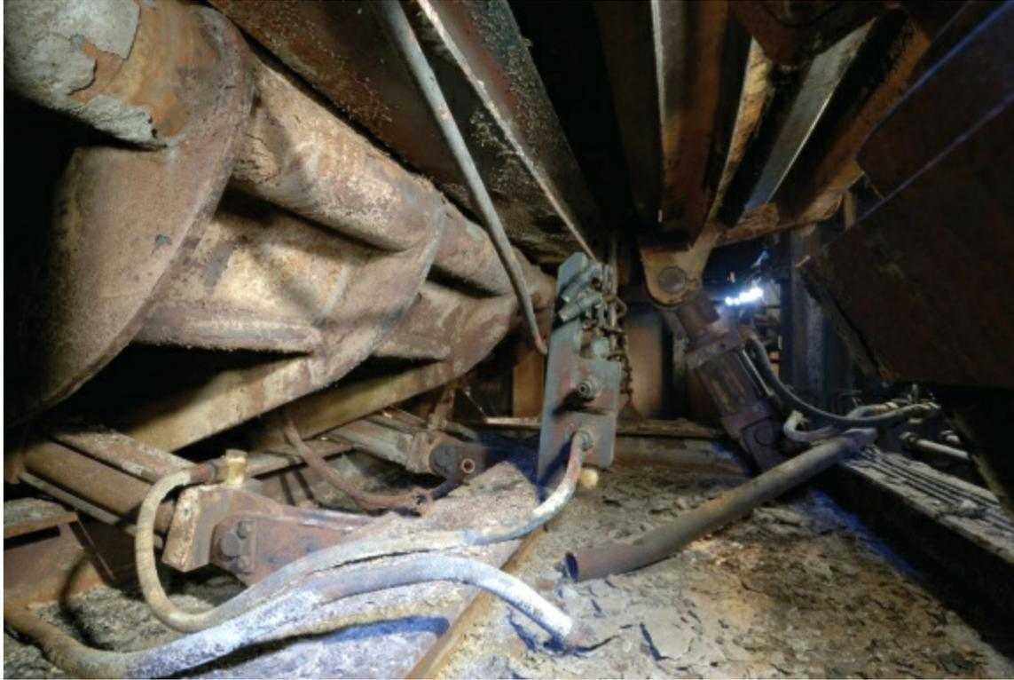
[Figure 7.1.3](#) Details of the hydraulic pipe that provoked the flash fire.
