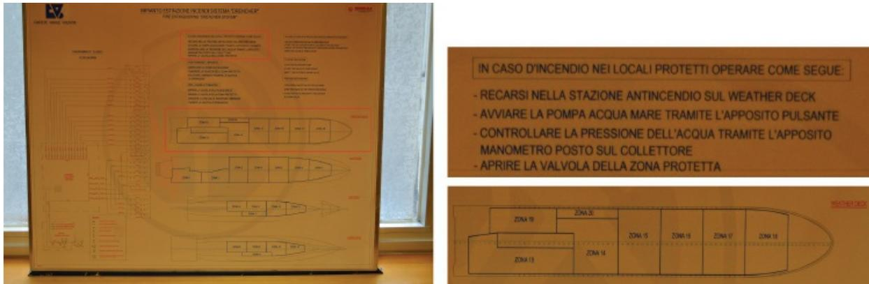
[Figure 7.2.5](#) Left. The drencher plan located in the drencher room. Right. Details of the instruction on the plan.
