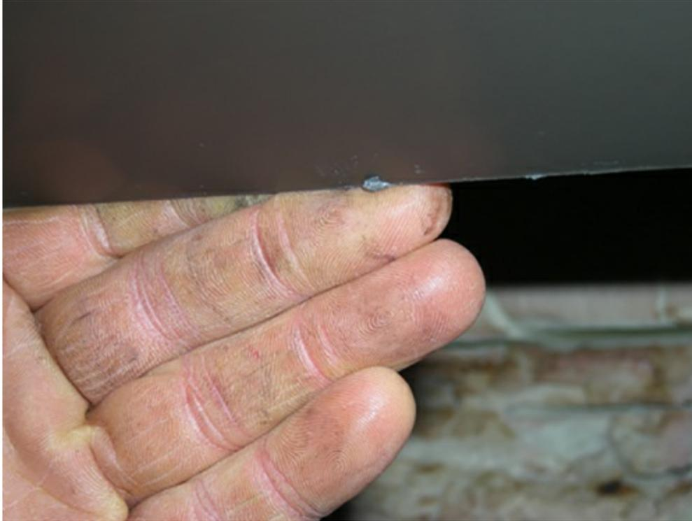
[Figure 4.11](#) Detail of a small imperfection on the edge of a metal sheet, ThyssenKrupp investigation
