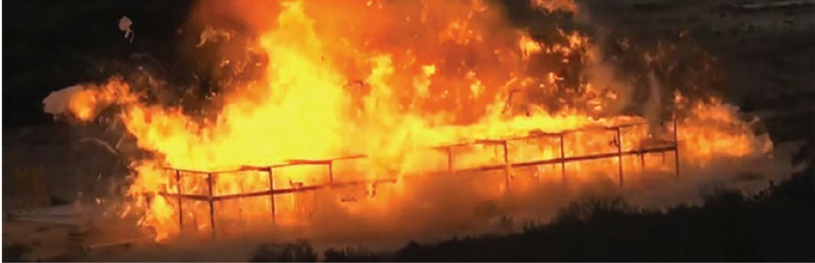
Figure 2.19 A Vapor Cloud Explosion test.
