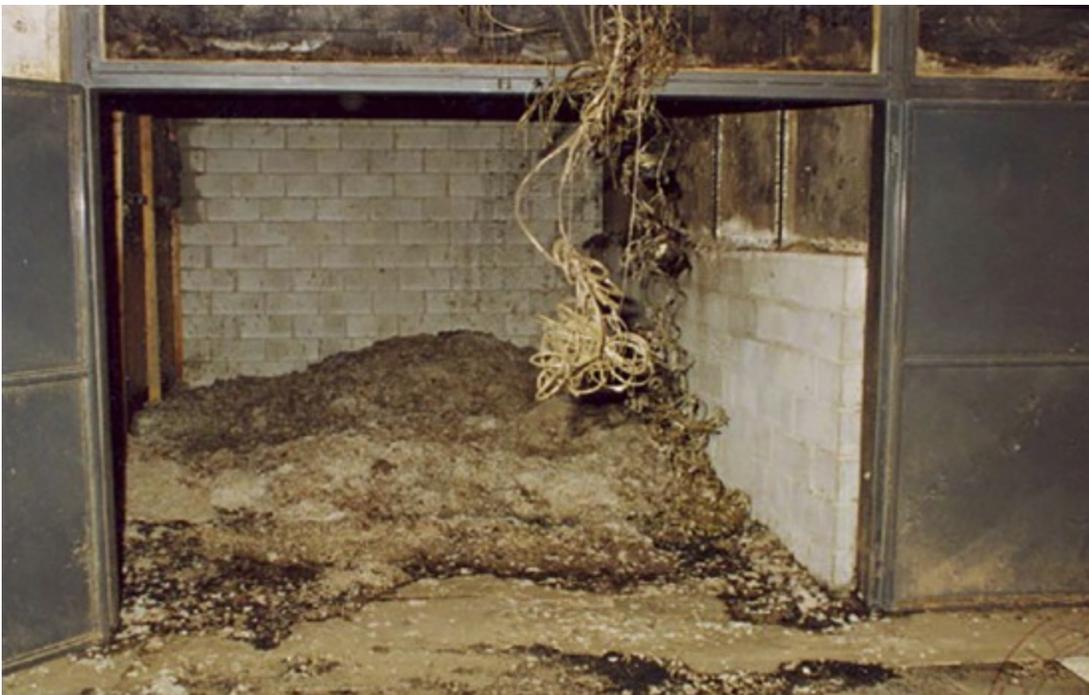
[Figure 4.22](#) Explosion of wool burrs, burrs storage boxes.
