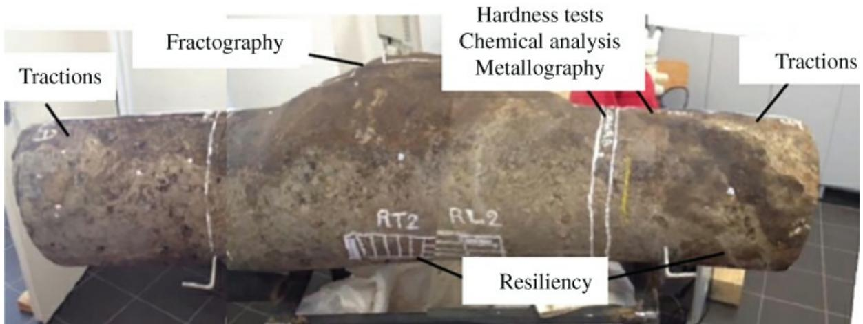
[Figure 7.9.5](#) Pipeline portions destined to mechanical tests and chemical analysis.
