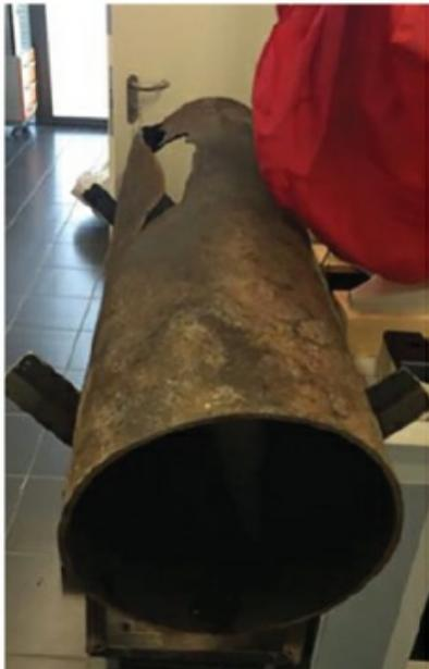
[Figure 7.9.4](#) The segment affected by fracture after sampling and details of external corrosion, related to the age of the pipe.
