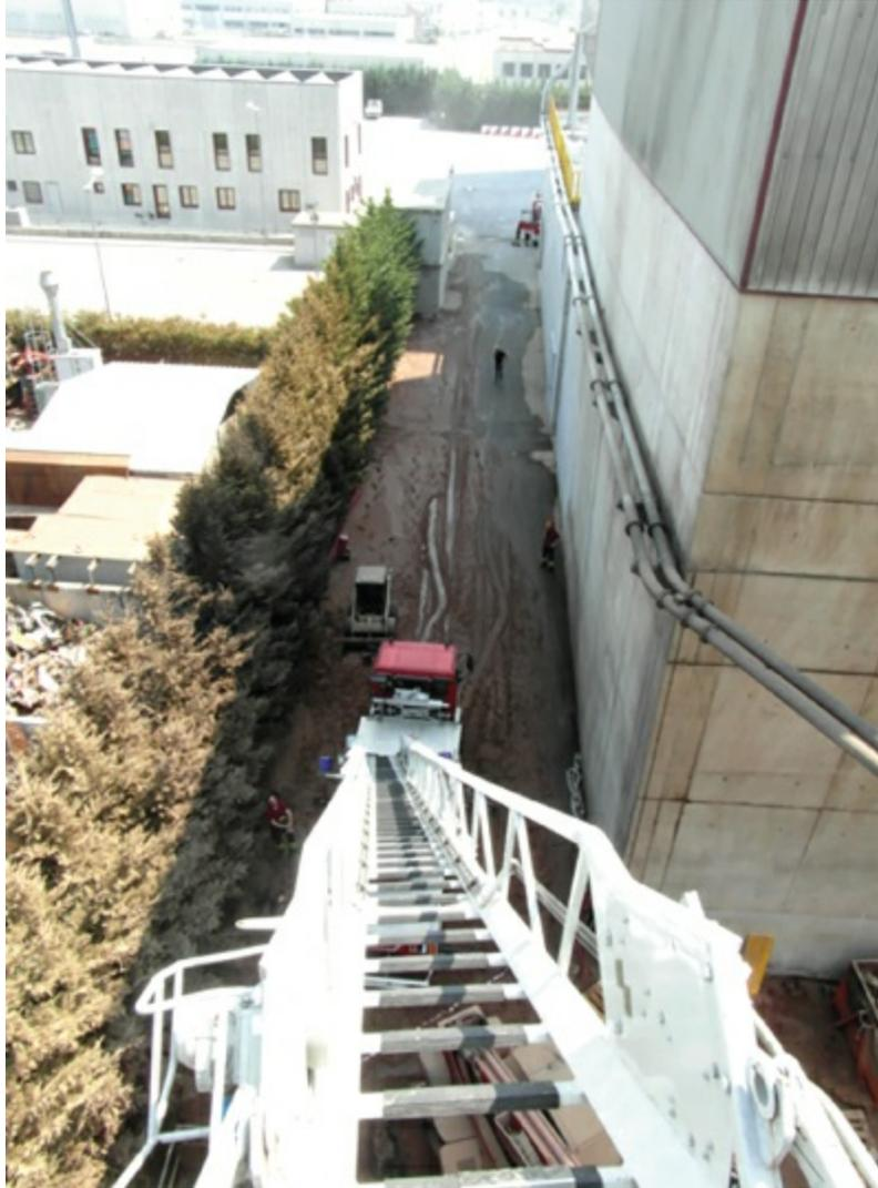
[Figure 7.5.6](#) The development of the flash fire could be deduced by the burned trees. The parked bobcat resulted in being ignited.
