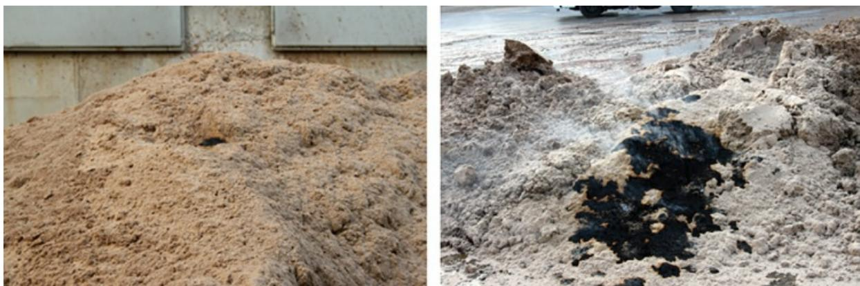
[Figure 7.5.4](#) The smoldering combustion in the saw dust discharged by the silo, in the occurrence of the event.
