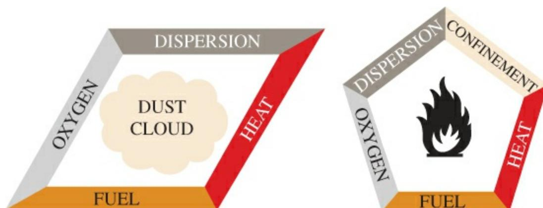
[Figure 7.5.8](#) Elements of a Flash Fire and the Explosion Pentagon.
