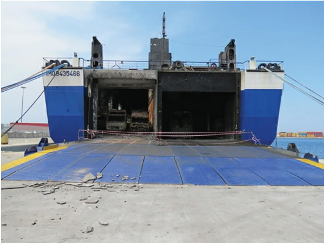
[Figure 2.10](#) Different colors at the access of deck 3 and 4 of the Norman Atlantic, suggesting two different typologies of fire. The oxygen-controlled fire at deck 3 (on the right) and fuel-controlled fire at deck 4 (on the left).
