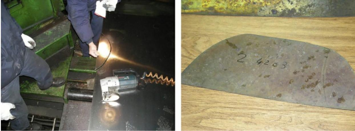
[Figure 4.4](#) Collection of some portions of metal sheet from the processing tape and their subsequent enumeration, ThyssenKrupp investigation.
