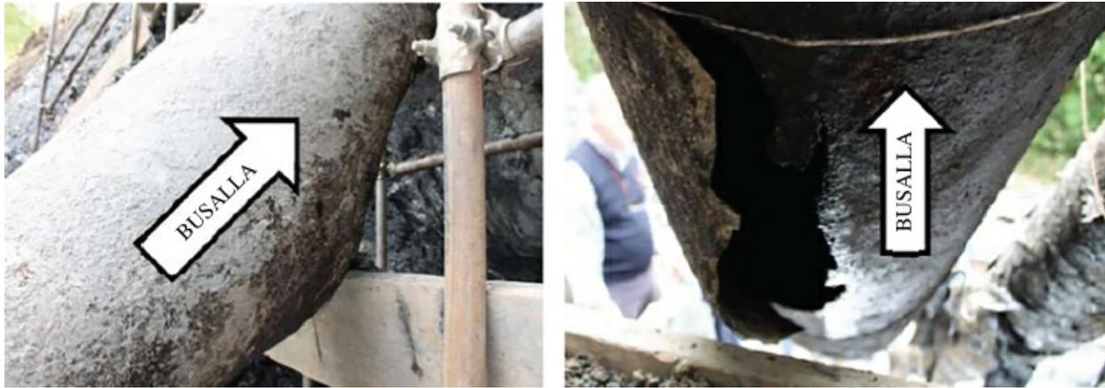
[Figure 7.9.3](#) Detail of the segment affected by fracture and fluid (oil and water, alternate) direction when the accident occurred.
