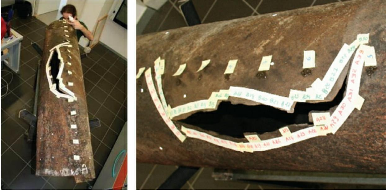
[Figure 7.9.6](#) Pipe segment in which the fracture along the longitudinal line “h 6” and the letter “A” identifying one of the two edges of the pipe (the other one is called “B”) are shown. Along the length of the fracture, different positions named from A1 to A33 are marked.
