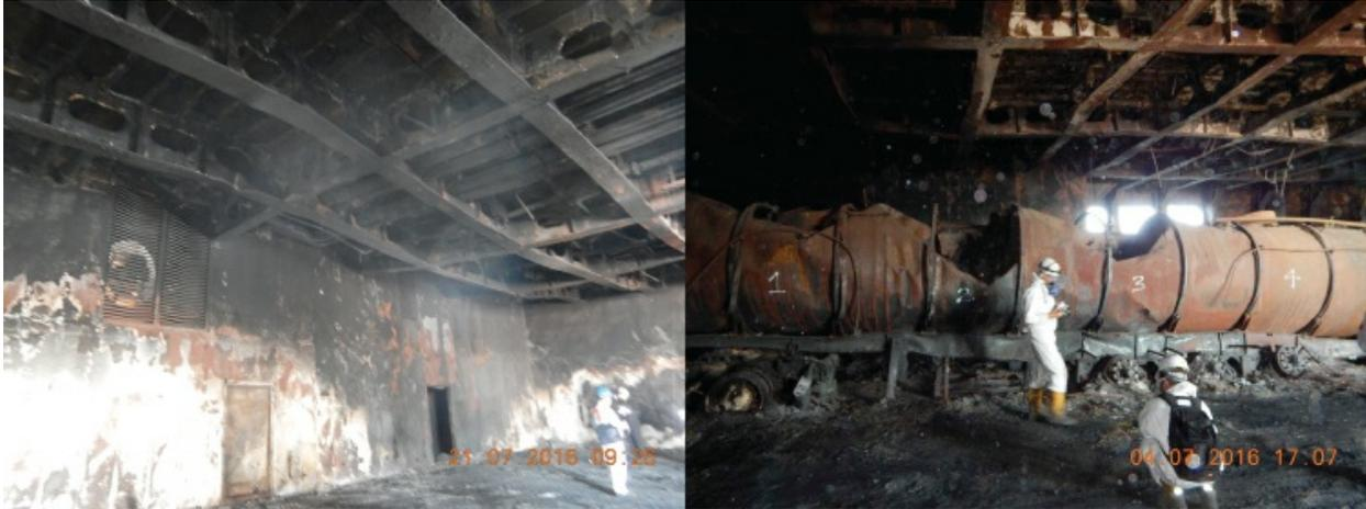
[Figure 7.2.7](#) Localised bending of transversal beams and V-shaped traces of smoke on the bulkhead. The majority of the fire load is attributable to the olive oil tanks.
