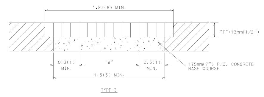
"T" = REPLACEMENT BRICK THICKNESS "W" = UTILITY TRENCH WIDTH
