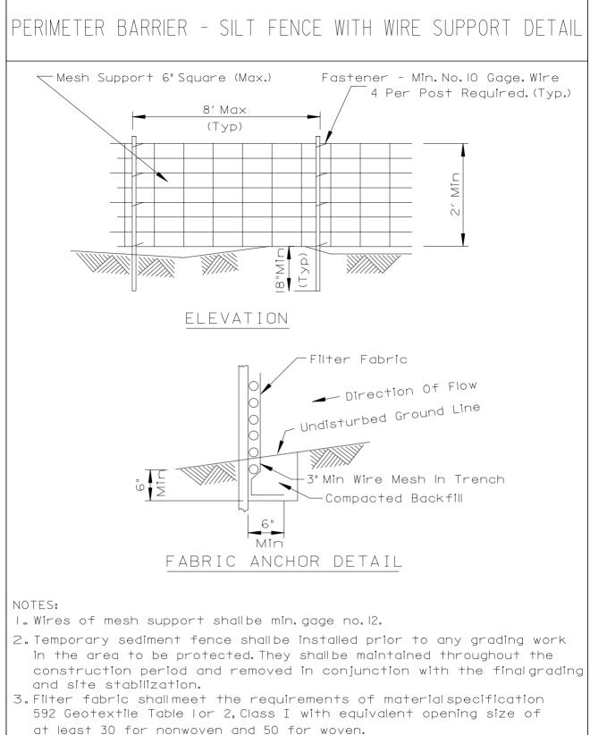
4. Fence posts shallbe either standard steelpost or wood post with a minimum cross-sectionalarea of 3.0 sq.in.
