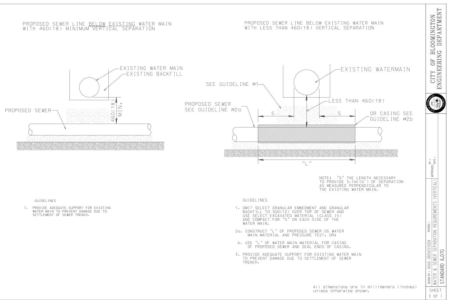
WHEN <u>PROPOSED</u> SEWER (OR WATER) IS LOCATED 3.1m(10') OR MORE FROM EXISTING WATER (OR SEWER), NO SPECIAL CONSTRUCTION IS REQUIRED
