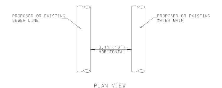
WHEN <u>proposed</u> sewer (or water) is located <u>less than 3.1m (10</u>')
