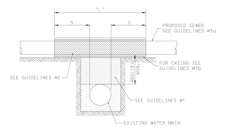
NOTE: "S" THE LENGTH NECESSARY TO PROVIDE 3.1m(10') of separation AS MEASURED PERPENDICULAR TO THE EXISTING WATER MAIN.
