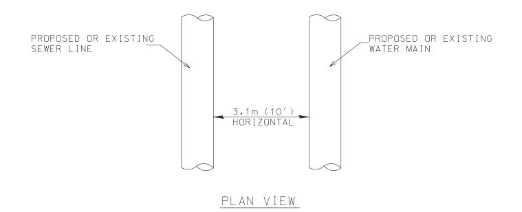
WHEN <u>PROPOSED</u> SEWER (OR WATER) IS LOCATED <u>LESS THAN 3.1m (10')</u> FROM EXISTING WATER (OR SEWER), DETAILS BELOW SHALL APPLY.
