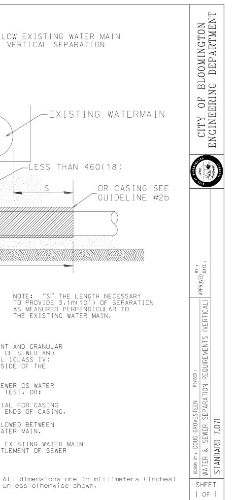
WHEN <u>PROPOSED</u> SEWER (OR WATER) IS LOCATED 3.1m(10') OR MORE FROM EXISTING WATER (OR SEWER), NO SPECIAL CONSTRUCTION IS REQUIRED
