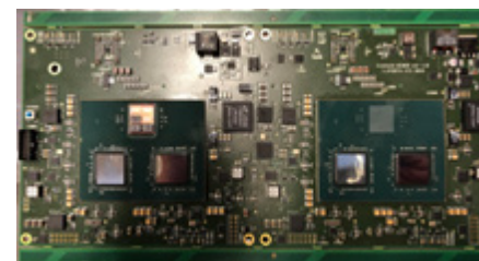
ExaNoDe prototype with Multi-Chip-Modules, 3D Integrated Circuit and FPGA bare dies
