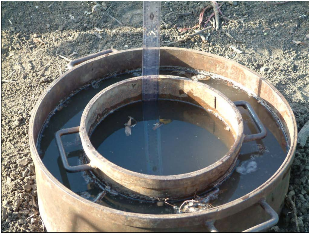
Photo 2 – Simple Double Ring Infiltrometer
