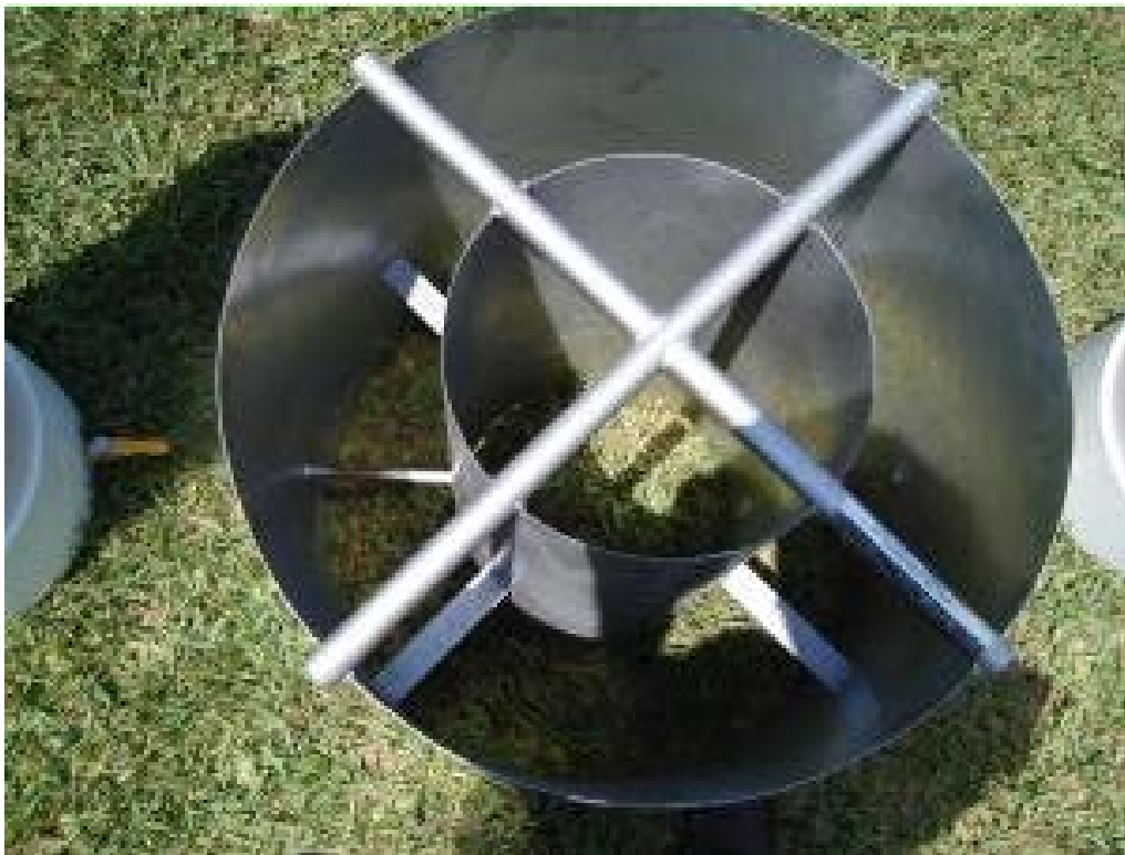
Photo 3 – Pre-fabricated Double Ring Infiltrometer (Photo courtesy of Turf-Tec International)
