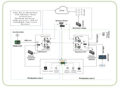
Figure 3: Multiple chain architecture
