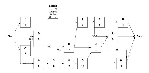
**Example Figure 2: Network with Smart Logic**
