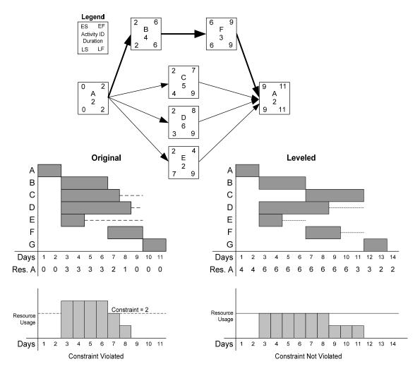
Figure 10: Resource leveling with constraints (project duration extended 2 days)
