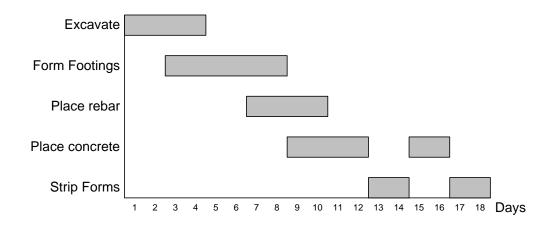
Figure 11: Example bar chart for placing a simple slab on a grade
