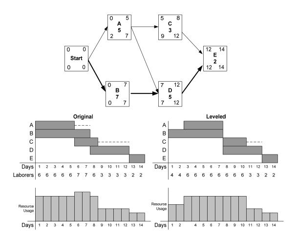
Figure 9: Resource leveling without constraints (within original project duration)
