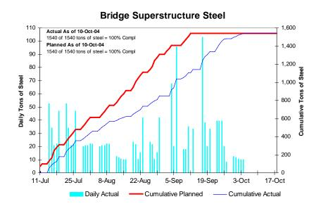
Figure 15: Superstructure Steel Commodity Curve
