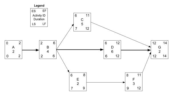
**Solution Figure 1: Network with Simple Logic**
