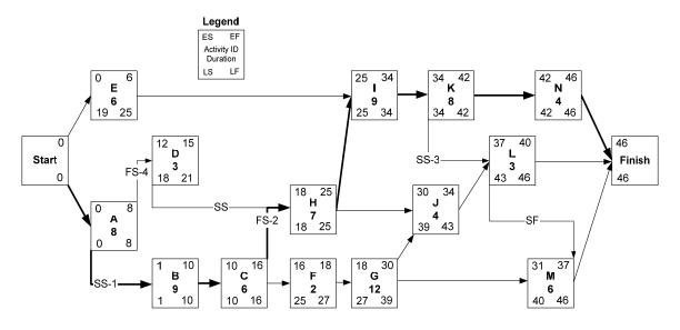
Solution Figure 2: Network with Smart Logic
