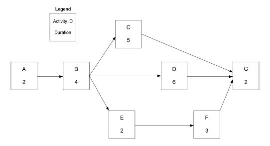
**Example Figure 1: Network with Simple Logic**
