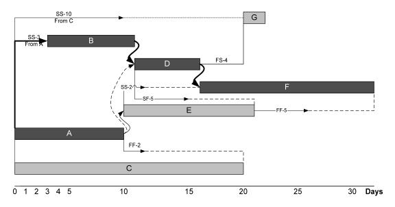
Figure 13: Time-scaled Logic Diagram
