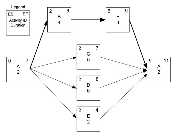
Figure 5: Basic Forward Pass Example
