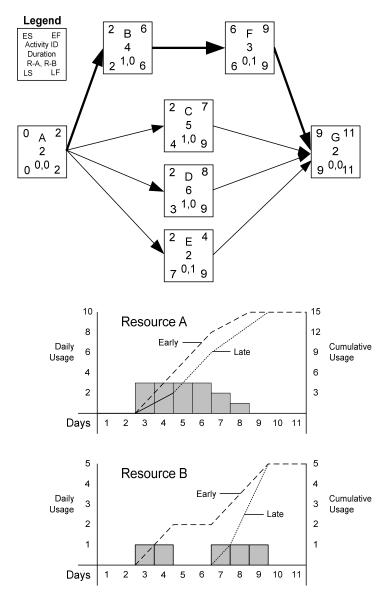
**Solution Figure 4: Multiple Resource Leveling Network**
