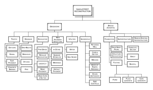
Figure 1: Example WBS for Tenth St. Reconstruction in Roanoke, VA
