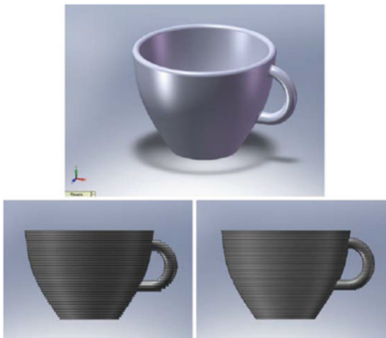
Fig. 1.1 CAD image of a teacup with further images showing the effects of building using different layer thicknesses
