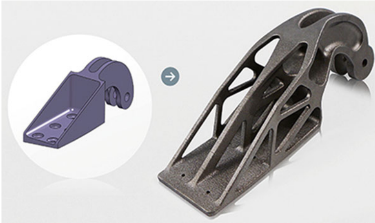
Fig. 19.9 A320 hinge bracket redesigned for AM. Courtesy EOS GmbH
