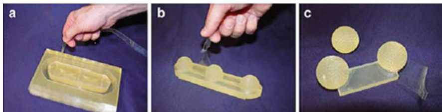
Fig. 9.2 Support material removal for three golf balls made using a Solidimension machine, showing: (a) the balls still encased in a central region, being separated from the larger block of bonded material; (b) the support material is glued in an accordion-like manner so that the excess material can be pulled out easily as a continuous piece; and (c) the balls after complete removal of excess support material (Courtesy 3D Systems)
