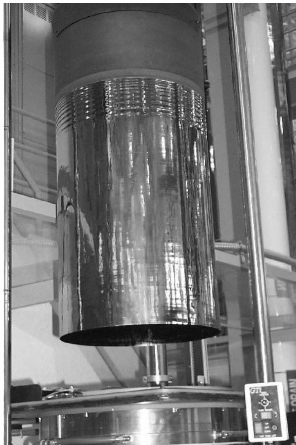
Figure 6.23 Experimental 50-cm-diameter EFG cylinder exiting from furnace
