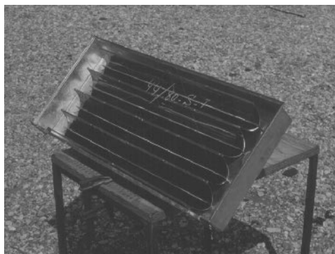
Figure 11.15 Static concentrator formed by an oil-filled CPC with bifacial cells
