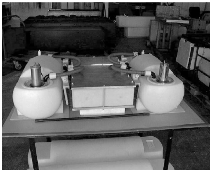
Figure 18.27 Prototype of a vanadium redox-flow battery with 32 cells and 14 Ah (Picture Courtesy by ZSW [29])
