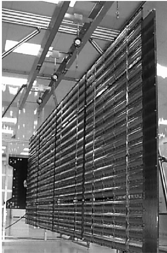
Figure 10.16 The SCARLET array used on Deep Space 1
