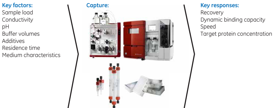
Fig 2.5. Initial purification of the target molecule from the source material is performed in the capture step, with the goals being rapid isolation, stabilization, and concentration of the target protein.
