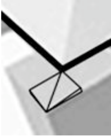
Folded plate splash block. Outer edges to extend beyond face of column.
