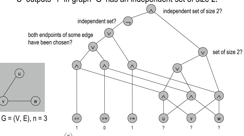
$\binom{n}{2}$  hard-coded inputs (graph description) n inputs (nodes in independent set)
