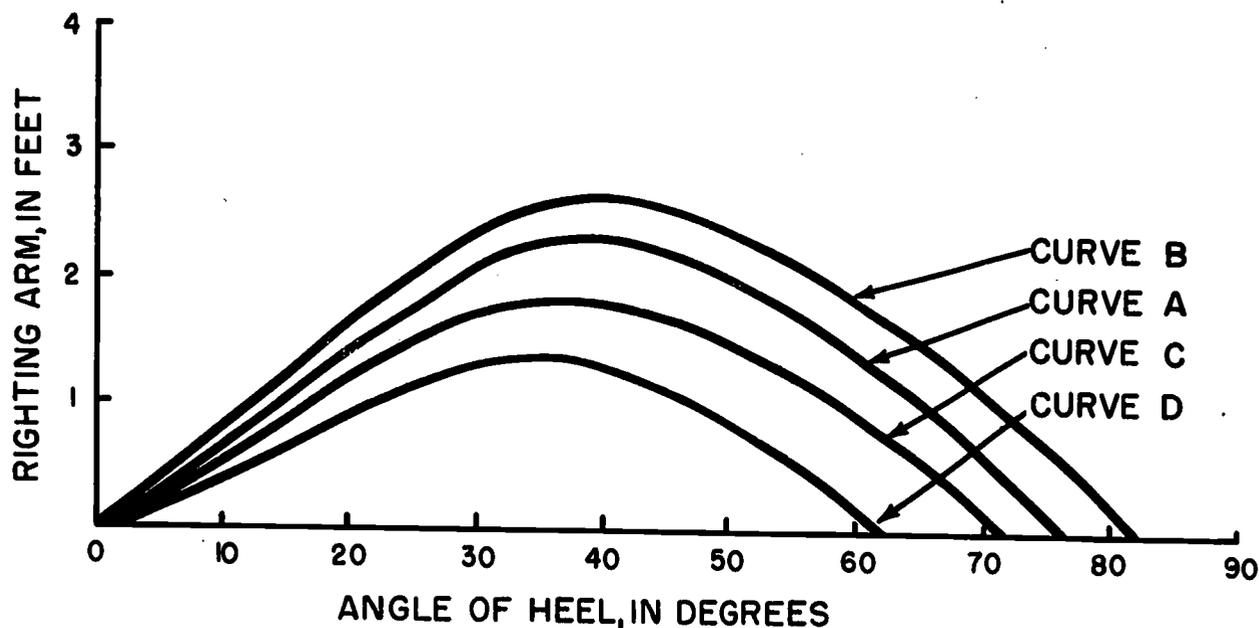
Figure 3-30.—Stability curve corrected for effects of added weight, free surface, and free communication.
