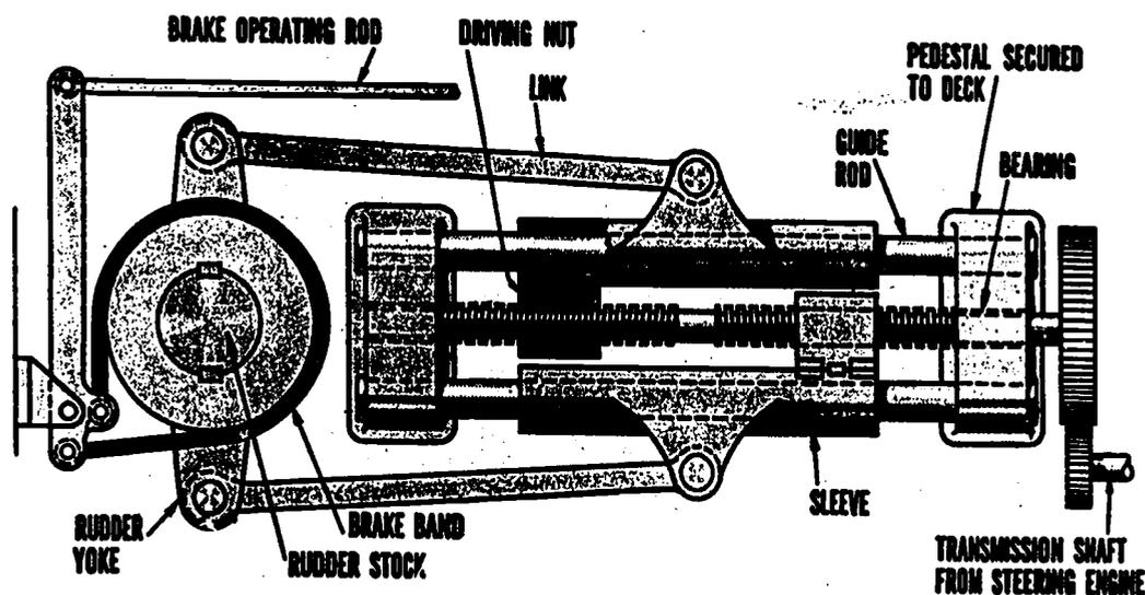
Figure 21-5.—Right-and-left screw steering gear.
