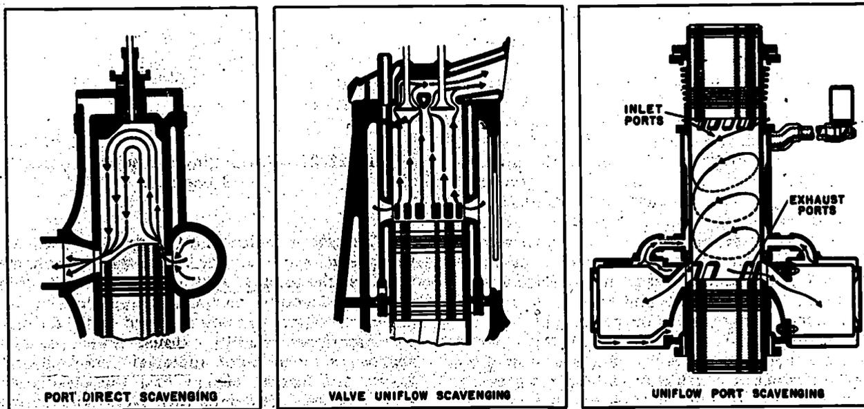
Figure 22-21.—Methods of scavenging—diesel engines.
