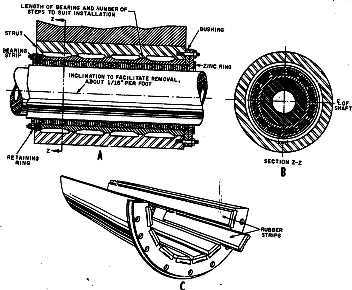
Figure 5-14.—Strut bearing. (A) Longitudinal cutaway view. (B) Cross-sectional view. (C) Arrangement of rubber stripping in the bearing bushing. 47.41
