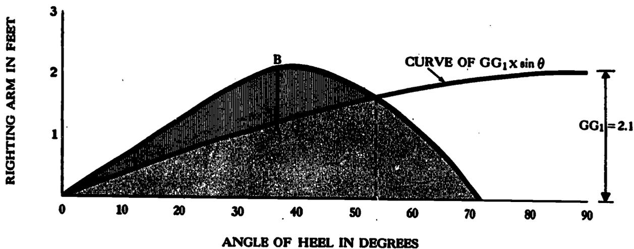
Figure 3-20.—Sine curve superimposed on original stability curve.
