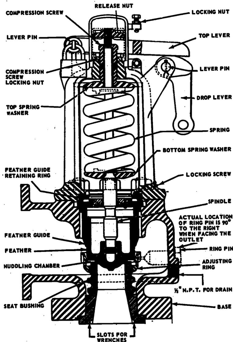
Figure 11-18.—Steam drum safety valve (huddling chamber type).
