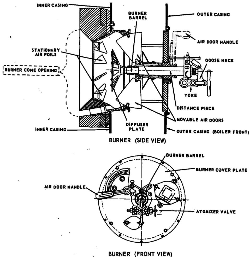
Figure 10-10.—Cross-sectional view of fuel oil burner with straight-through-flow atomizer. 38.69
