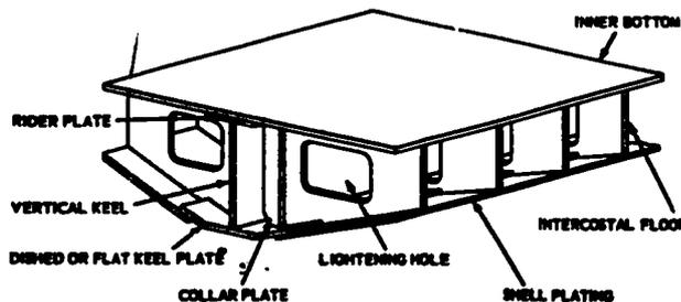
Figure 2-7.—One type of keel structure.
