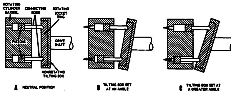
Figure 15-12.—Diagram showing how tilting box position affects position of pistons. 147.111
