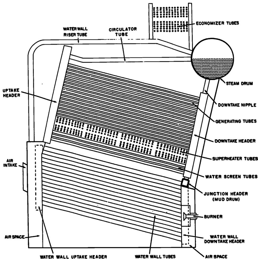
Figure 10-16.—Side view of header-type boiler.
