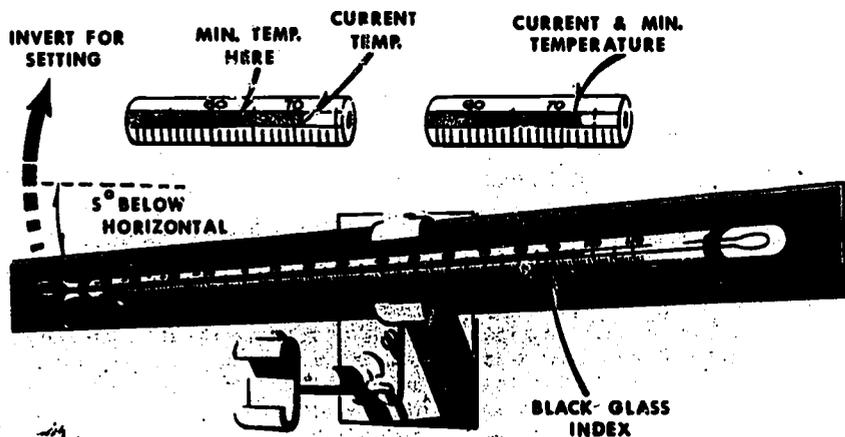
Figure 7-5.—Minimum indicating thermometer.
