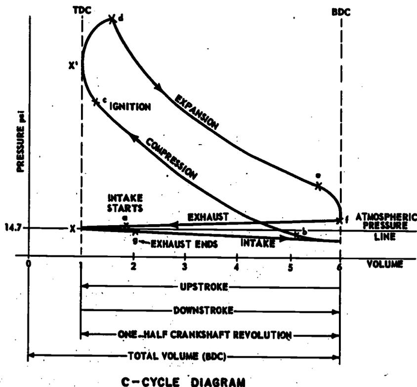
Figure 22-6.—Pressure-volume diagram, Otto 4-stroke cycle.
