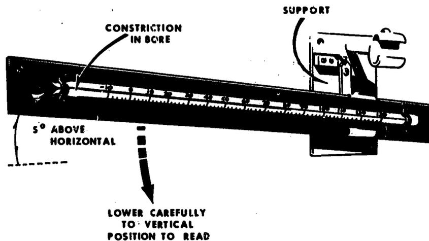
Figure 7-4.—Maximum indicating thermometer.
