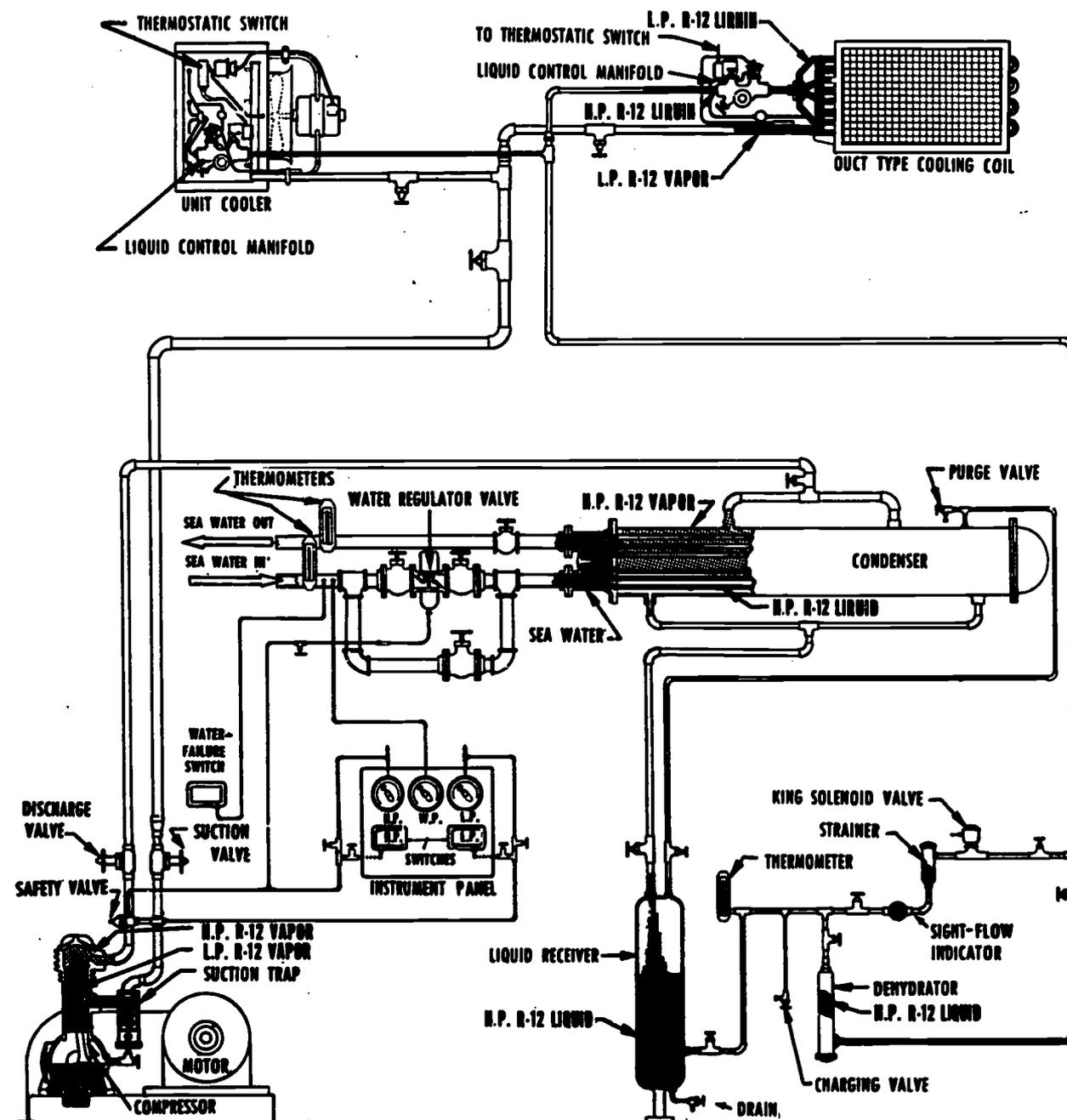
Figure 19-15.—Refrigerant circulating type of mechanical cooling system.
