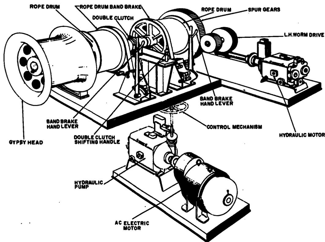
Figure 21-9.—Typical electrohydraulic winch.
