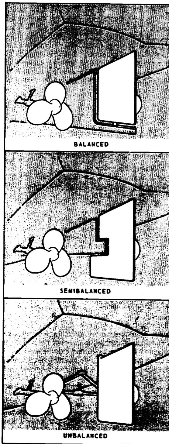
Figure 5-25.—Balanced, semibalanced, and unbalanced rudders.
