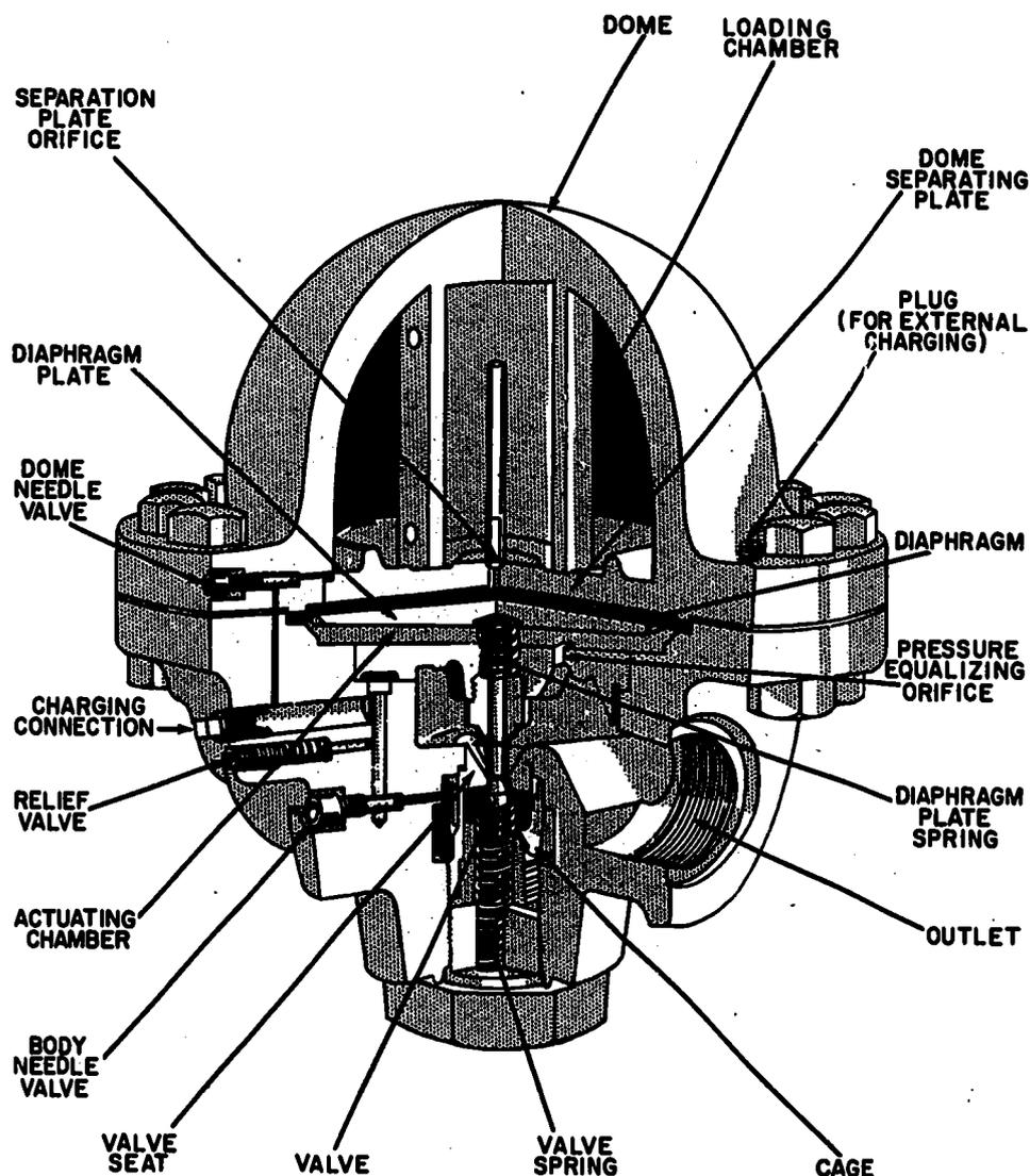
Figure 14-21.—Pneumatic pressure controlled reducing valve for low temperature service 47.60
