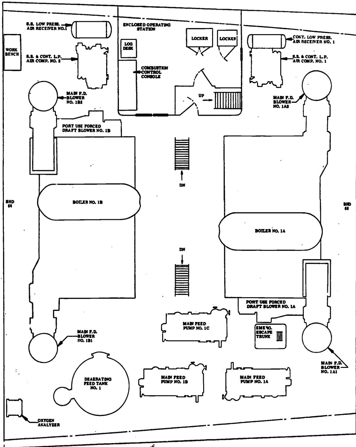
Figure 9-3.—Arrangement of machinery on upper level of No. 1 fireroom, DLG 14 and DLG 15.
