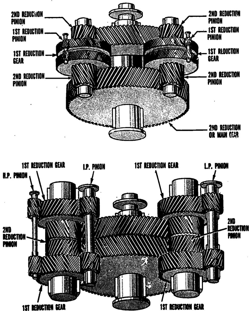
Figure 5-20.—Nested reduction gearing.
