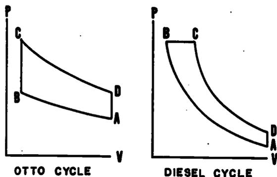
Figure 22-5.—Pressure-volume diagrams for theoretical combustion cycles.
