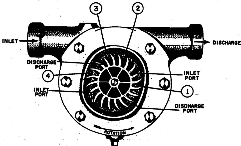
Figure 17-11.—Rotary-centrifugal compressor.
