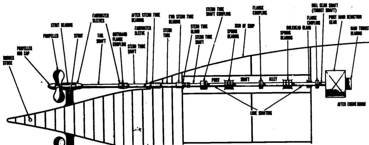
Figure 5-15.—Propulsion shafting, twin-screw ship.
