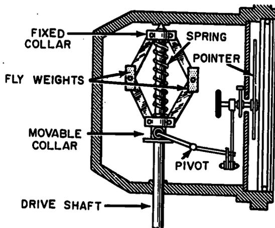
Figure 7-33.—Main parts of centrifugal tachometer. 2.66X
