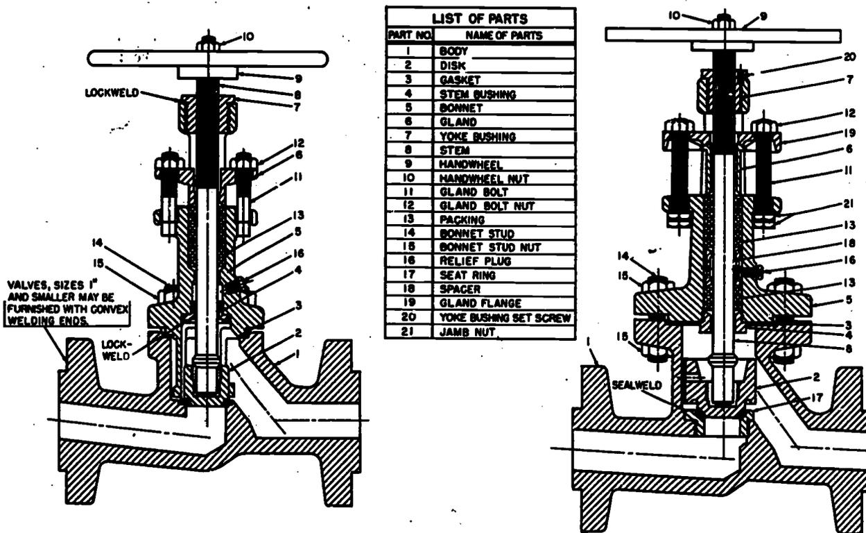
Figure 14-19.—Stop-check valves.
