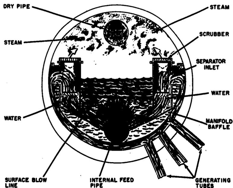
Figure 11-3.—Flow of steam and water in steam drum of double-furnace boiler.
