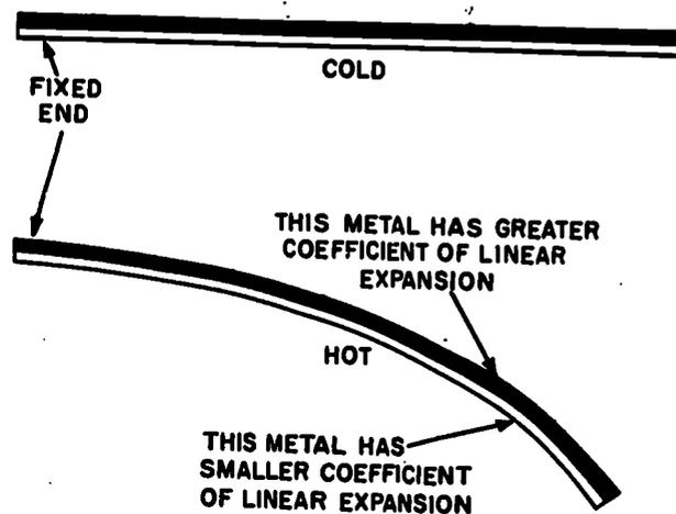
Figure 7-6.—Effect of unequal expansion of bimetallic strip. 147.53
