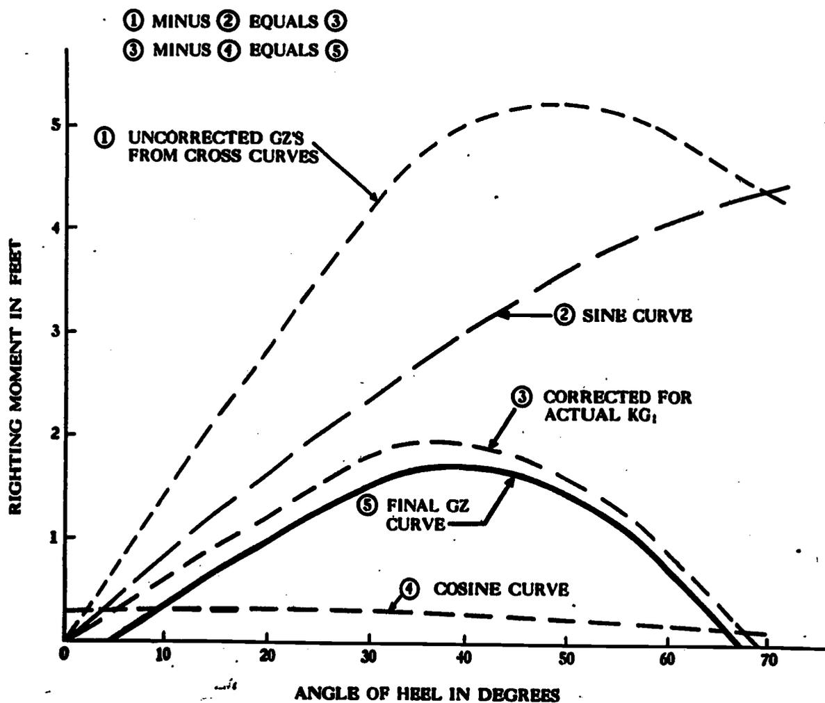
Figure 3-26.—Curve of righting arms corrected for weight addition.
