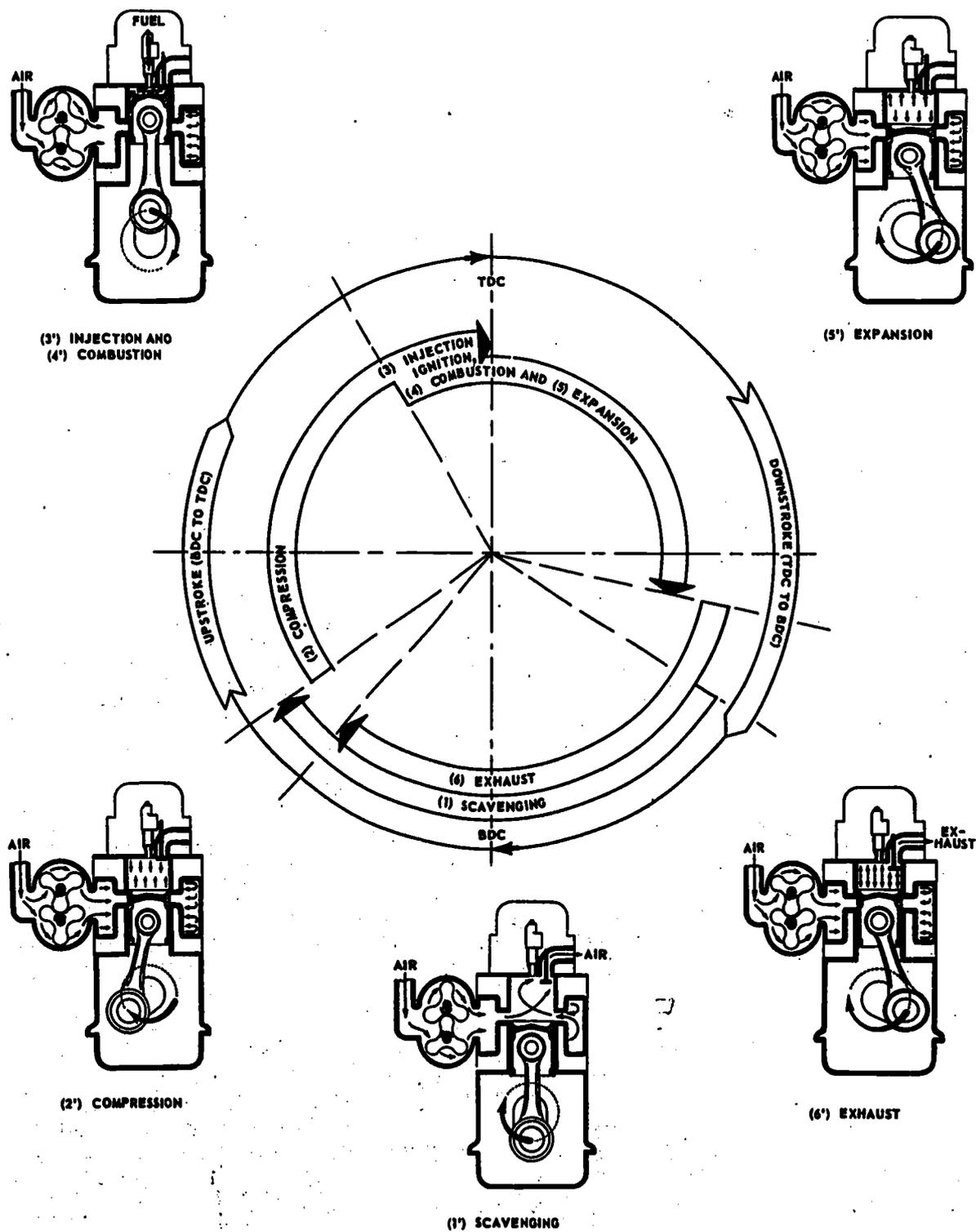
Figure 22-2.—Strokes and events of a 2-stroke cycle diesel engine.
