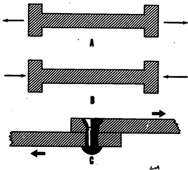
Figure 2-2.—Stresses in metal: (A) tension; (B) compression; (C) shear.
