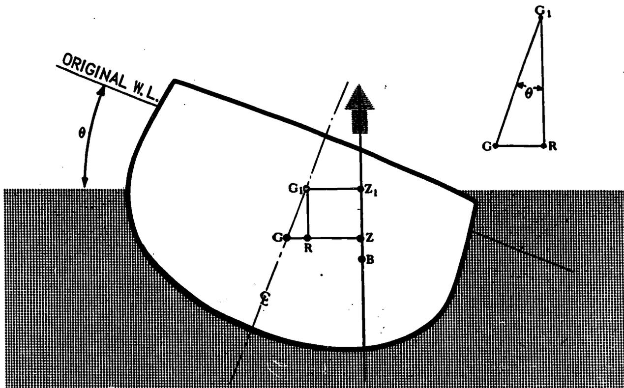
Figure 3-18.—Loss of righting arm due to rise in center of gravity.
