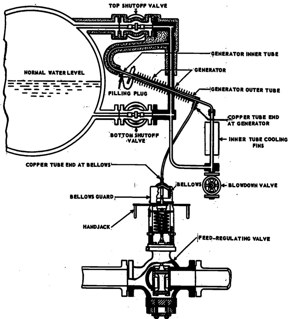
Figure 11-37.—Single-element feed water regulator.
