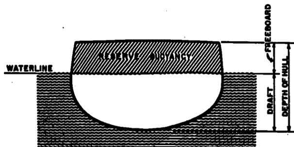
Figure 3-7.—Reserve buoyancy, freeboard, draft, and depth of hull. 8.47
