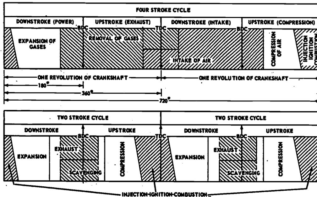
Figure 22-3.—Comparison of the 2- and 4-stroke cycles.
