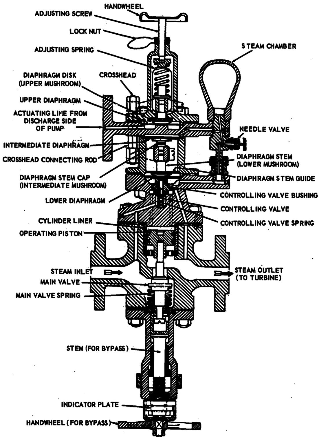
Figure 16-10.—Constant-pressure pump governor for main feed pump.
