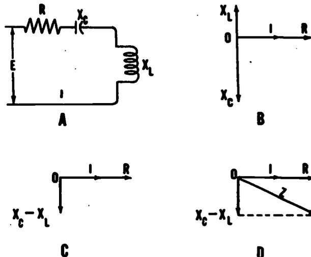
Figure 20-18.—Vector solution of an a-c circuit.
