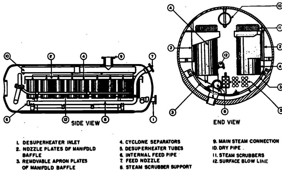
Figure 11-6.—Arrangement of internal fittings in older single-furnace boiler.
