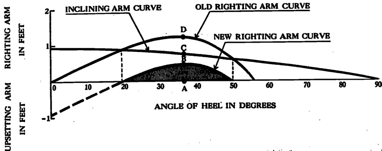
Figure 3-24.—New curve of static stability after correction for horizontal weight movement. 147.40
