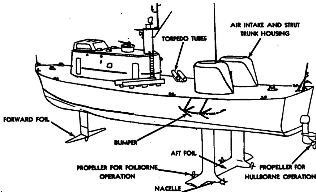
Figure 25-1.—Hydrofoil (USS High Point, PCH 1)
