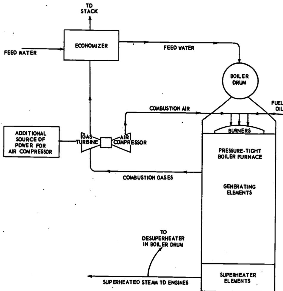
Figure 10-25.—Schematic view of pressurized-furnace boiler.
