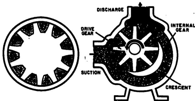
Figure 15-24.—Internal gear pump. 147.117
