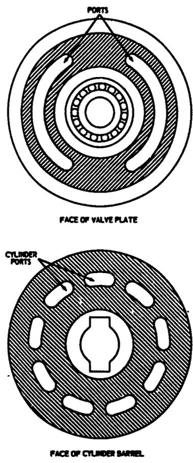
Figure 15-13.—Suction and discharge ports in face of cylinder barrel and in valve plate. 147.112
