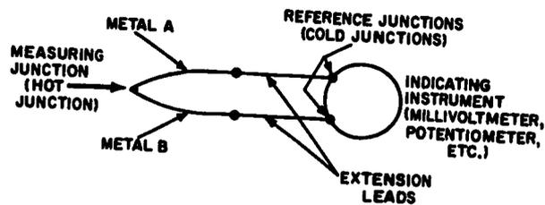
Figure 7-10.—Simple thermocouple. 147.55
