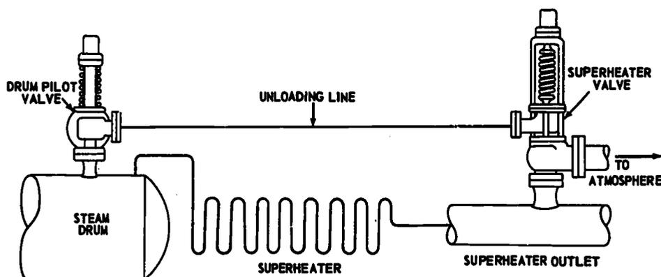
Figure 11-21.—Crosby two-valve superheater outlet safety valve assembly.
