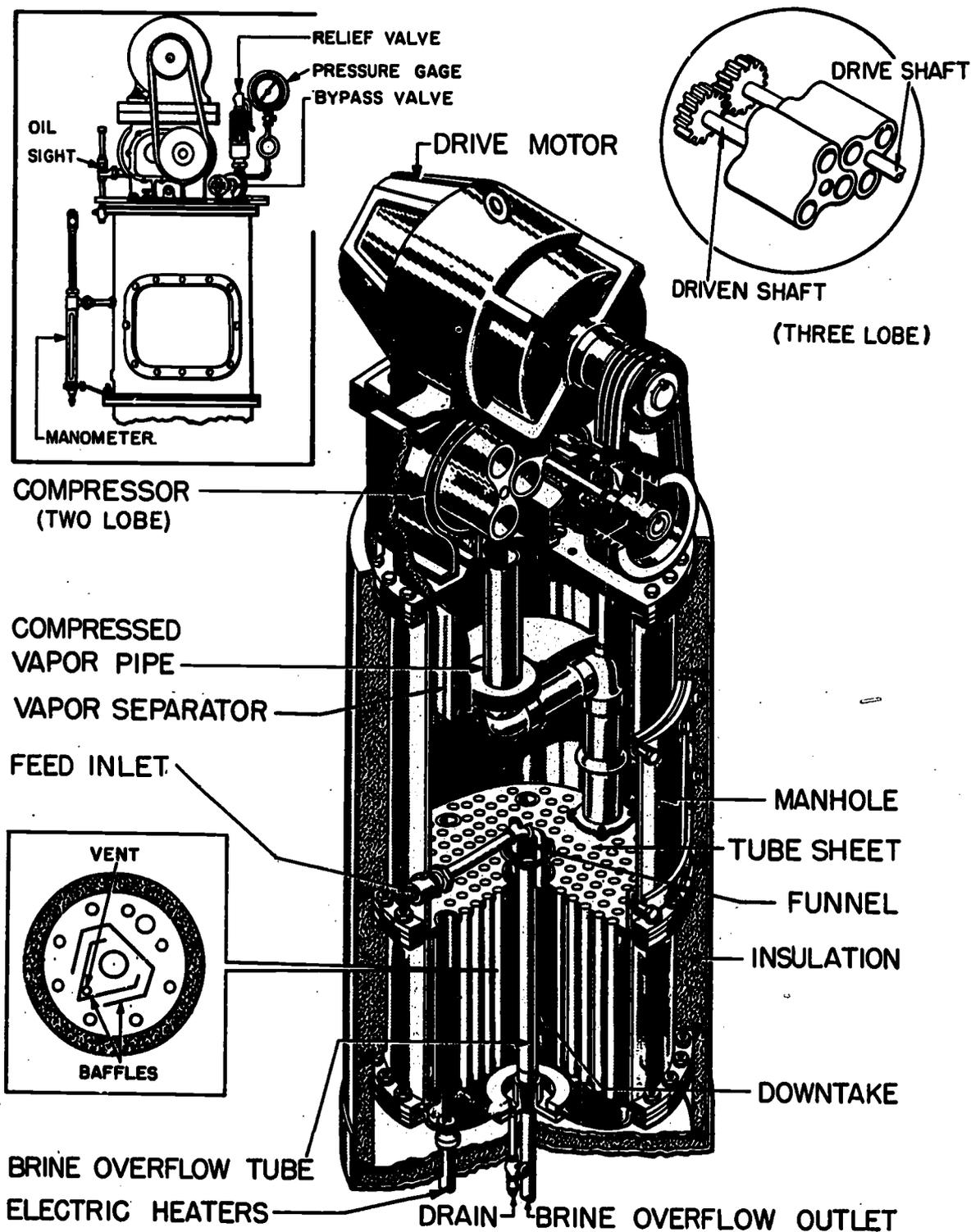
Figure 18-2.—Cutaway view of vapor compression distilling plant.
