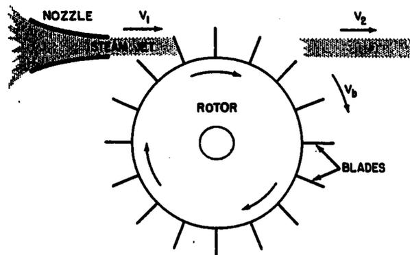
Figure 12-3.—Elementary impulse turbine. 147.92
