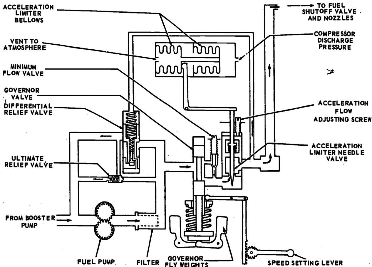
Figure 23-17.—Schematic diagram of fuel control assembly.
