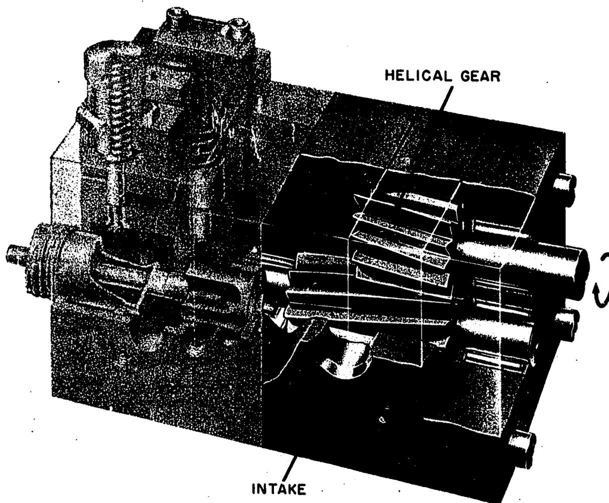
Figure 15-17.—Helical gear pump.
