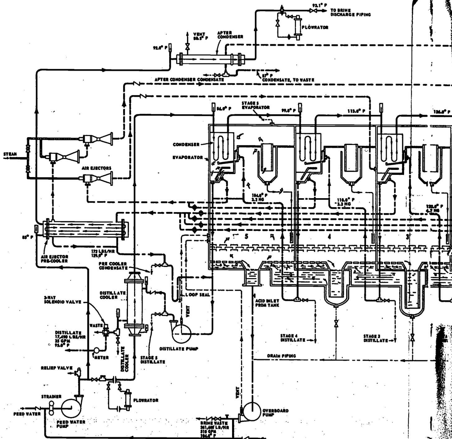
Figure 18-10.—General arrangement of five-stage flash-type distilling plant.
