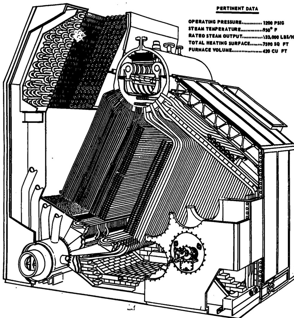
Figure 10-22.—Newer 1200-psi single-furnace boiler for post World War II destroyer.
