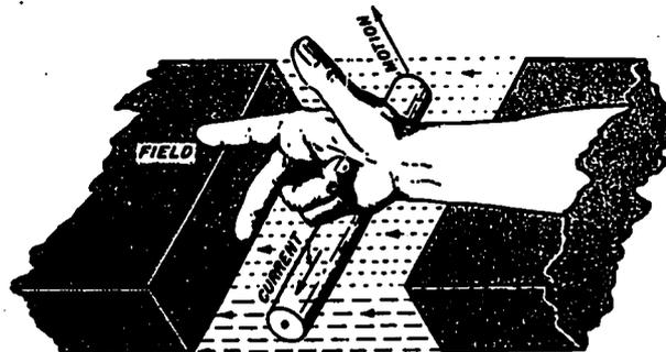
Figure 20-16.—Right-hand motor rule for electron flow.
