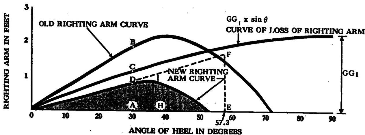
Figure 3-21.—Curve of static stability as corrected for loss of stability due to a vertical weight shift.
