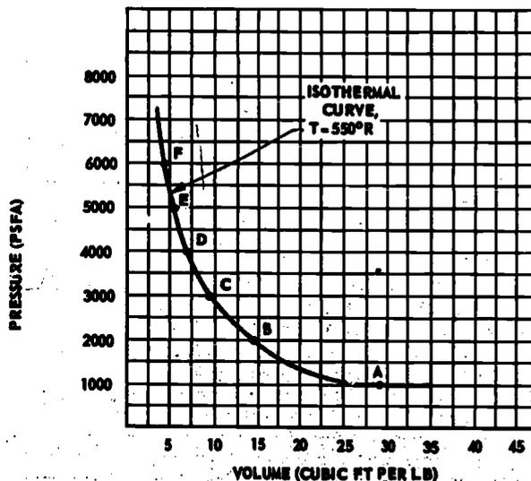
Figure 8-14.—Constant temperature (isothermal) line on p-v diagram.
