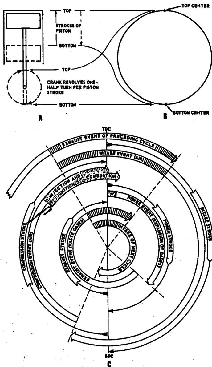
Figure 22-1.—Relationship of events and strokes in a 4-stroke cycle diesel engine. 54.19A
