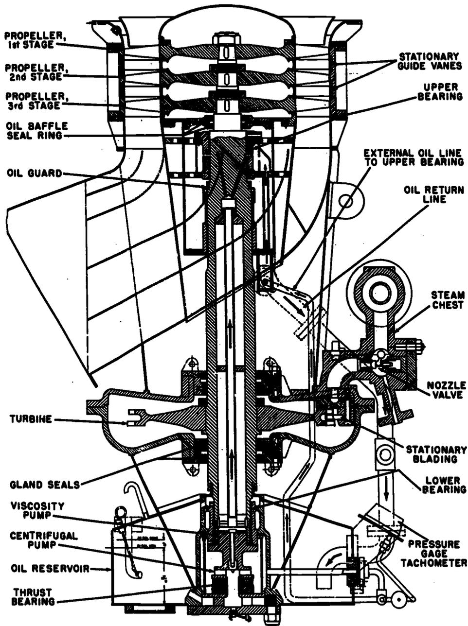
Figure 15-35.—Sectional view of three-stage vertical propeller-type blower.
