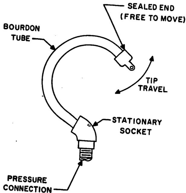
Figure 7-9.—C-shaped Bourdon tube. 38.211(147B)
