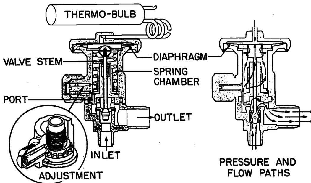
Figure 19-4.—Thermostatic expansion valve.
