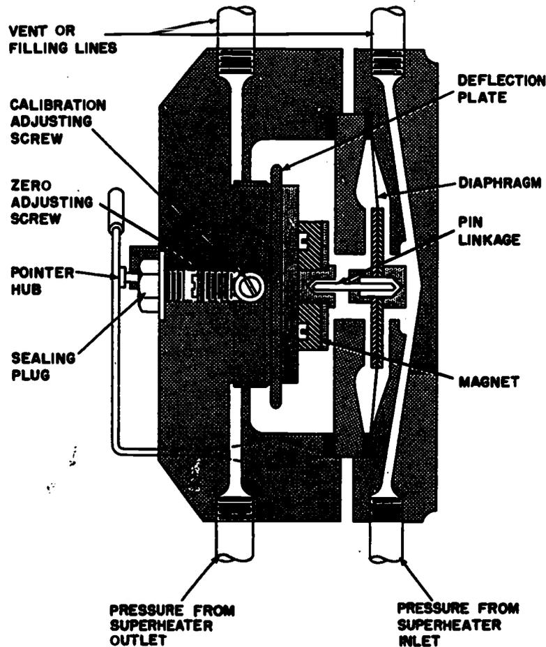
Figure 11-30.—Cross section of Yarway indicating unit (front view).
