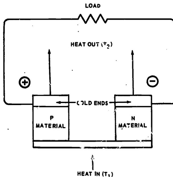
Figure 25-9.—Thermoelectric converter.
