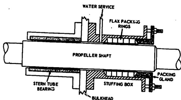
Figure 5-13.—Stern tube stuffing box and gland. 47.40
