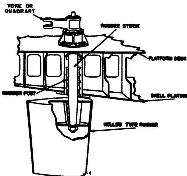
Figure 5-24.—Rudder assembly.
