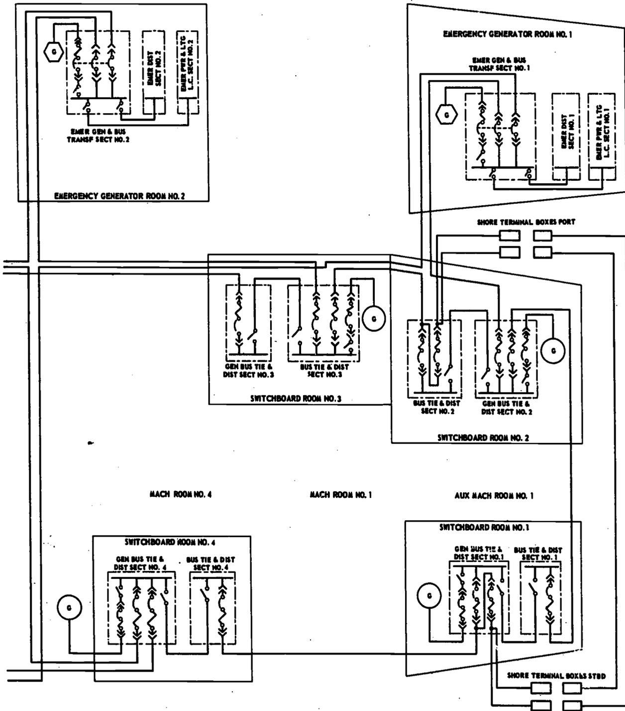
Figure 20-23.—Ship's service and emergency power distribution system in a large carrier.—Continued.
