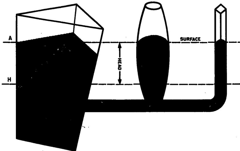
Figure 15-2.—Pressure in liquid is not affected by the shape of the vessel.
