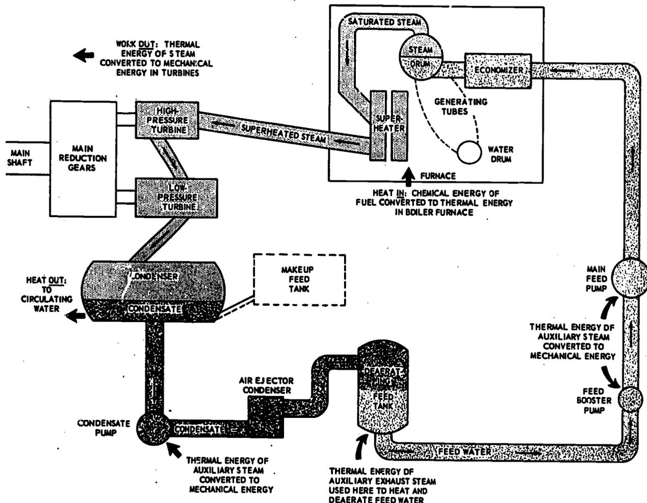
Figure 8-18.—Energy relationships in the basic propulsion cycle of conventional steam-driven ship. 38.2
