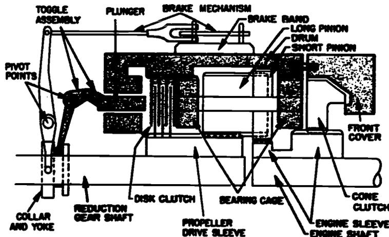
Figure 22-38.—Schematic diagram of Joe's reverse gear assembly.
