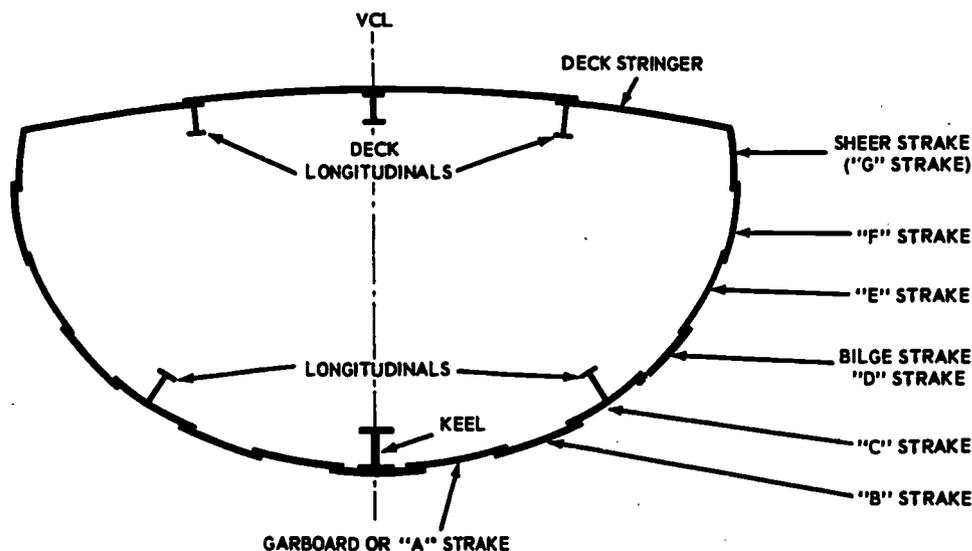
Figure 2-6.—Destroyer hull girder, showing some strength members.
