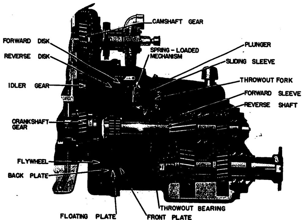
Figure 22-30.—Transmission with independent oil system.
