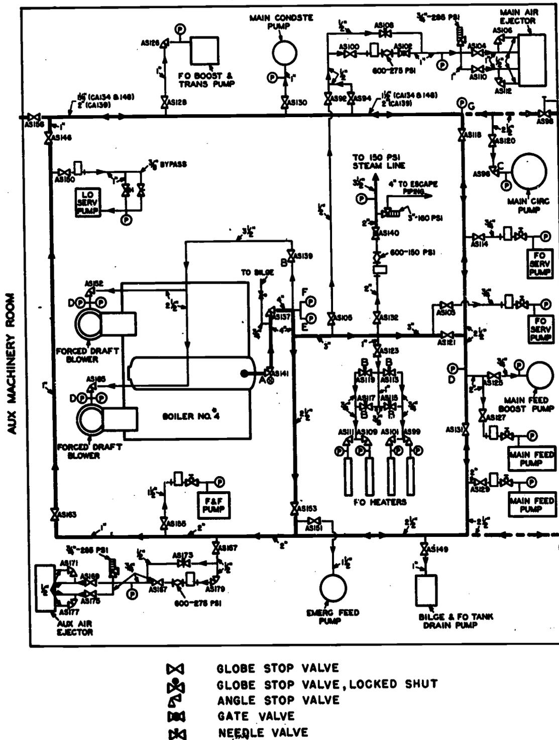
Figure 9-16.—Part of 600-psi auxiliary steam system, CA 139 class.
