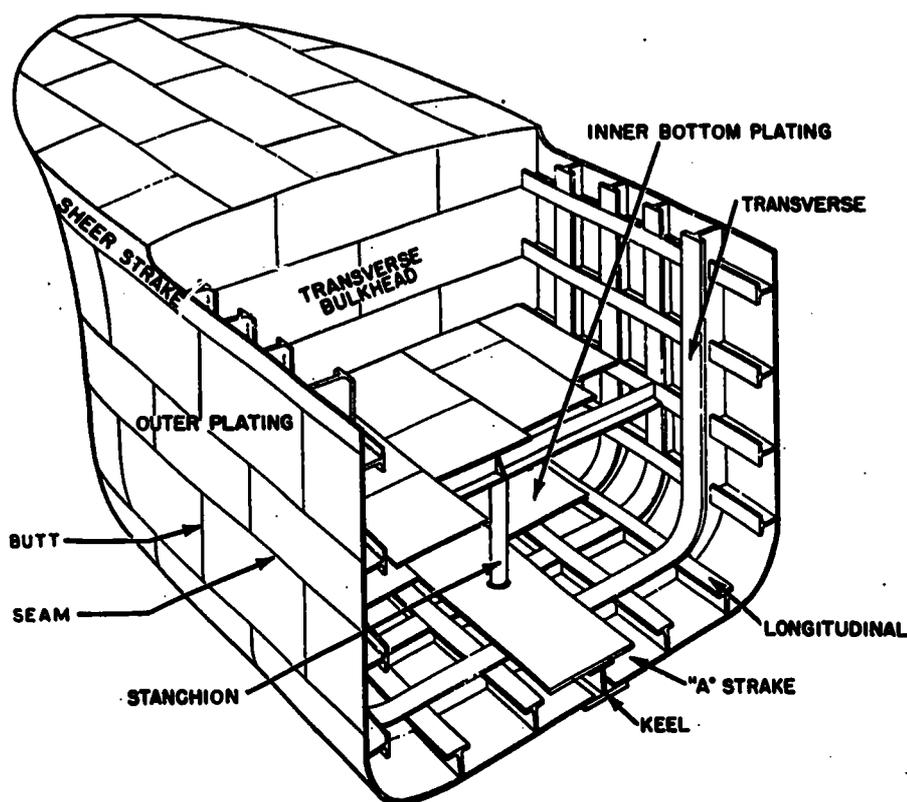
Figure 2-18.—Section of ship, showing plating and framing.
