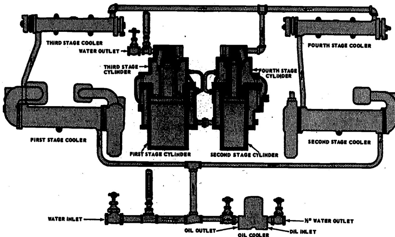
Figure 17-9.—Cooling water system for multistage air compressor.
