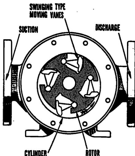
Figure 15-23.—Moving vane pump. 47.47
