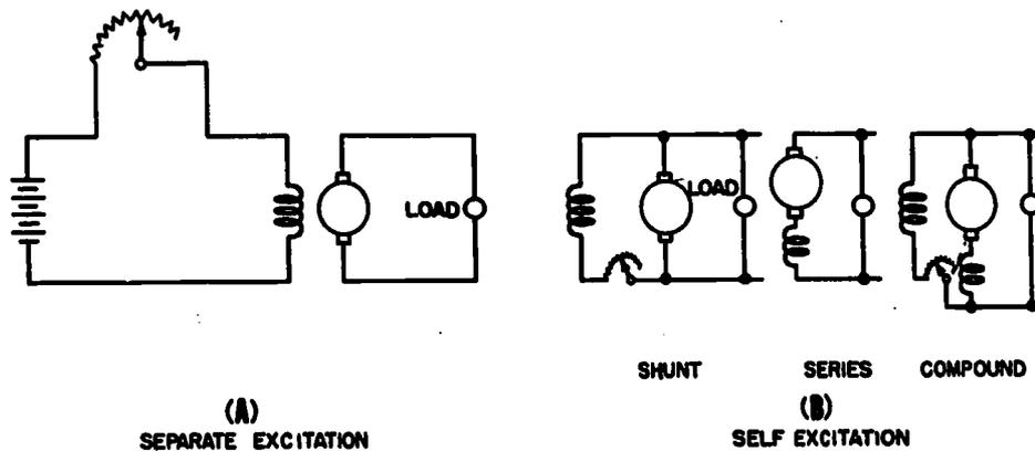
Figure 20-15.—Types of d-c generators.
