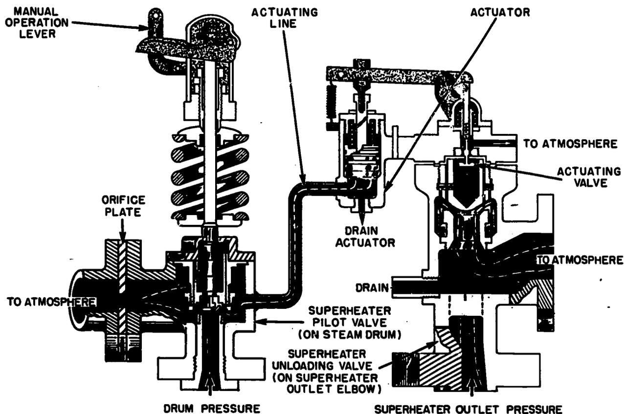
Figure 11-22.—Three-valve superheater outlet safety valve assembly (Consolidated). 104.22
