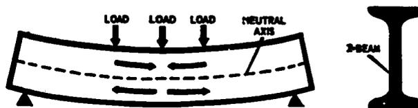
Figure 2-3.—I-beam with load placed over center.
