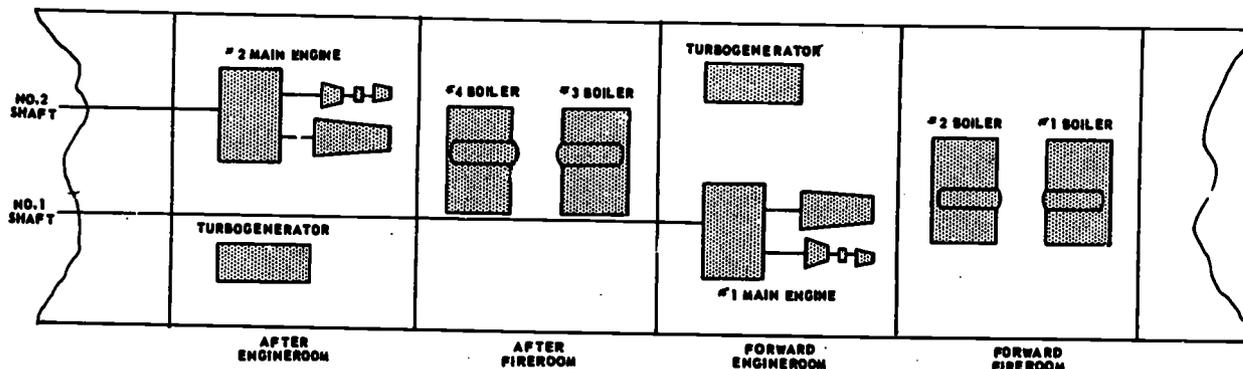
Figure 9-2.—Propulsion machinery arrangement, DD 445 and DD 692 classes.
