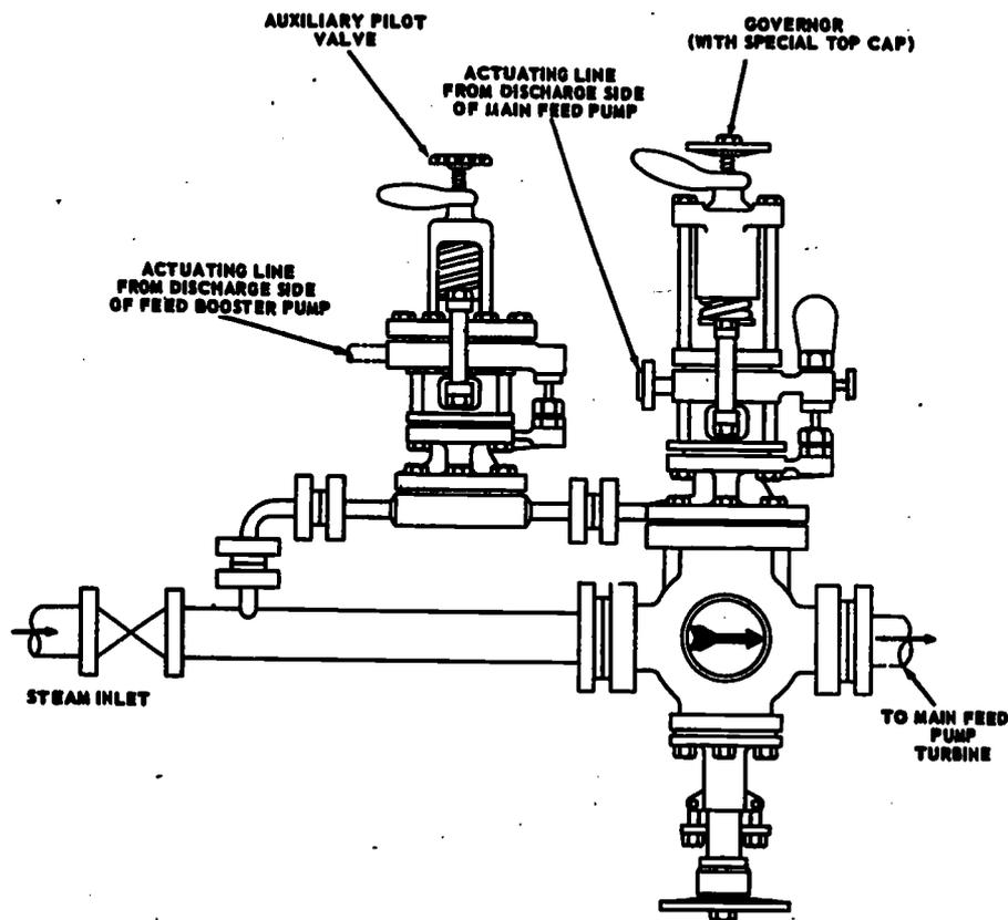
Figure 16-11.—Automatic shutdown device for main feed pump.
