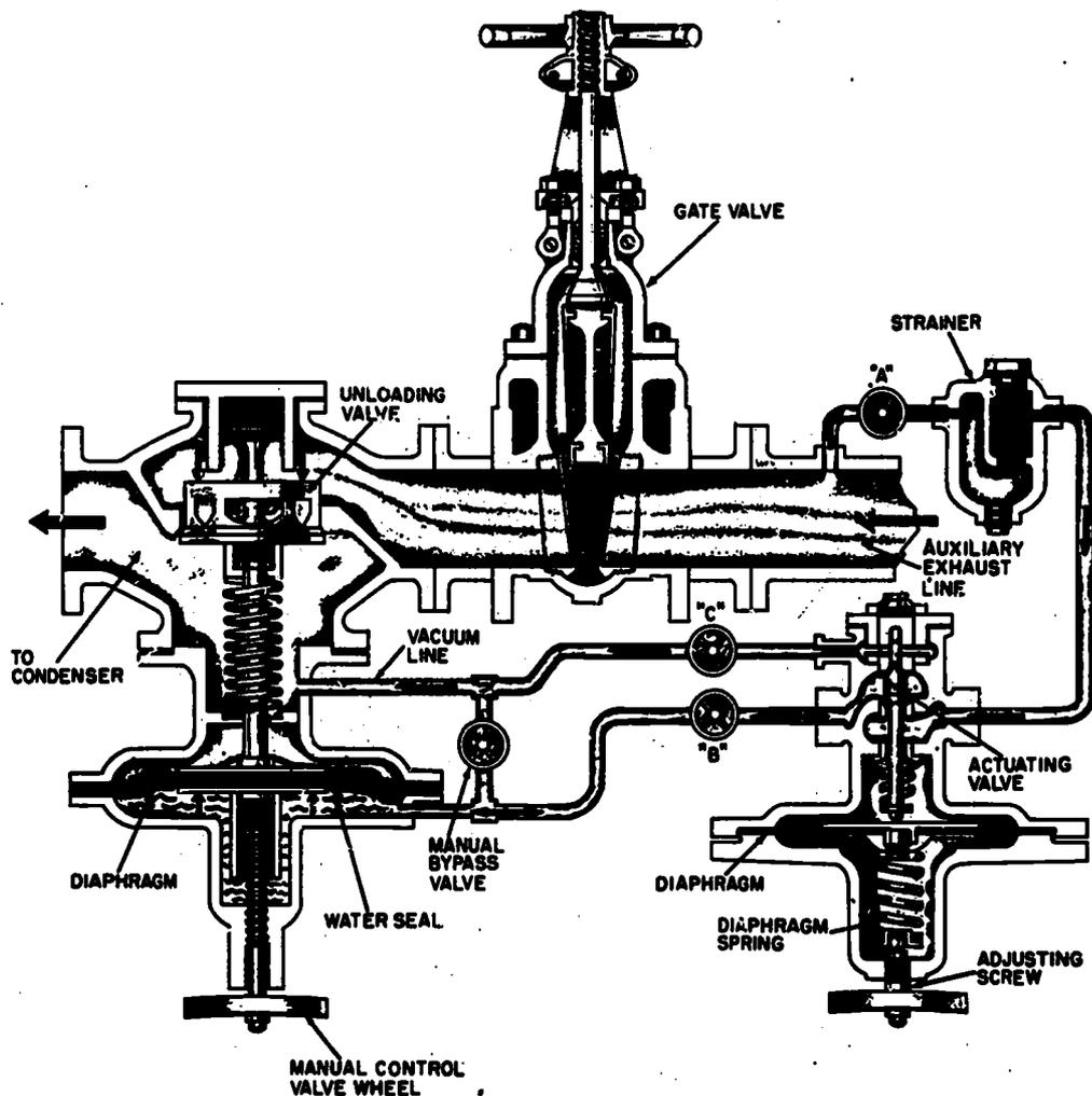
Figure 14-27.—Automatic unloading valve.
