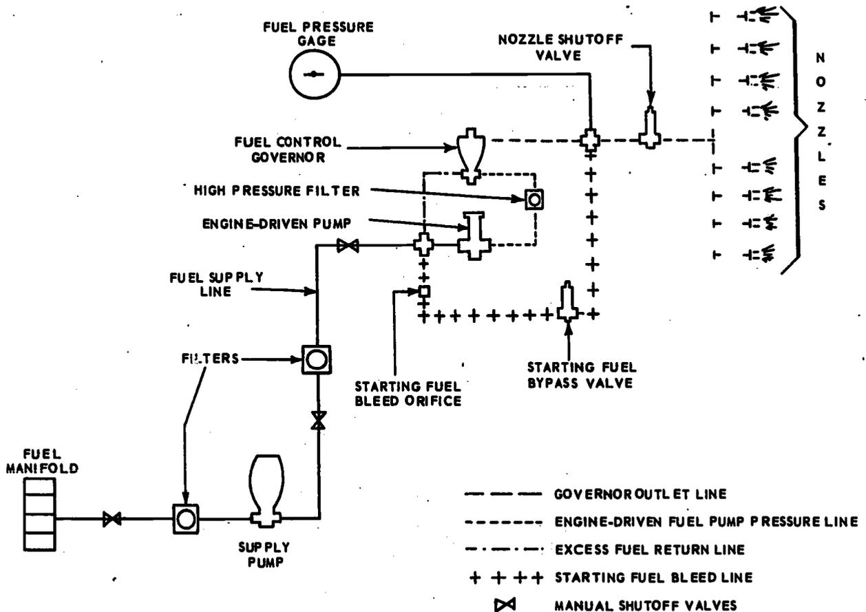
Figure 23-15.— Fuel flow diagram for gas turbine engine.
