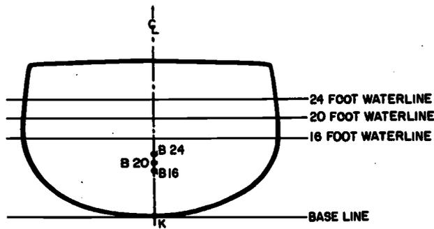
Figure 3-5.—Successive centers of buoyancy (B) for different drafts. 8.50
