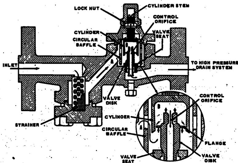
Figure 14-7.—Impulse steam trap.
