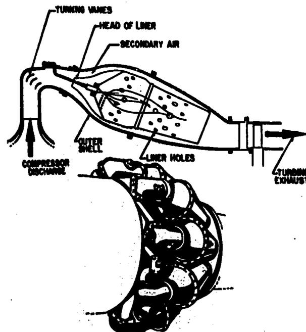
Figure 23-7.—Tubular or can-type combustion chamber.
