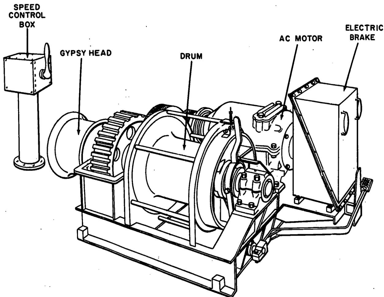
Figure 21-8.—A-C electric motor drive winch.
