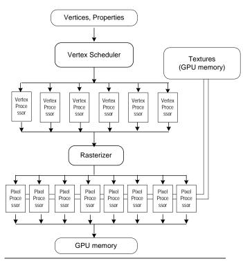
Figure 1. Simplified block diagram for a GPU
