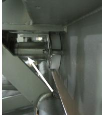
The drive motor is separated from the blender wall to prevent oil or grease from entering the blender.
