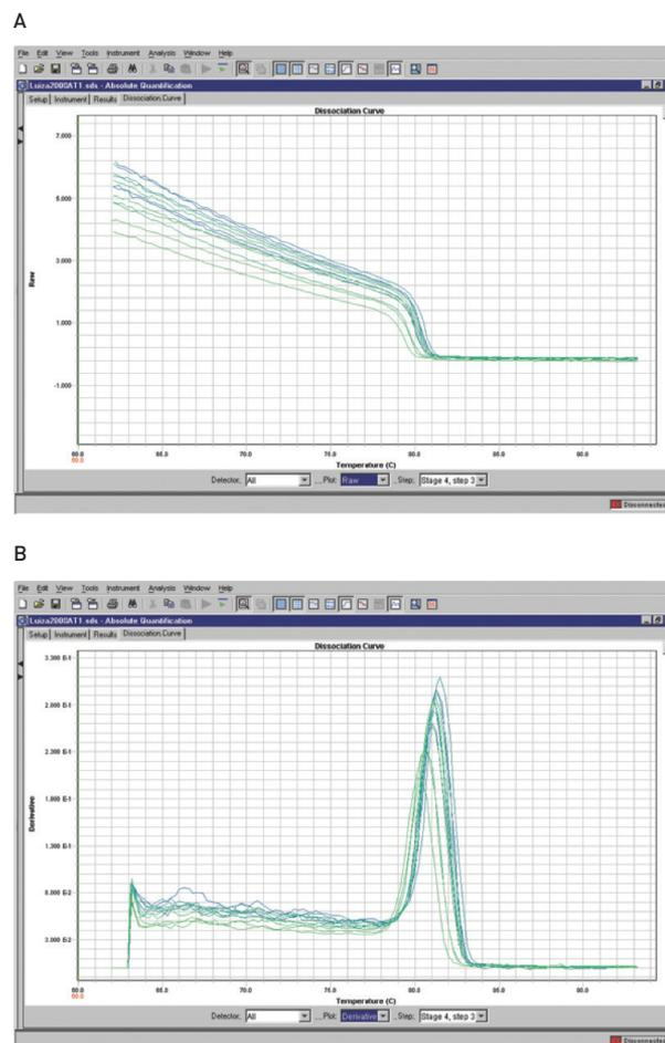
Figure 5. Melting curve (A) and  $-\Delta F/\Delta T$  vs. temperature (B).
