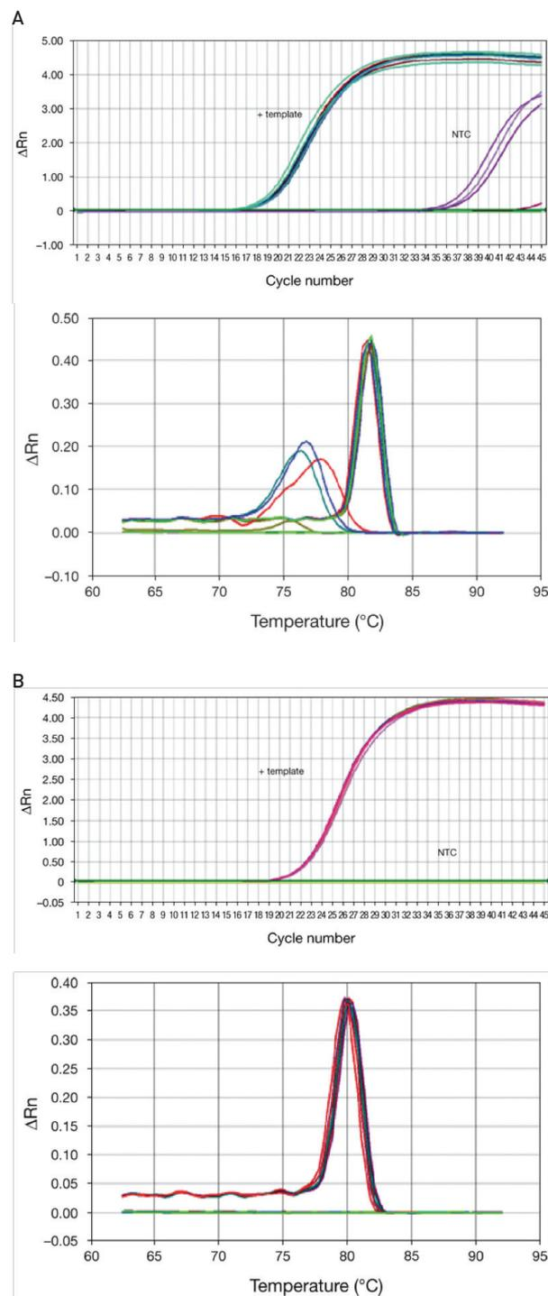
Figure 31. Amplification plots showing effects of poorly stored primers (shown by the melt curve and background fluorescence) (A) vs. properly stored primers (B).
