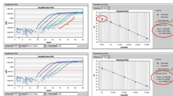
**Figure 36.** Improvement of standard curve slope achieved by excluding outlier data. Amplification was performed on a dilution series over 5 orders of magnitude. Across this range, the slope is only -2.9, which is outside the desired efficiency window. The curves represented by the lower panels have had the highest dilutions omitted from the standard curve, and the efficiency reanalyzed. The slope has improved to -3.1, which is considered efficient enough to validate the assay.
