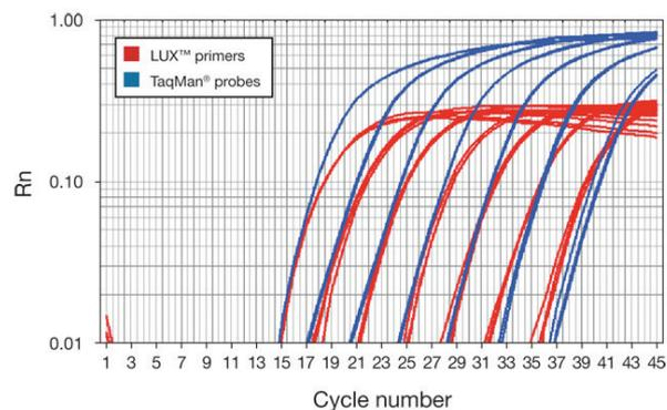
**Figure 35.** Log plot screen shot showing an example of two sets of curves with differing plateau heights and therefore different exponential phases. The most accurate portion of an amplification curve for C<sub>t</sub> determination is directly in the middle of the exponential phase when viewing the log plot. The ideal threshold setting is sometimes unique for each set of data.
