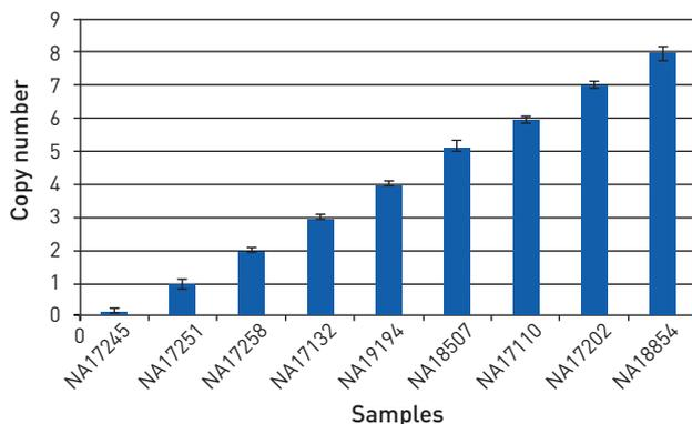
**Figure 43. Precision demonstrated for copy number analysis of the *CCL3L1* genetic locus on chromosome 17. (A)** Copy number was measured across 9 DNA samples. The CV (column 6) was below 2.6% for each set of replicates, demonstrating a high degree of measurement reproducibility within each replicate group. **(B)** As demonstrated by non-overlapping error bars, the achieved measurement precision enables statistical discernment of the *CCL3L1* copy number in samples containing 7 and 8 copies.
