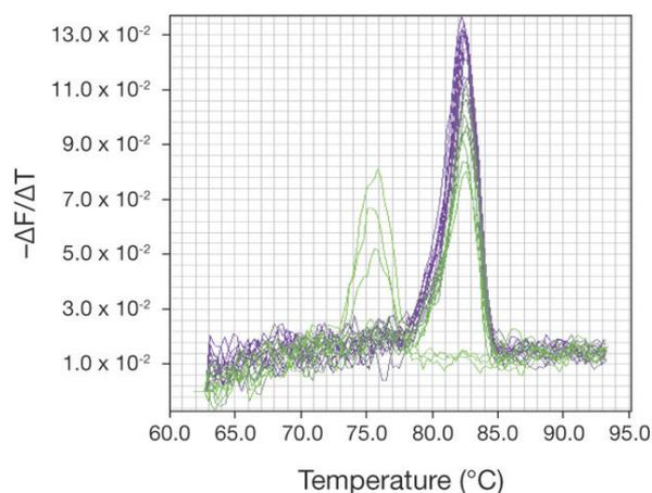
Figure 12. Melting curve analysis can detect the presence of nonspecific products, such as primer-dimers, as shown by the additional peaks to the left of the peak for the amplified product peaks.
