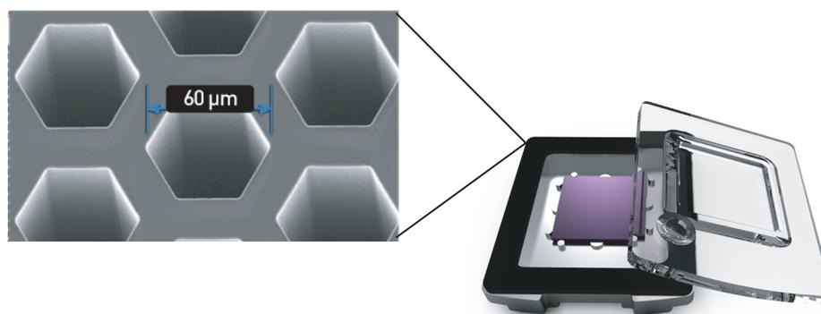
**Figure 38. QuantStudio® 3D Digital PCR 20K Chip.** Each chip is designed with 48 subarrays x 64 through-holes/subarray. Hydrophilic and hydrophobic coatings on plates enable reagents to stay in the bottomless through-holes via capillary action.
