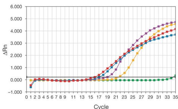
**Figure 32. Template dilution series to assess reaction efficiency.** Dilutions with earlier  $C_t$  values exhibit compressed  $C_t$  values and abnormal curve shapes. As the template becomes more dilute, inhibition vanishes and the curves take on the more characteristic exponential phase shape.
