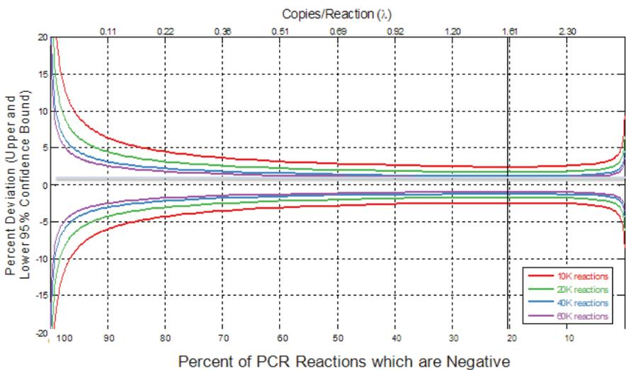
Figure 40. Poisson equation used to calculate target quantity from digital PCR data.
