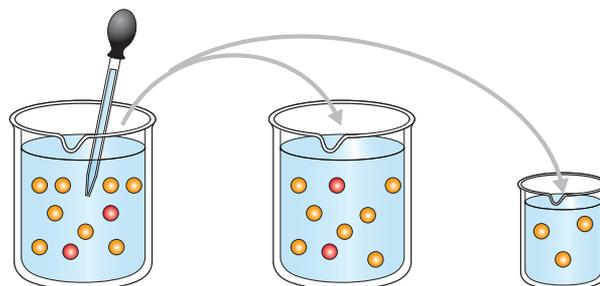
**Figure 41.** The Poisson principle assumes an appropriate volume of the total pool is sampled. Increasing the amount sampled from the total pool increases the ability to accurately determine the number of targets.
