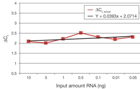
**Figure 26. Relative efficiency plot.** The  $\Delta C_t$  ranges from 2.0 to 2.5. When plotted against dilution or input amount of RNA, a slope is obtained. While a perfectly flat line (slope = 0) indicates identical efficiency across all input concentrations, a slope of  $<0.1$  is generally considered acceptable when employing the  $\Delta\Delta C_t$  method.
