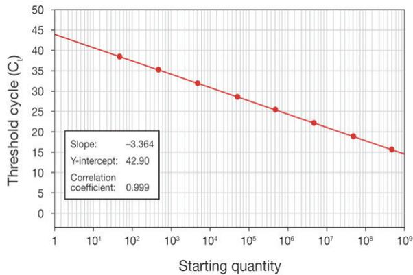
**Figure 4. Example of a standard curve of real-time PCR data.** A standard curve shows threshold cycle ( $C_t$ ) on the y-axis and the starting quantity of RNA or DNA target on the x-axis. Slope, y-intercept, and correlation coefficient values are used to provide information about the performance of the reaction.
