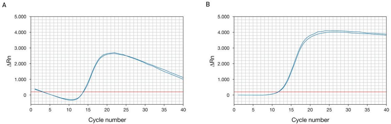
Figure 33. Amplification plots showing an incorrectly set baseline (A) and a correctly set baseline (B).
