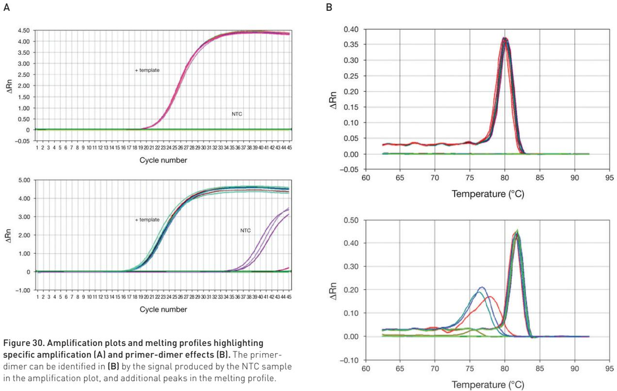
**Figure 30. Amplification plots and melting profiles highlighting specific amplification (A) and primer-dimer effects (B).** The primer-dimer can be identified in (B) by the signal produced by the NTC sample in the amplification plot, and additional peaks in the melting profile.
